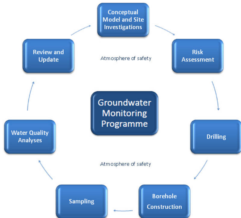
Figure 1 Groundwater monitoring programme stages
