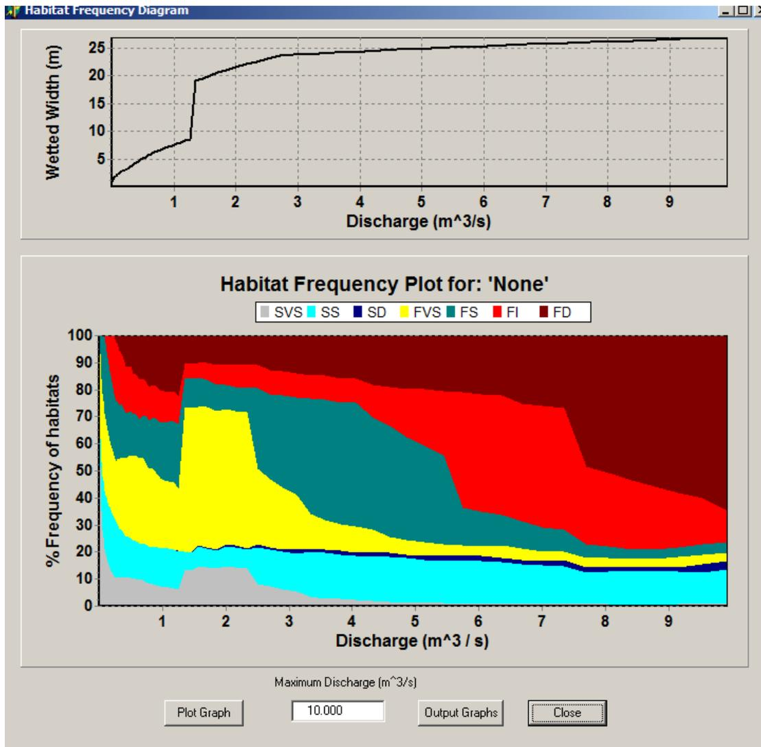
Figure 3.13 Habitat frequency plot generated for EWR site 6 by RDRM model
