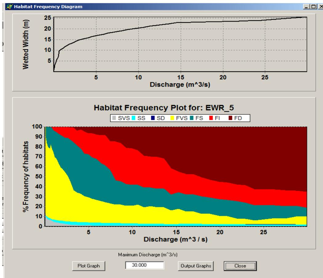
Figure 3.29 Habitat frequency plot generated for EWR site 5 by RDRM model
