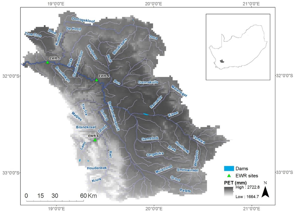
Figure 2.3 Potential evapotranspiration (PET) data for Doring catchment derived from the South African Atlas of Climatology and Agrohydrology (Schulze 2007)
