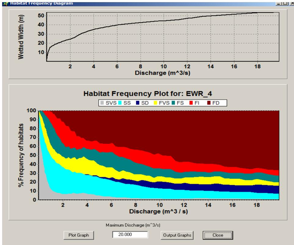
Figure 3.21 Habitat frequency plot generated for EWR site 4 by RDRM model
