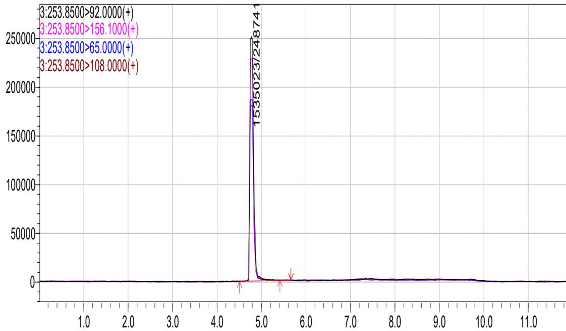
Figure 6: Chromatogram for Sulphamethoxazole
