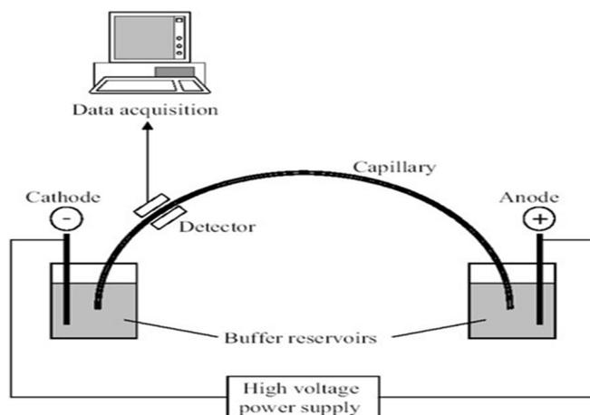
**Figure 2: Principle of Capillary Electrophoresis**
