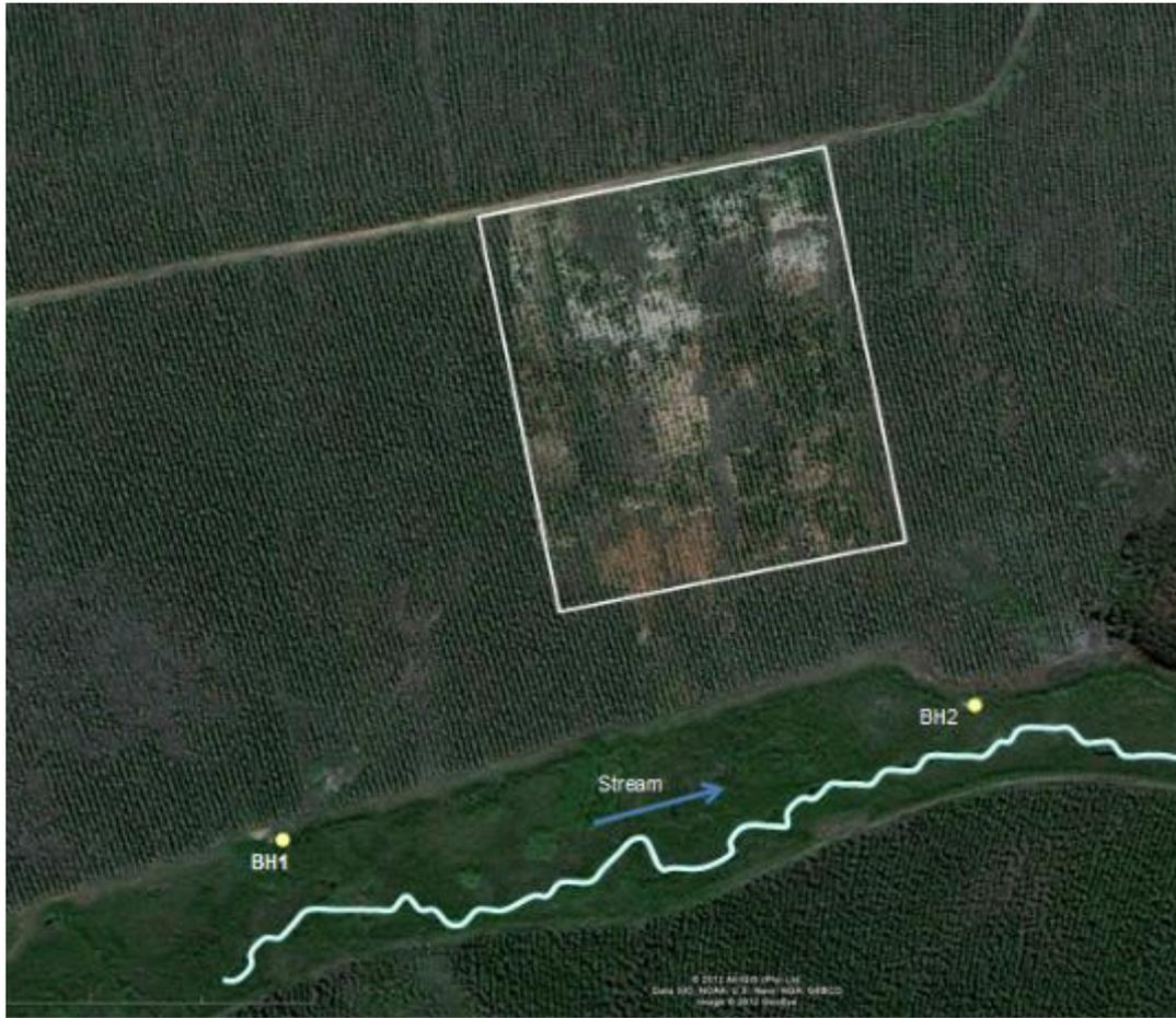
**Figure 5-4: Location of boreholes in relation to experimental site (outlined in white)**
