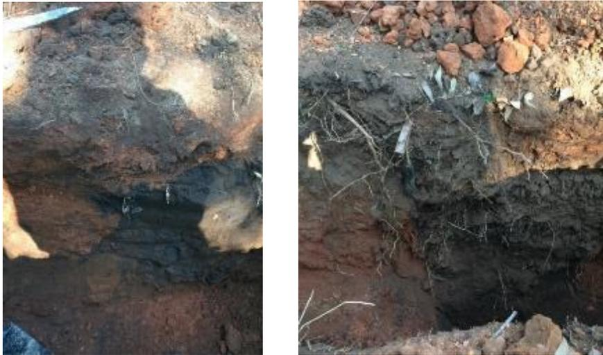
**Figure 6-9: Observed visual differences in surrounding soil and buried sludge trenches, demonstrating a continued difference after >10 years**
