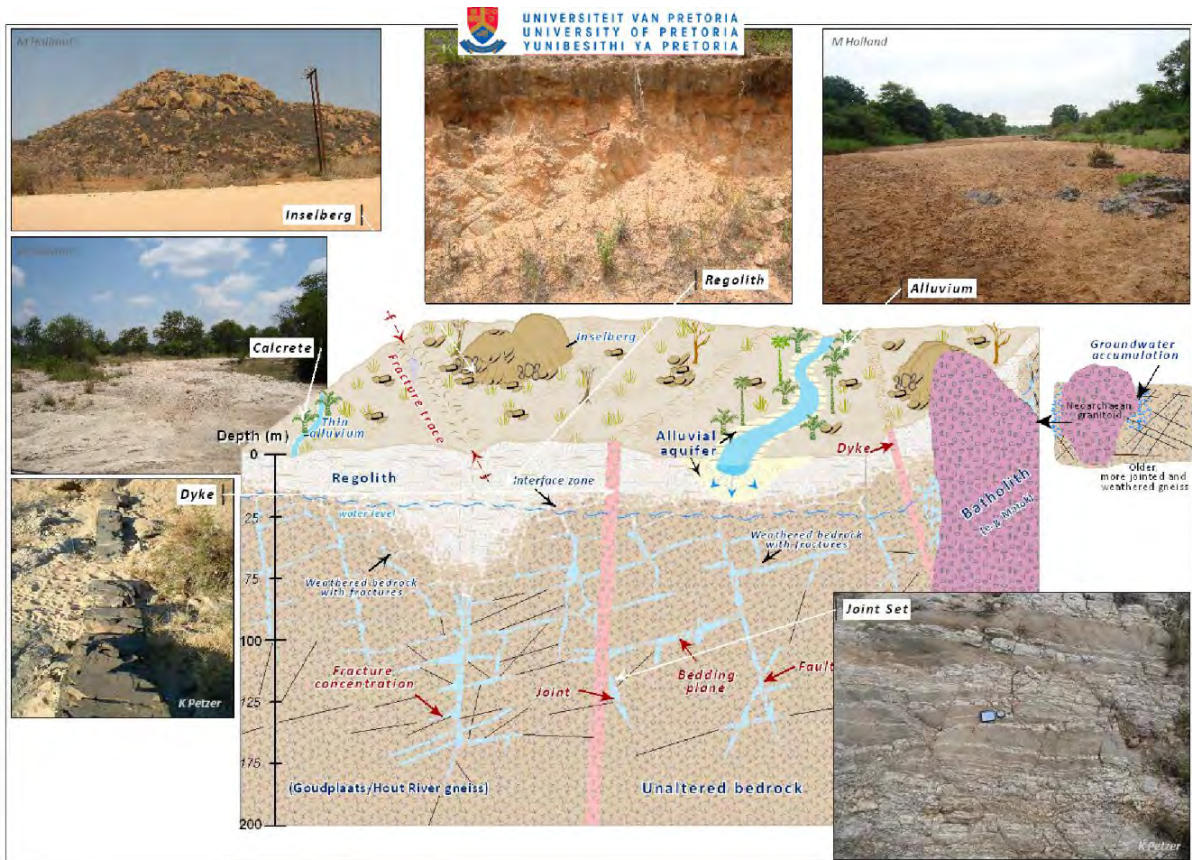
Figure 5.36: Conceptual models of vadose zone and aquifer layers in the region from Walker et al., 2018 (middle) and Holland 2011 (bottom) highlighting the weathered and fractured layer aquifers and riparian alluvial aquifer
