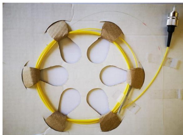
Figure 3-7: Optic fibre displaying the connector, a splice, and a bare FBG between the red markers
