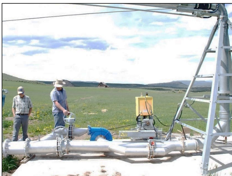
Figure 2-20: Small hydropower connected to centre pivot (Agri-Pulse, 2017)
