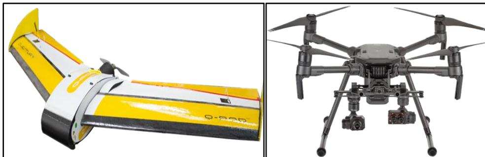
Figure 2-2: Examples of (a) fixed-wing UAVs and rotary (b) winged UAVs. Fixed-wing UAVs have wider coverage, which could be 10 times bigger than rotary winged, but image quality is poor due to flying speed, and cannot stay stationary in flight mode.
