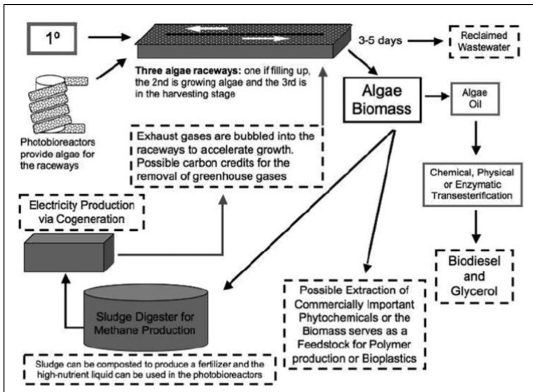
Figure 39: Flow diagram of an algae-based wastewater treatment system<sup>6</sup>
