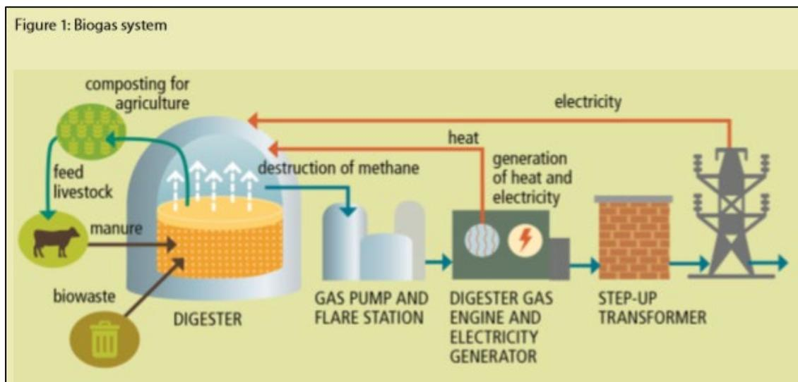
**Figure 36: Typical Biogas to Energy diagram**
