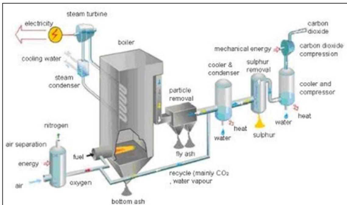
**Figure 37: Typical Combustion Waste to Energy Process**
