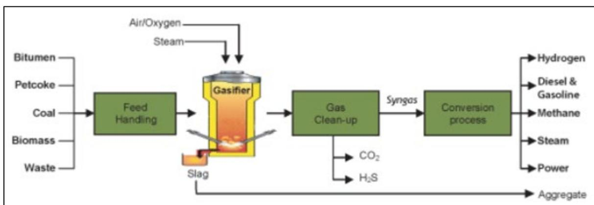
Figure 40: Typical Gasification Diagram
