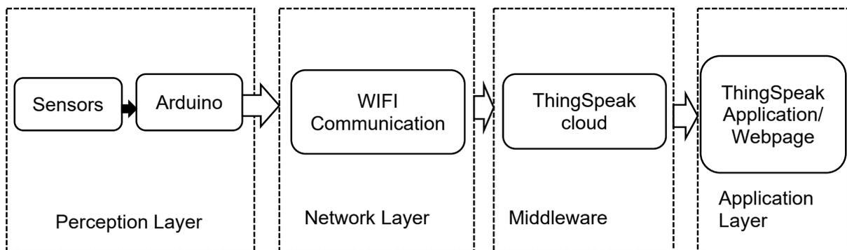
Figure 5.3: The IoT architecture layer for the groundwater quality system
