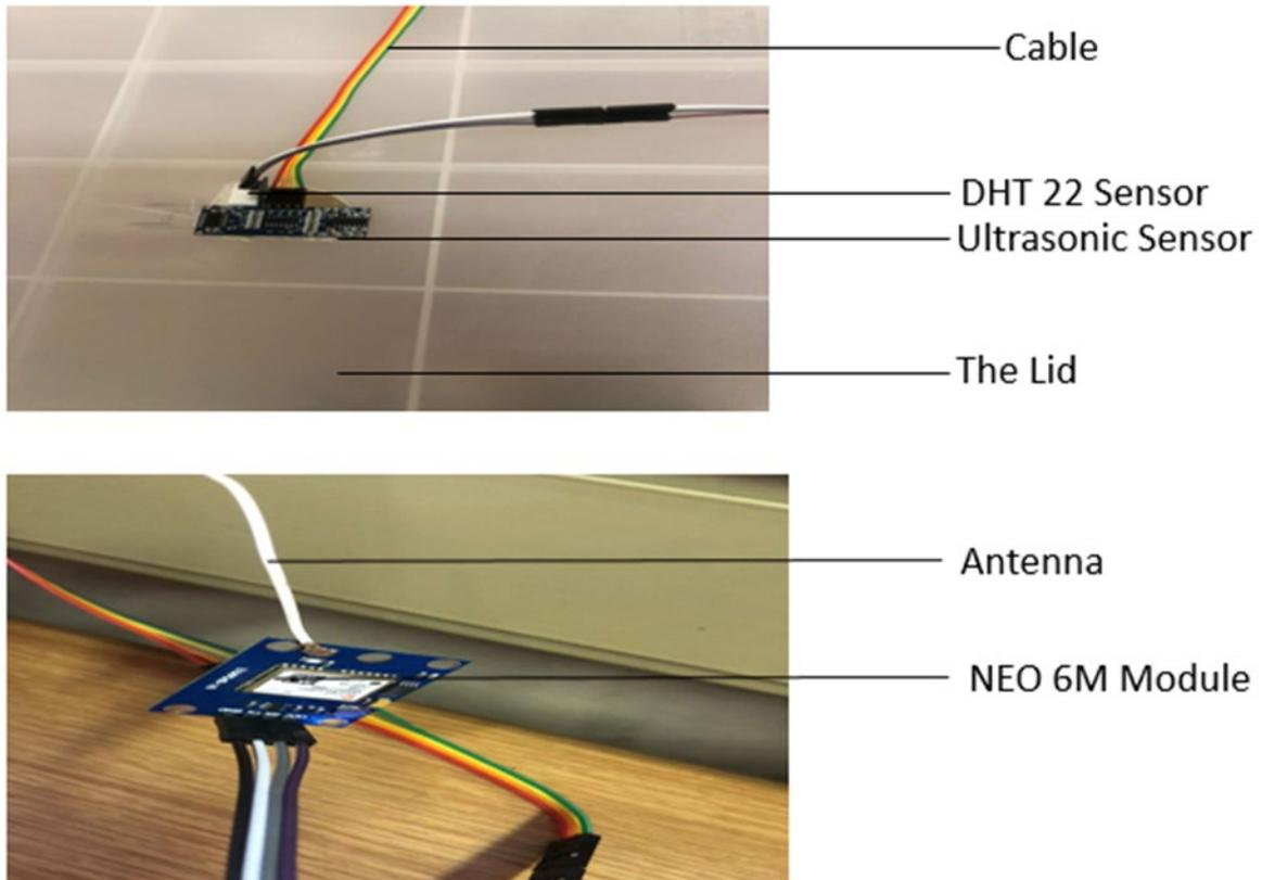
Figure 7.2: Data acquisition unit for groundwater-level monitoring subsystem
