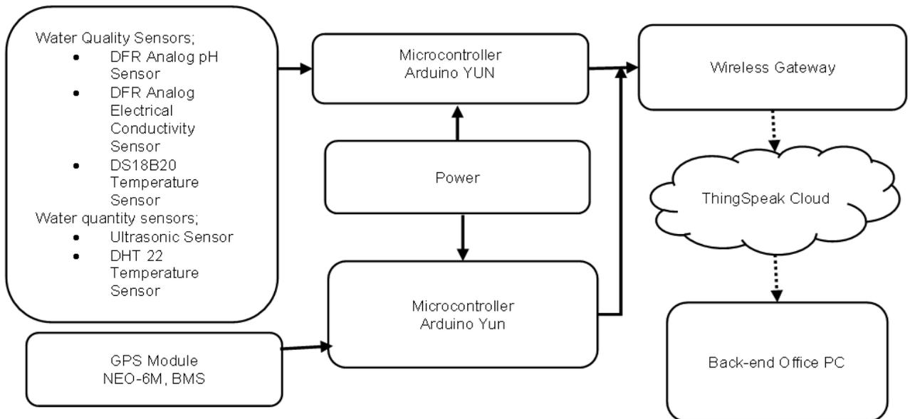
*Figure 6.1: Block diagram of the integrated groundwater monitoring system*
