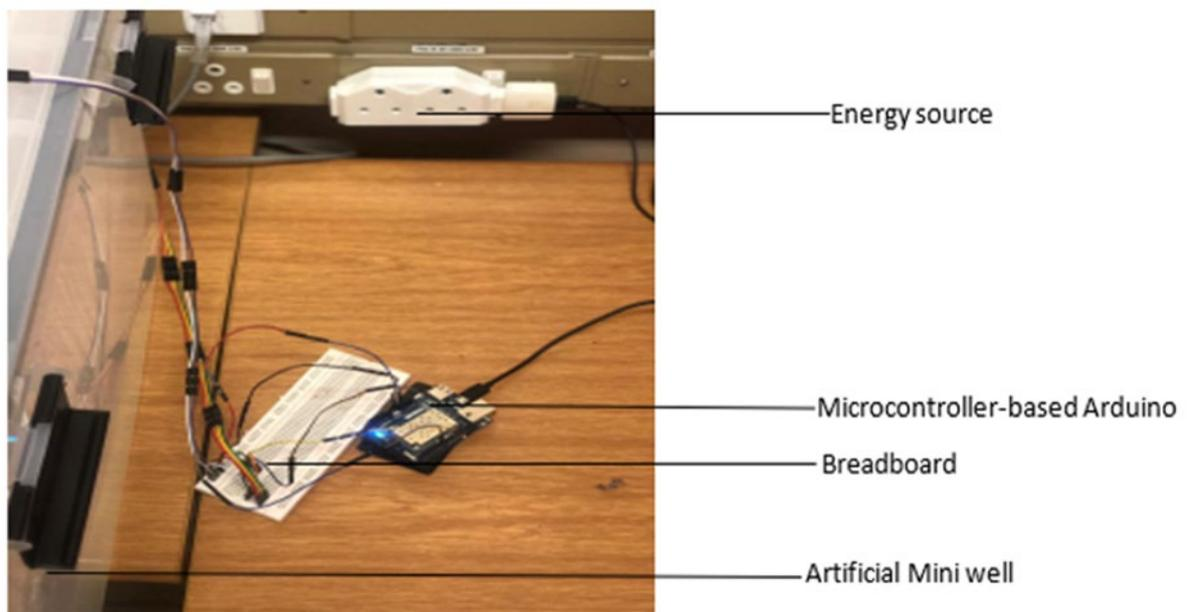
*Figure 7.4: Data capturing and processing unit for groundwater-level monitoring subsystem*
