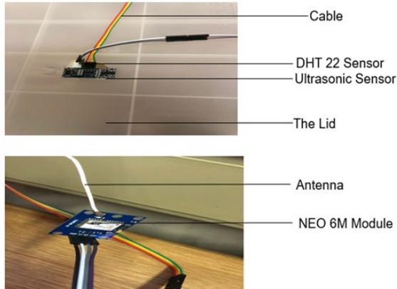
**Figure 6.2a: Level data acquisition unit**
