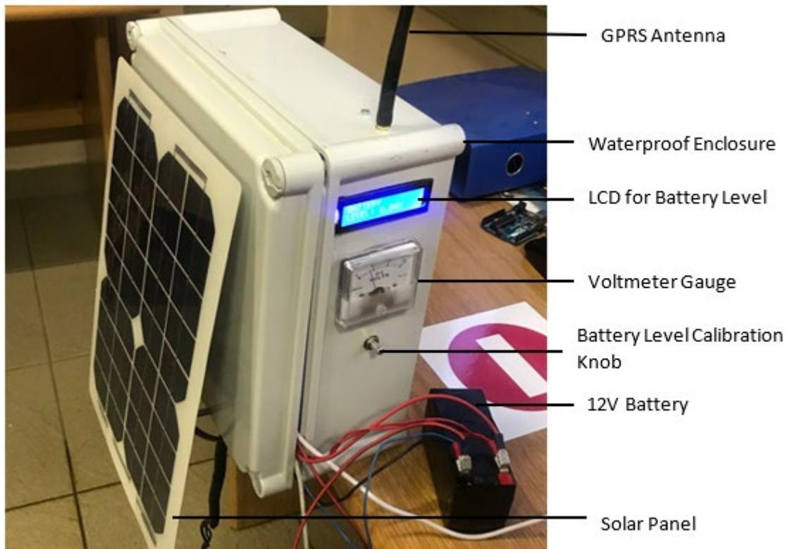
*Figure 6.6: The integrated prototype*
