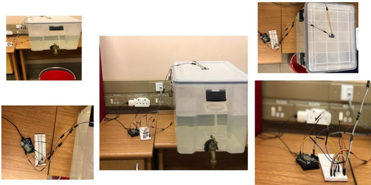
Figure 7.6: The complete groundwater-level monitoring subsystem
