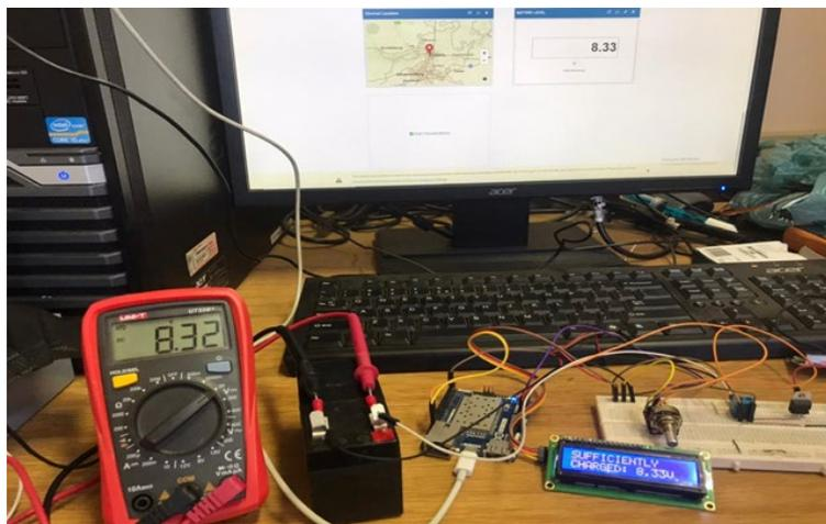
Figure 7.13: Battery-level monitoring testing
