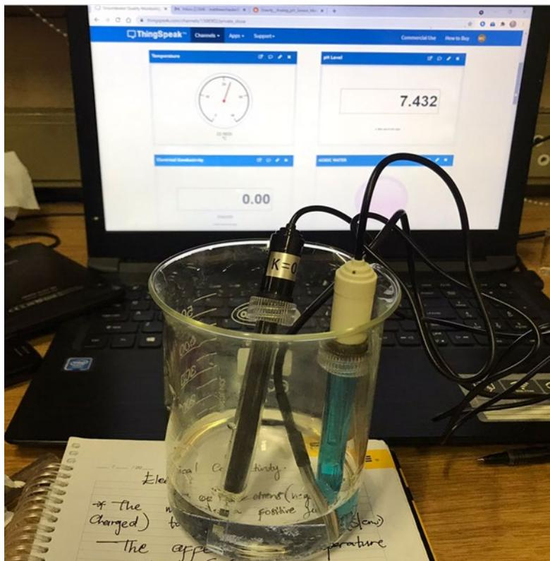
Figure 7.10: The result of the water quality sensors' calibration set-up
