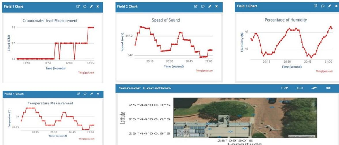
Figure 4.9: Graphical display unit/storage unit on the ThingSpeak IoT platform
