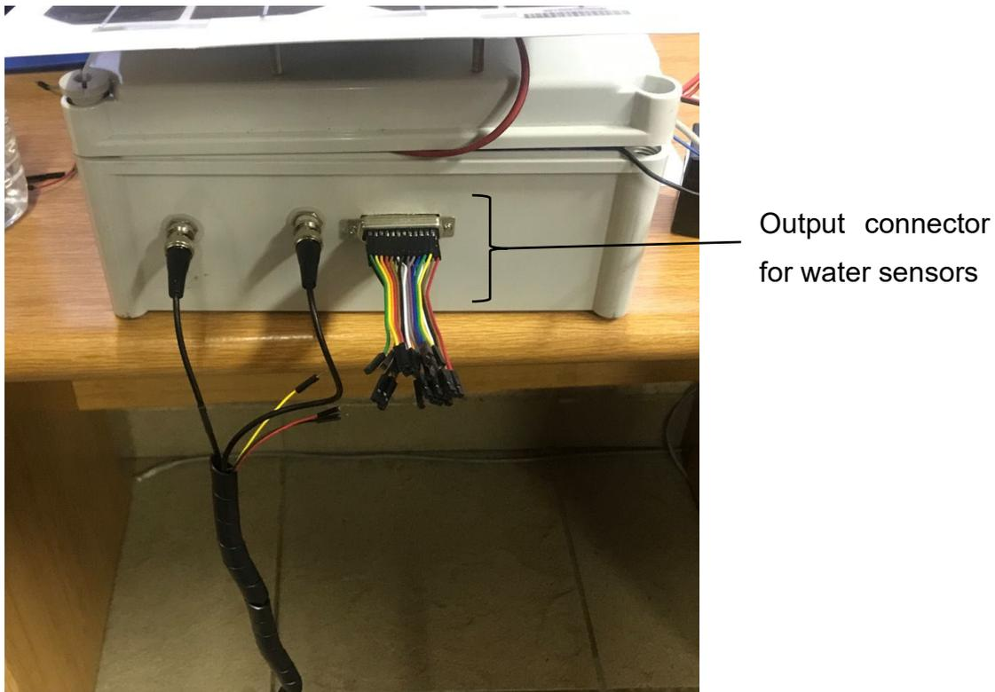
*Figure 6.7: The rear side of the integrated prototype*
