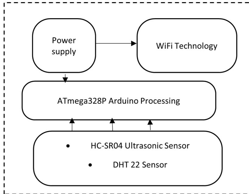
Figure 4.6: Schematic diagram of data capturing layer
