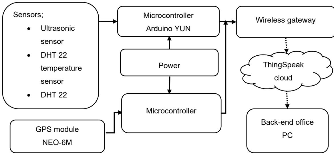
Figure 4.1: Block diagram of groundwater level monitoring system
