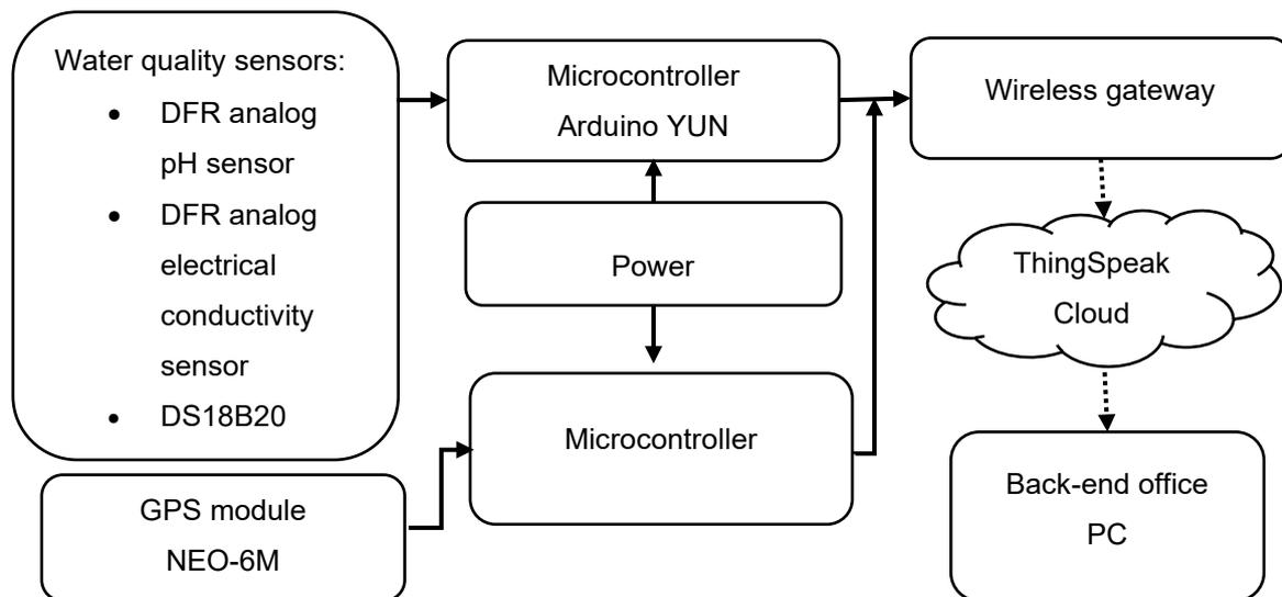
*Figure 5.1: Block diagram of groundwater quality monitoring system*
