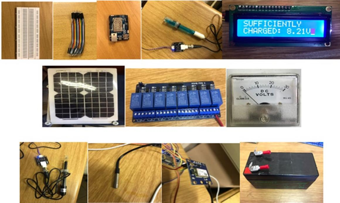
*Figure 7.7: Components used for groundwater quality subsystem development*
