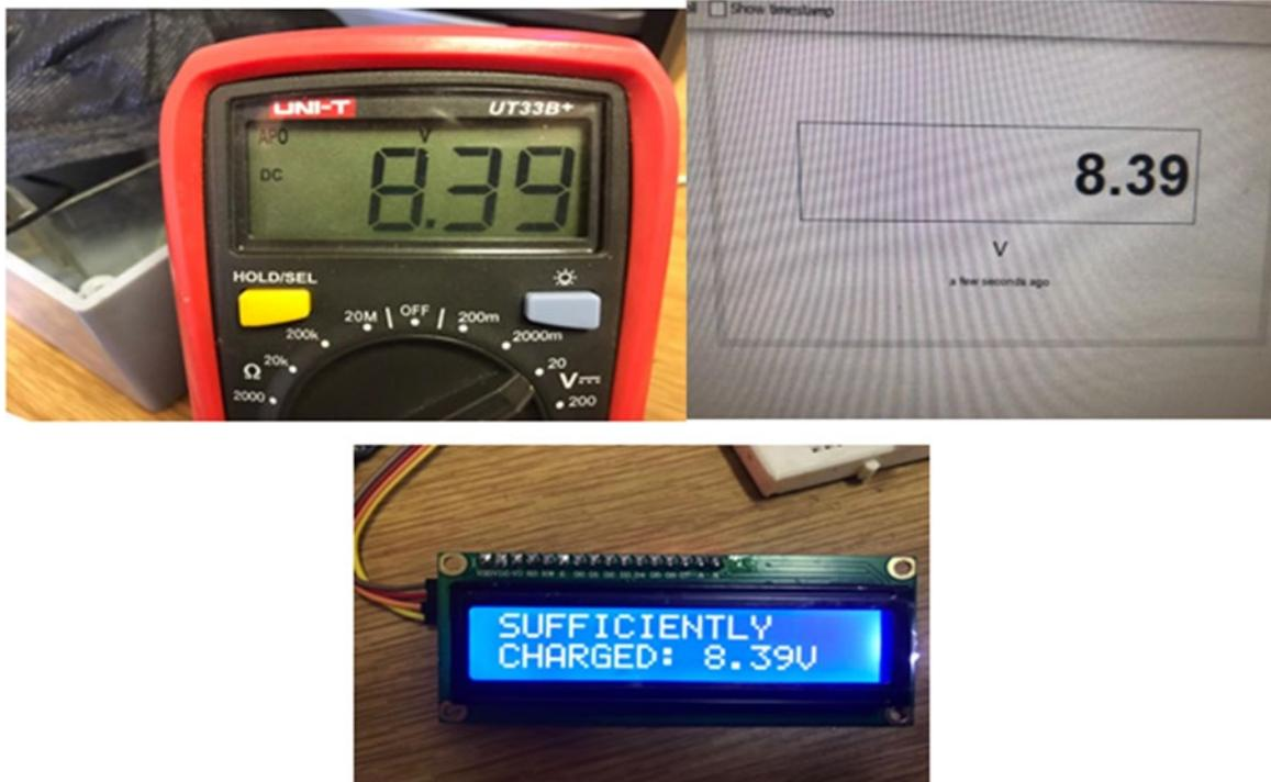
Figure 7.18: Battery level results
