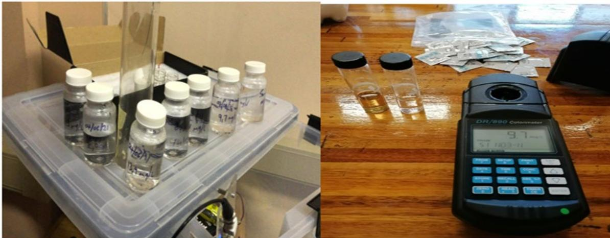
Figure 7.15: Nitrate concentration samples and HACH DR/890 colourimeter showing colour change, i.e. presence of nitrates
