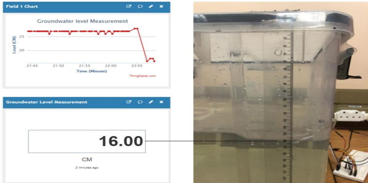
Figure 4.13: Set-up 1 results
