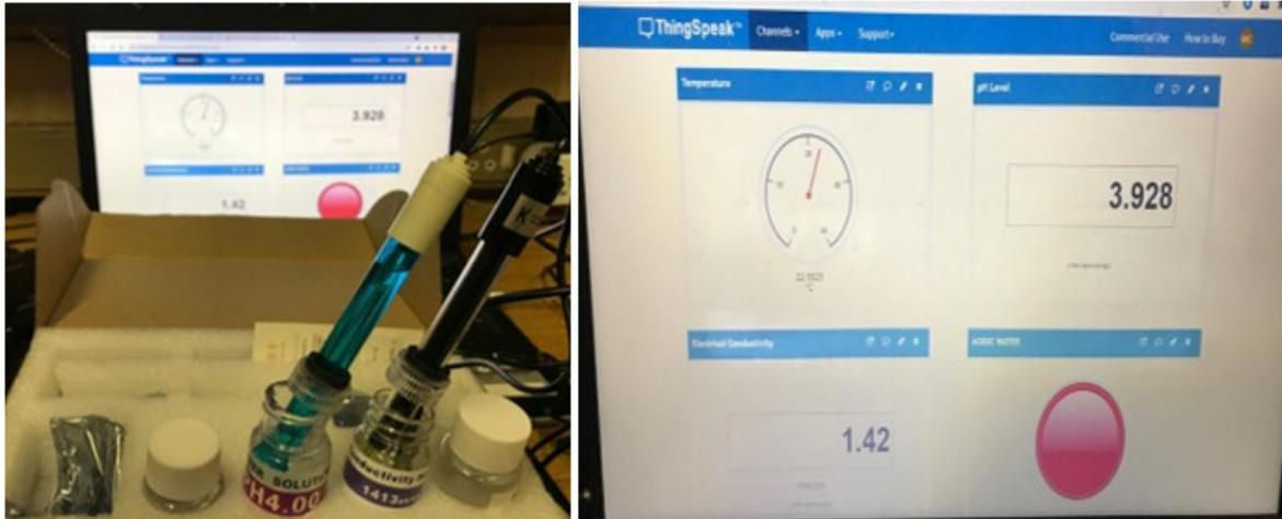
Figure 7.11: Water quality sensors' calibration (pH = 4.00 and electrical conductivity = 1413uS/cm)
