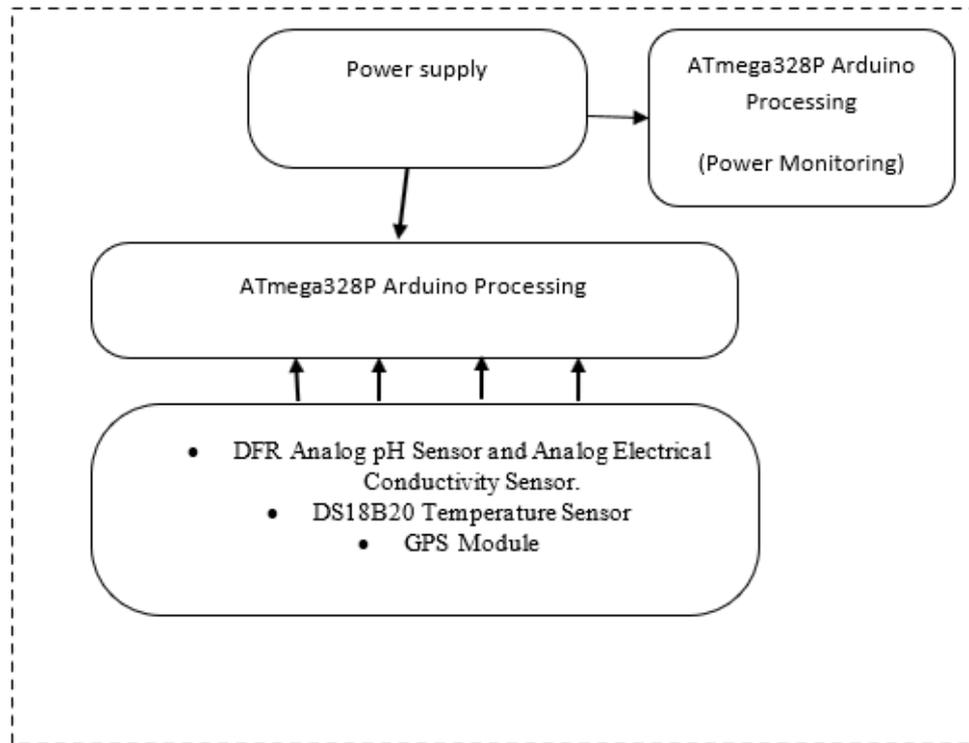
Figure 5.4: Schematic diagram of data-capturing layer
