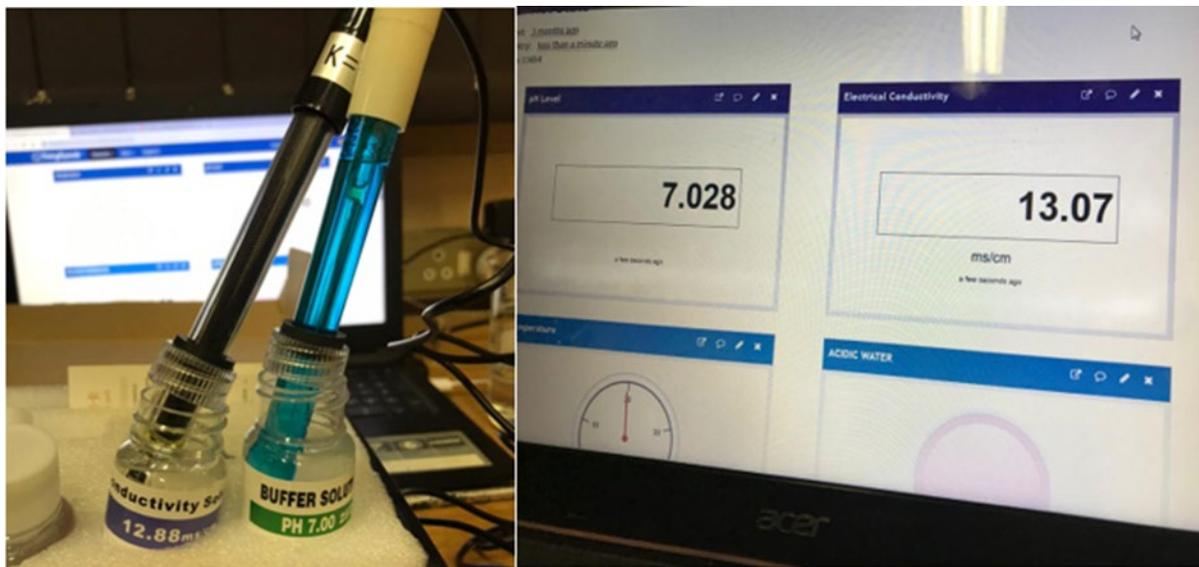
Figure 7.12: Buffer solutions; (pH = 7.00 and electrical conductivity = 12.88 mS/cm)
