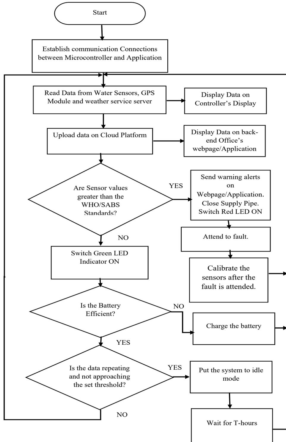
Figure 5.2: Groundwater quality monitoring flow chart
