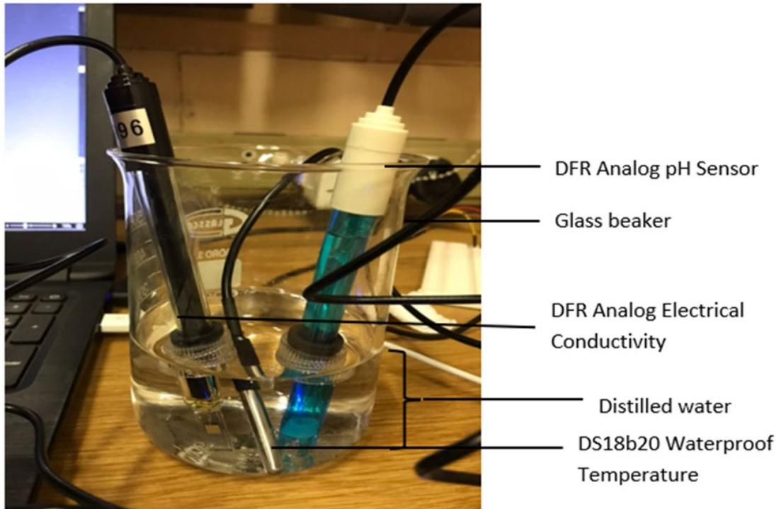
Figure 7.9: Water quality sensors' calibration set-up
