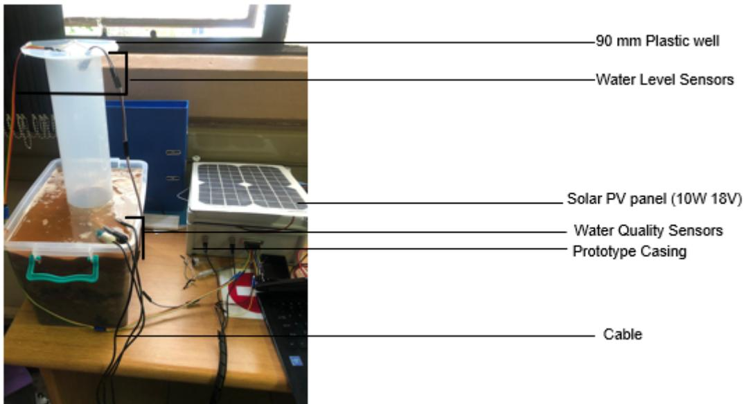
Figure 6.8: The integrated groundwater monitoring system during testing
