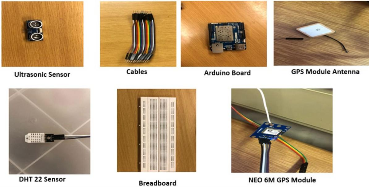
Figure 7.1: Components used for groundwater-level monitoring subsystem development
