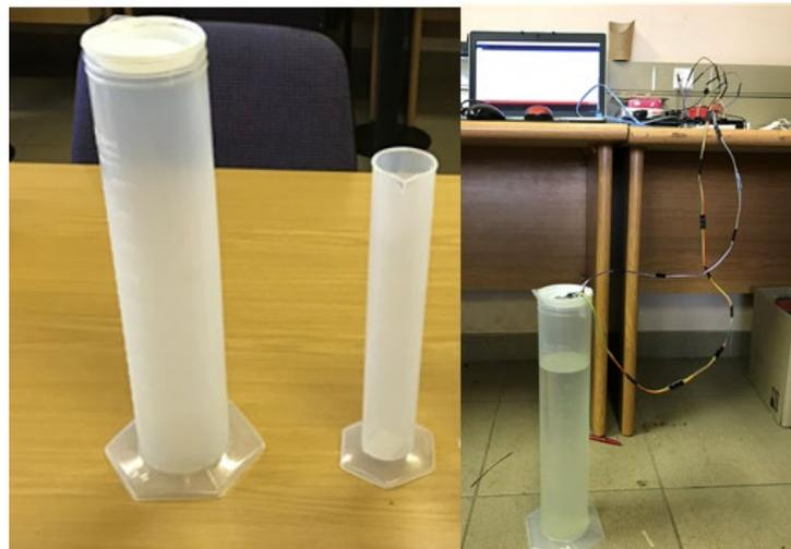
*Figure 4.10: A 50 mm and 90 mm diameter well*
