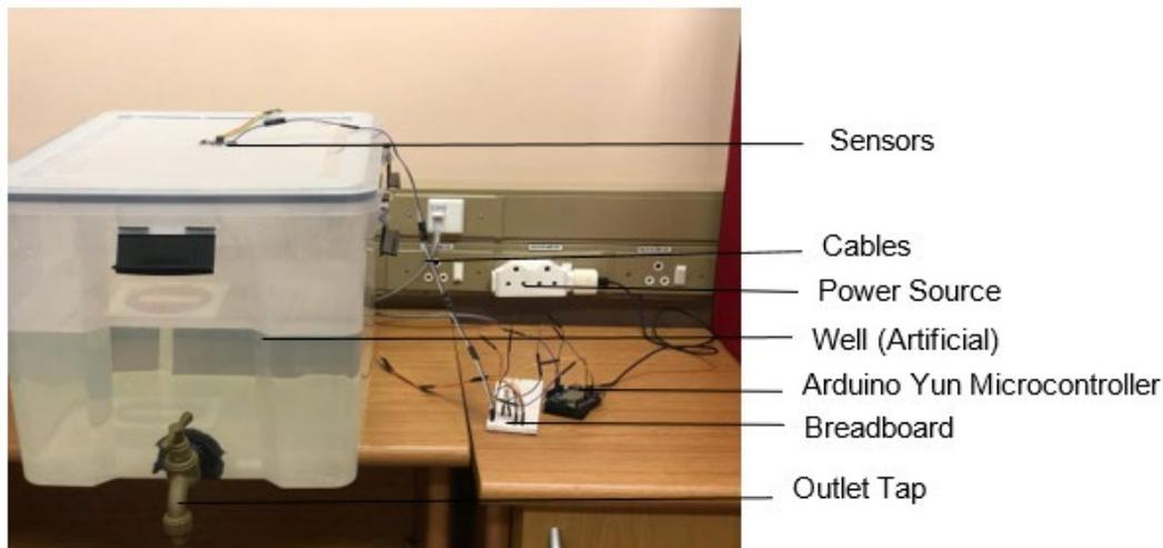
*Figure 4.8: Overall integrated groundwater monitoring subsystem laboratory set-up*
