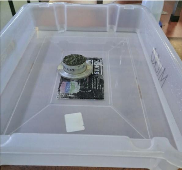
**Figure 6.6. Faecal sludge in a core undergoing saturation in water via a saturated ceramic filter (the container lid is absent for more clarity)**
