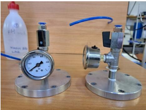
**Figure 6.3. Pressure gauges fixed on pressure cell lids**
