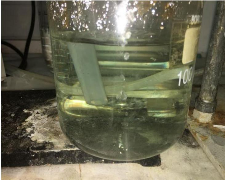
Figure 4-13 Ferrous iron rich leachate solution generated from pH-controlled column and used for crystallization studies.
