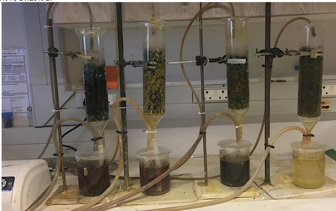
Figure 4-12 Leachate solutions generated after 530 days of experiments. From left to right: CW30%-B; CW20%-A; CW30%-A; CW20%-B.
