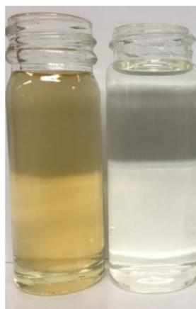
Figure 6-3 Colour removal from synthetic wastewater after solid-liquid separation
