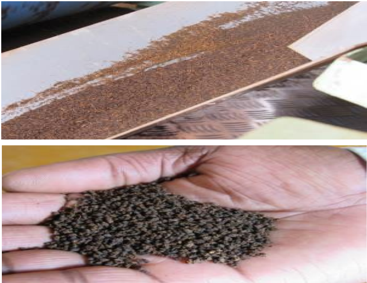
Figure 4.9: Tea in the process of fermentation, and a sample of dried black tea produced at Mukumbani Tea Factory
