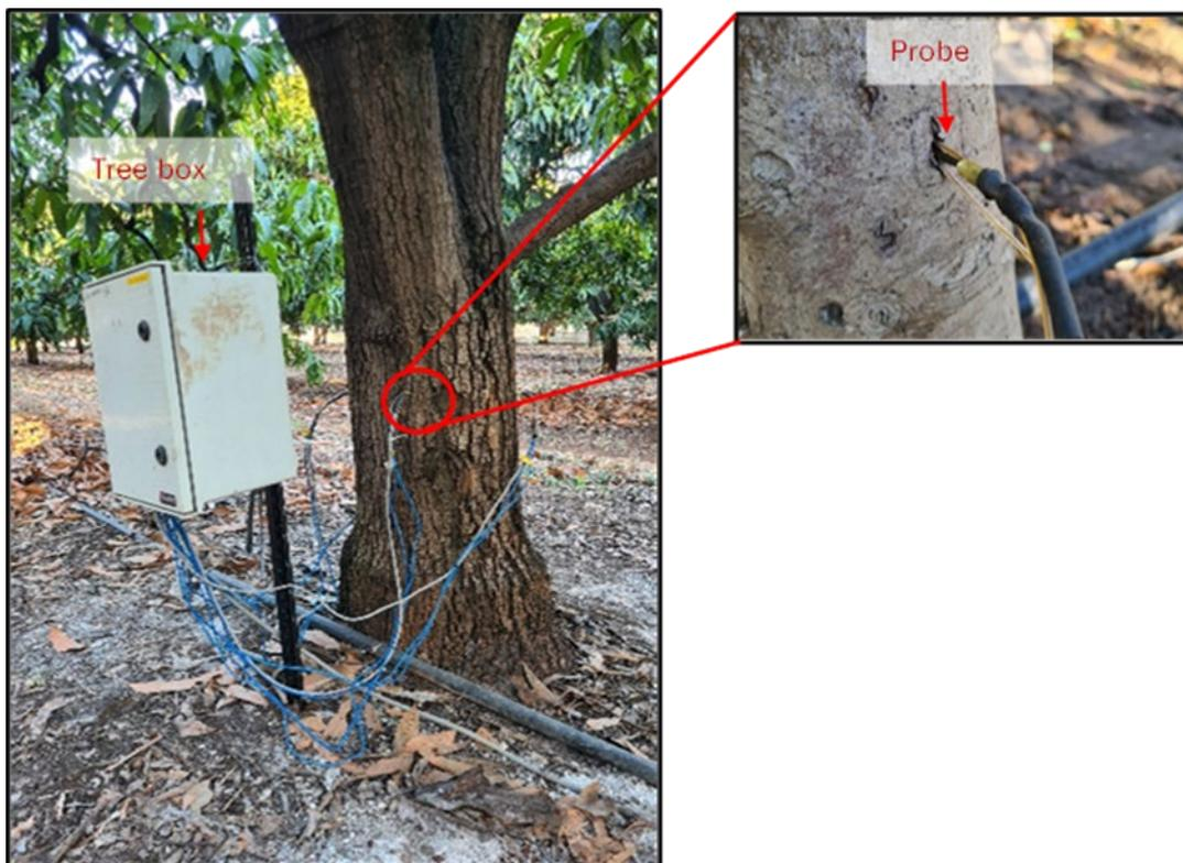
Figure 3.9: Tree box with four HRM probes. The insert shows an HRM probe, with two thermocouples installed at the top and bottom and a heater installed in the middle.
