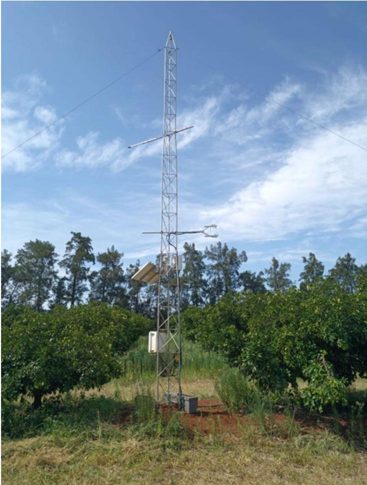
Figure 5.3: Eddy covariance system measuring evapotranspiration in the grapefruit orchard.
