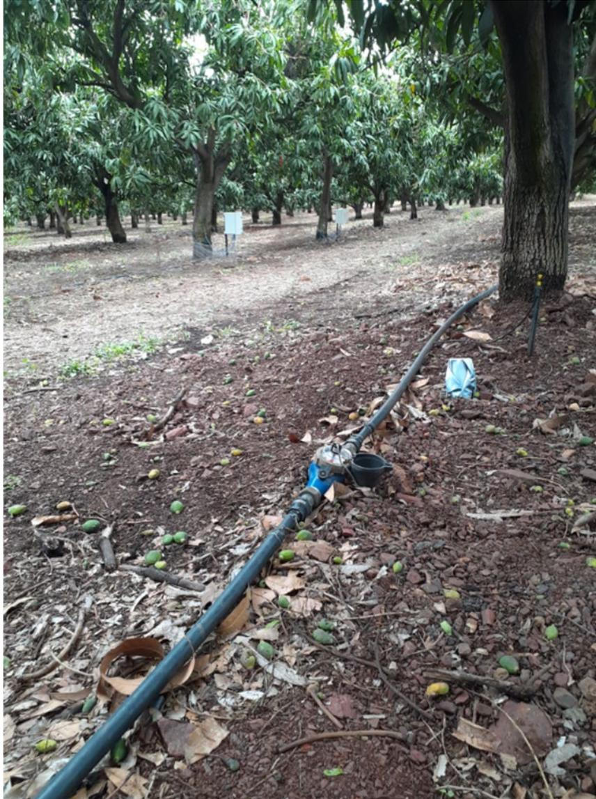
Figure 3.5: Water flow meter monitoring the irrigation volumes in the mango orchard.
