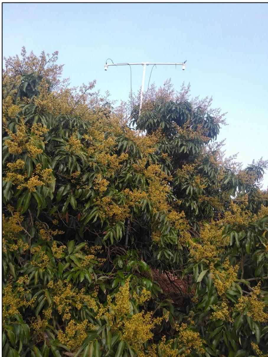
Figure 4.4: Setup of the infrared (IR) thermometer used to continuously measure canopy temperature of litchi trees.
