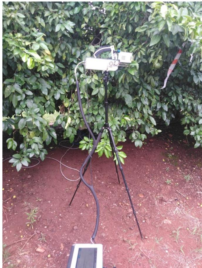
Figure 5.4: Measuring the leaf gas exchange with the Li 6800 in a mature grapefruit orchard.
