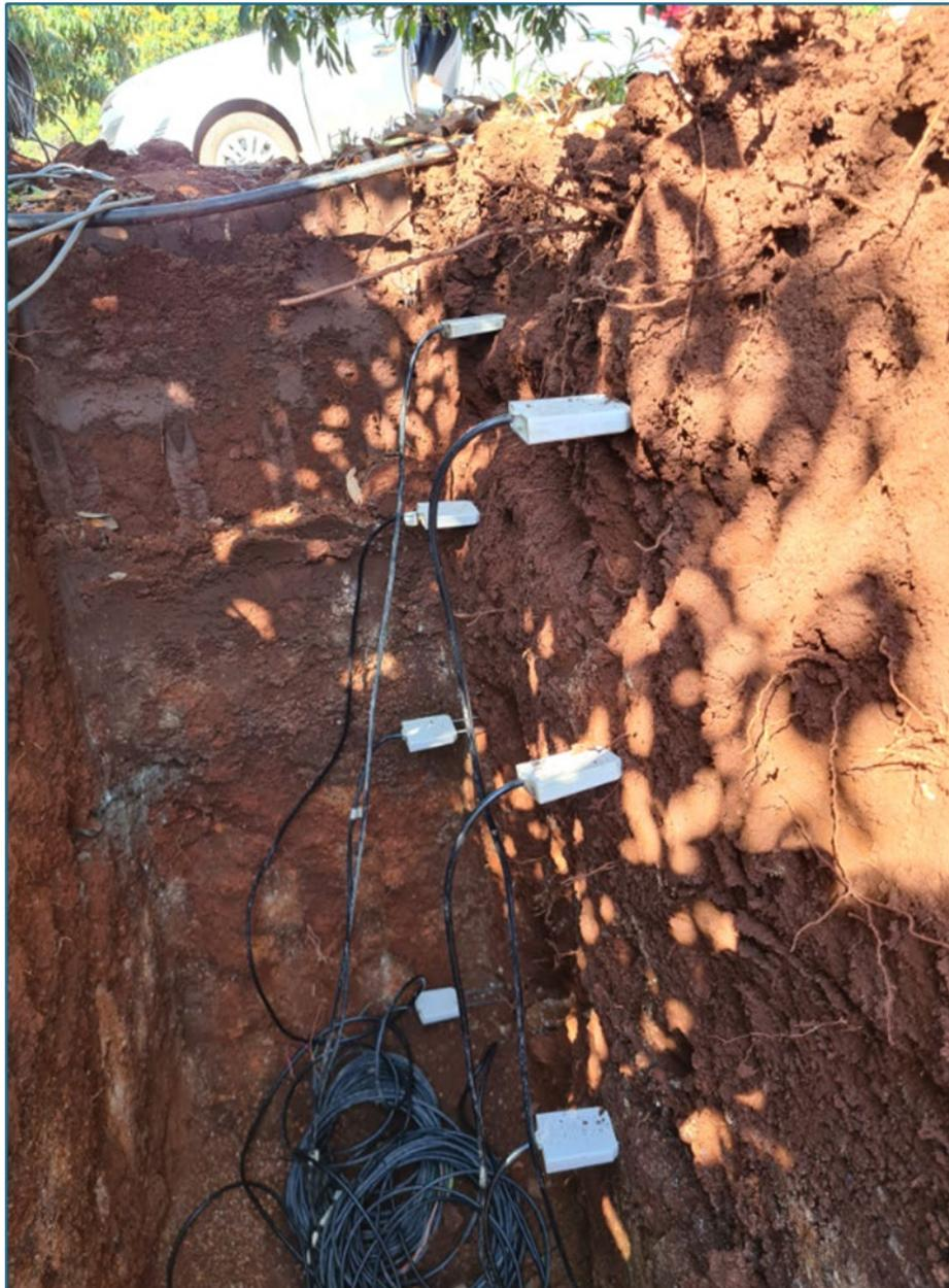
Figure 3.6: Placement of moisture probes to measure the volumetric soil water content in the mango orchard.
