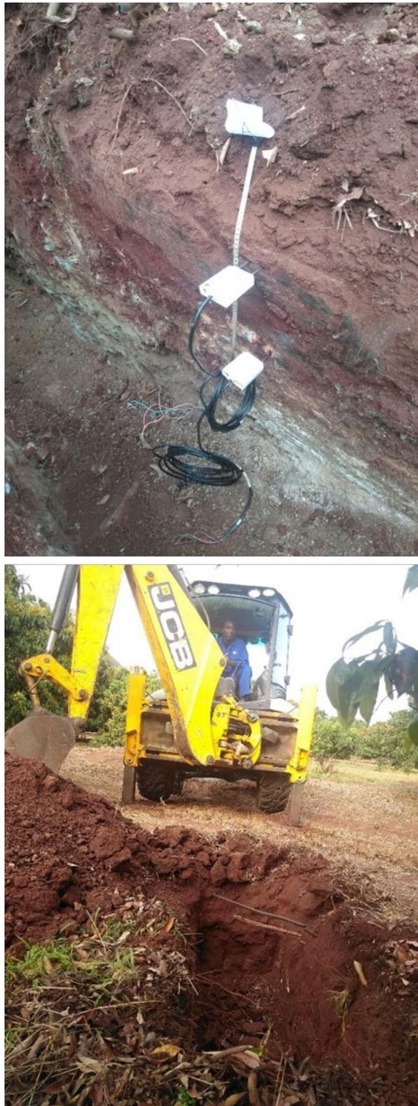
Figure 4.2: Soil Moisture probes installed at 30 cm, 60 cm and 120 cm horizontally below the ground in the profile pit.
