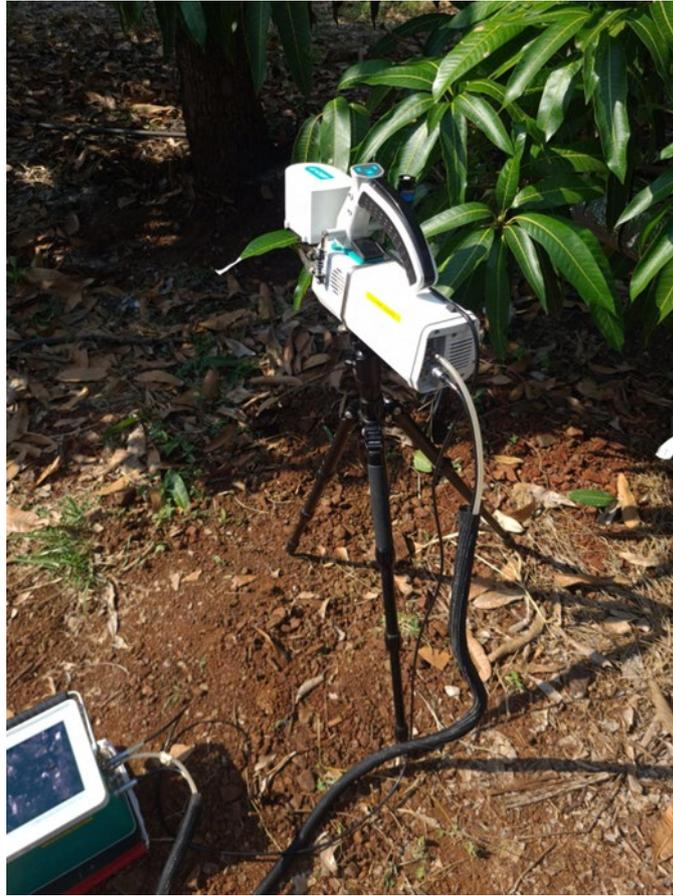
Figure 3.11: Infrared gas analyser measuring leaf photosynthesis, transpiration, and stomatal conductance of a mango tree in Malelane.
