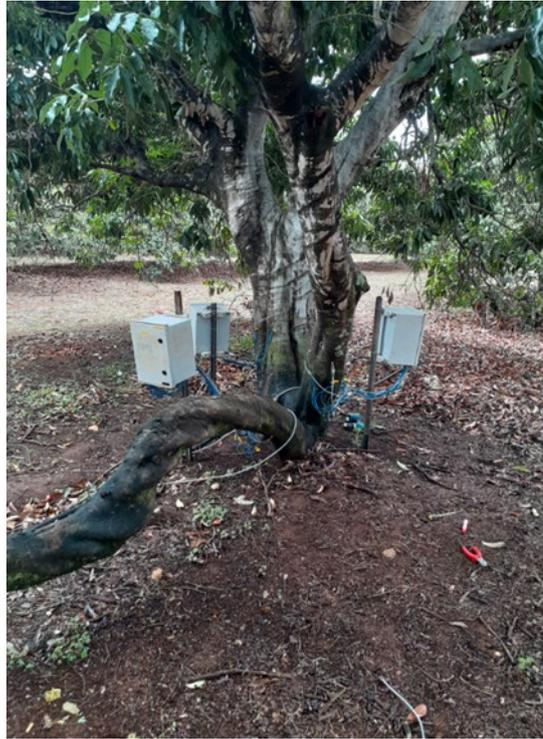
Figure 4.3: Heat Ratio Method setup on a litchi tree with multiple stems.
