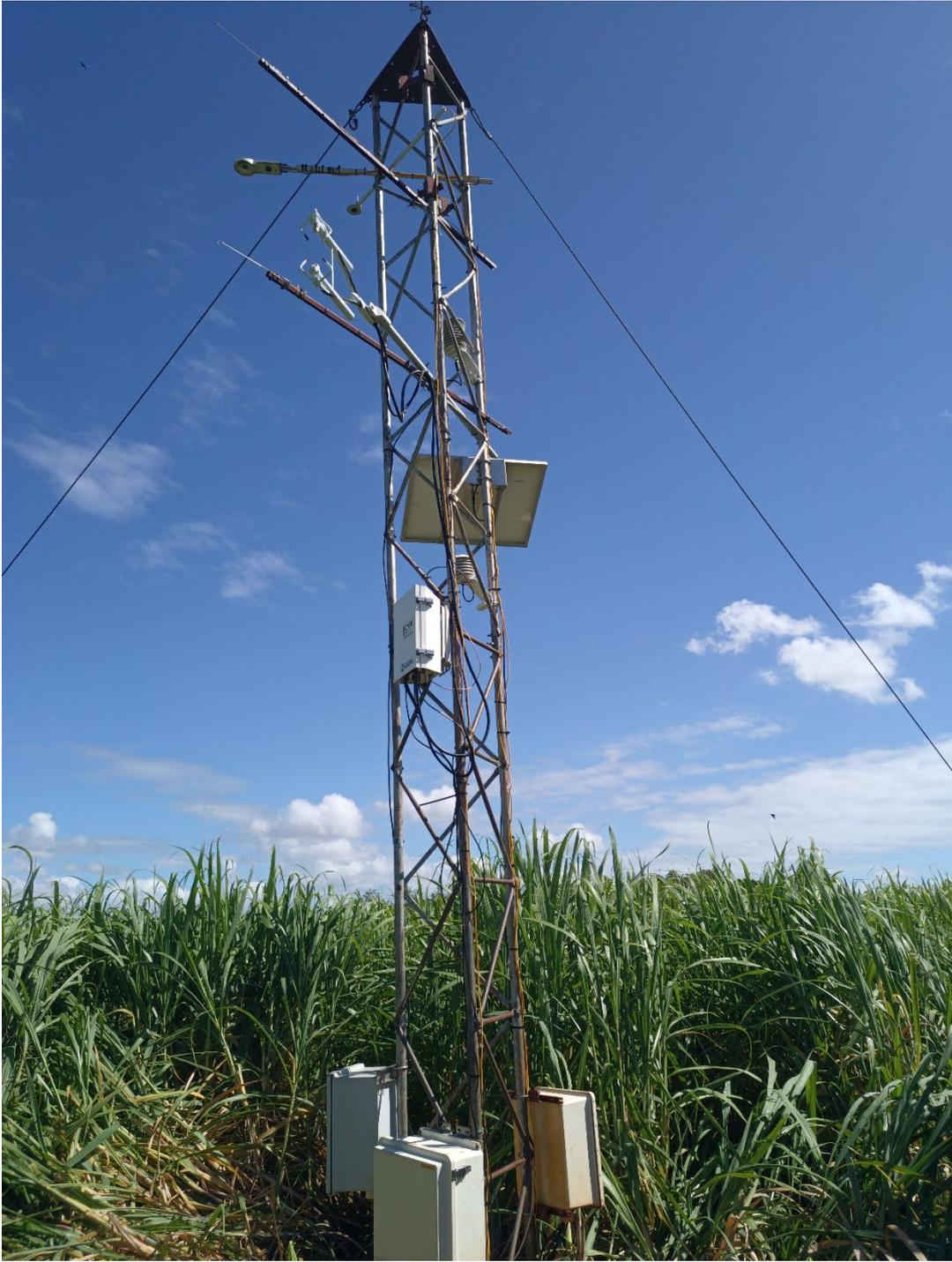
Figure 7.4: Calibration of the surface renewal method using the open path eddy covariance system.
