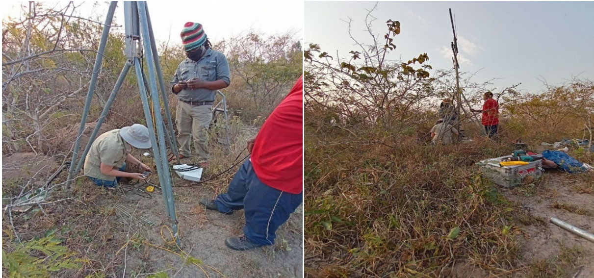
Figure 8-8: Installation of a Surface Renewal system in a bush encroached site in the Maputaland Coastal plain area
