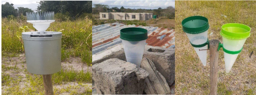
Figure 7-4 Rainfall samplers from left to right Palmex rain sampler RS1; rooftop rain gauge and rain gauge at 1.2 m
