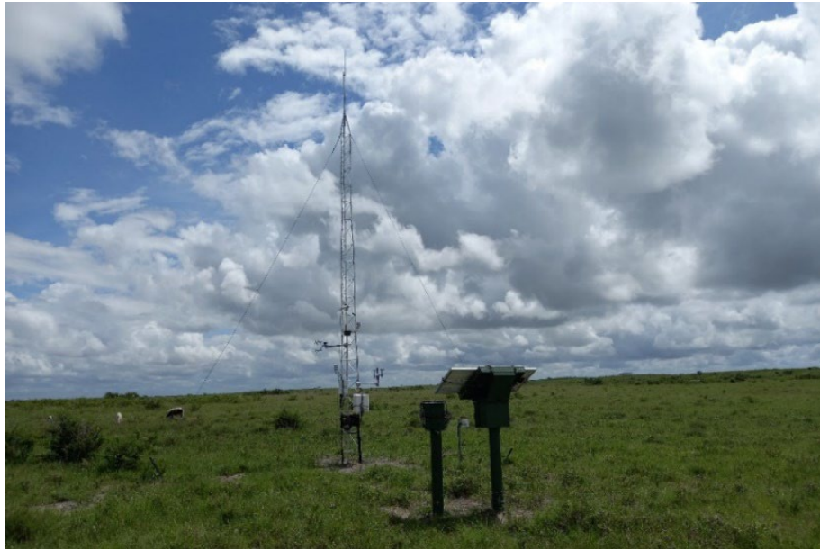
Figure 8-5 The grassland site where the Eddy Covariance system is installed
