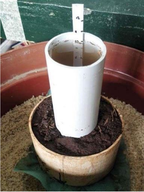
Figure 7.7: Measuring saturated hydraulic conductivity using the falling head method in the laboratory.
