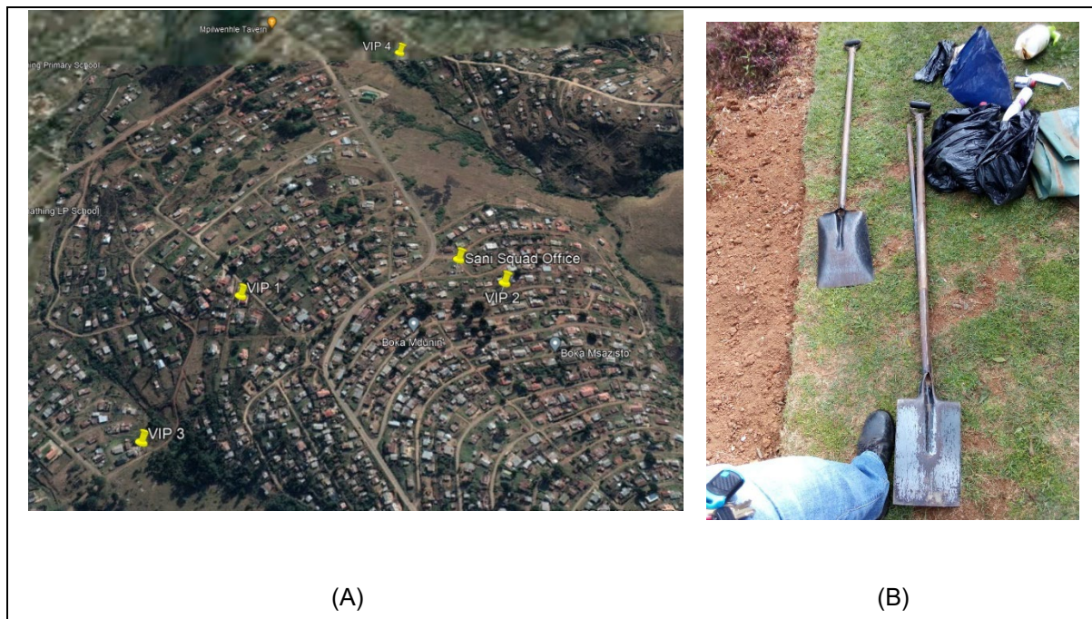
Figure 3-1: Sample collection (A) location of VIP latrines (Google Earth, 2022), and (B) Tools used to collect faecal sludge sample from the pit
