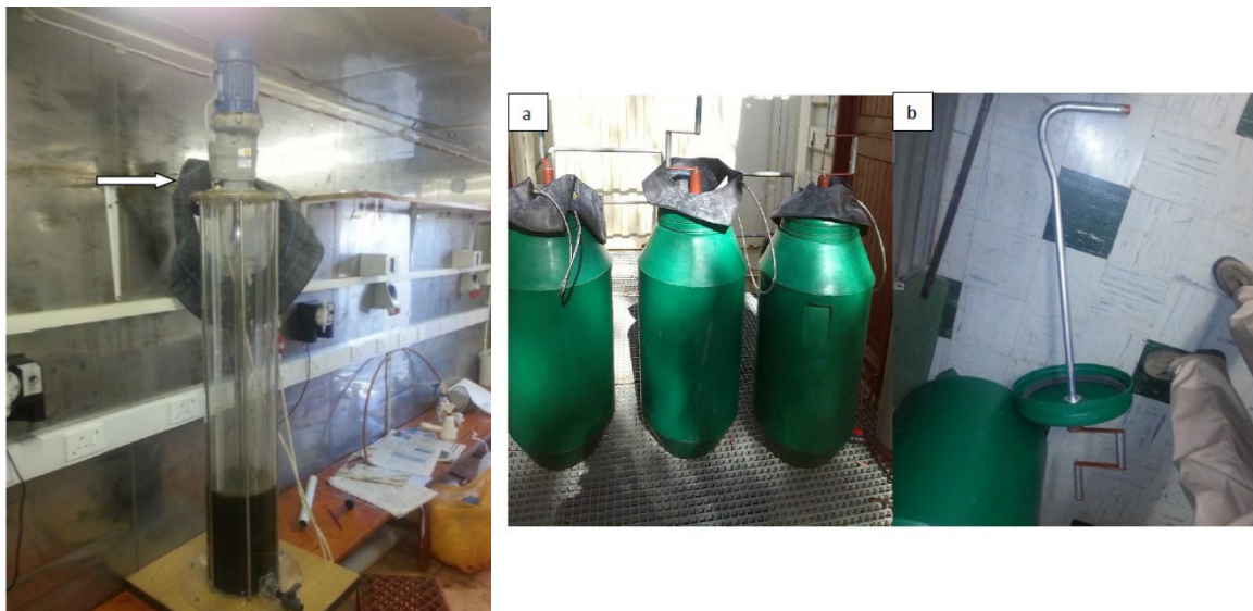
Figure 2-9: Left image, a perplex digester with a tube for gas collection (white arrow). Right image, 2 nd larger type of digester using 200 L containers, with attached car tyre tubes (a) and crank handle for mixing (b) (Madikizela et al., 2017)
