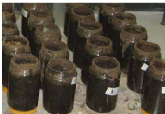
Figure 2-6: Laboratory trials of pit additive using honey jars under aerobic conditions (Foxon et al., 2009)
