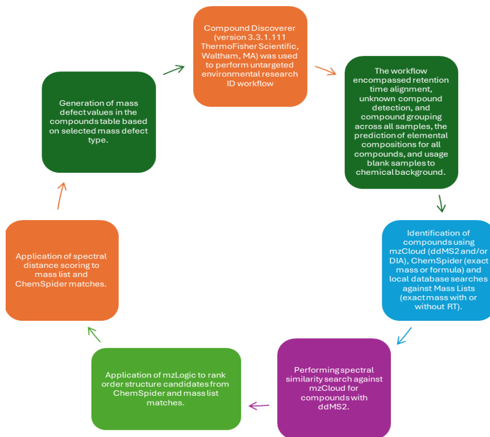
Figure 2-9: Non-targeted HRAM data Analysis Workflow using Compound Discoverer Software (Identification confidence taken from Schymanski et al., 2014. Environ. Sci. Technol., 48, 2097–2098.
