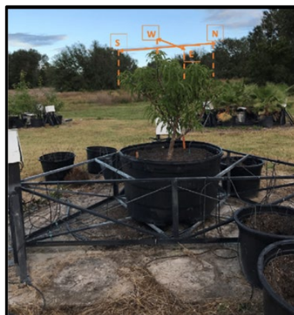
Figure 2.8: Lysimeter measuring evapotranspiration for a young peach tree (Photo taken from Zambrano-Vaca C).
