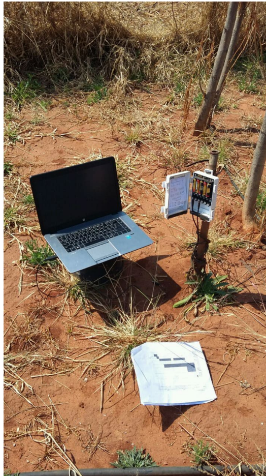
Figure 5.3: An EM50 datalogger connected to 10-HS capacitive soil water content sensors to record data automatically daily on a 2-year-old Moringa plantation at ARC-VIMP.
