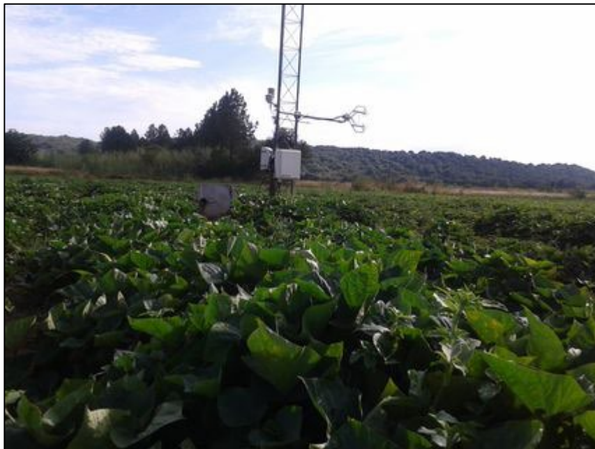
Figure 2.10: Eddy covariance system measuring sweet potato evapotranspiration at the Agricultural Research Council – Vegetable, Industrial and Medicinal Plants research station (Photo taken by Mr Ntsieni Mulovhedzi).
