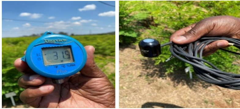
Figure 6.6: Tinytag datalogger used to measure air temperature and relative humidity (left) and net radiometer used to measure solar radiation (right), in the Moringa trials at ARC-VIMP.
