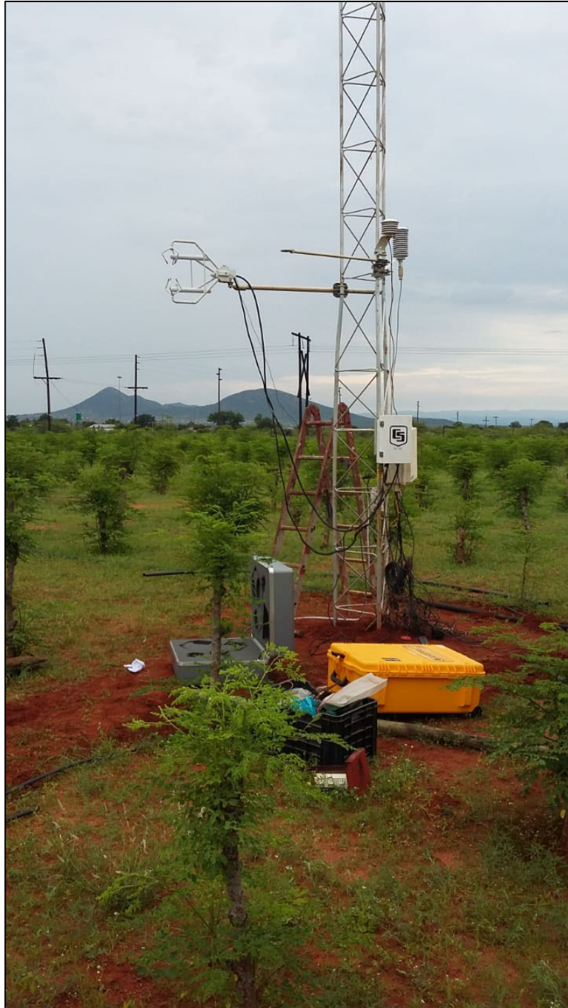
Figure 3.5: A complete eddy covariance system installed on an 8-year old Moringa stand to measure evapotranspiration at Tooseng research site, Limpopo province (Picture taken by Mr Ntsieni Mulovhedzi).
