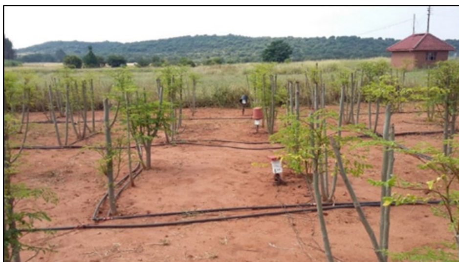
Figure 2.6: Capacitive 10-Hs soil water sensors connected to an EM-50 datalogger to automatically monitor Moringa soil water content under different deficit irrigation regimes (Photo taken by Mr Ntsieni Mulovhedzi).
