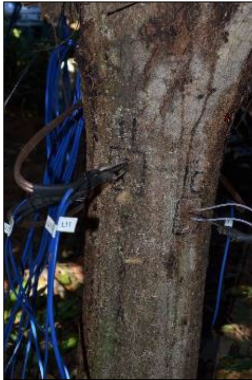
Figure 2.14: Thermocouples and a heat temperature probe installed on the trunk of a seven-year-old macadamia tree to measure sap flow movement through the xylem (Photo taken by Dr Nadia Araya).
