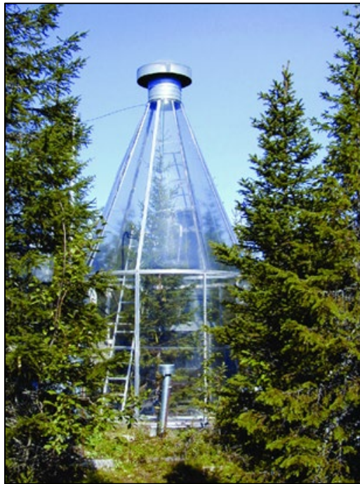
Figure 2.13: A whole-tree chamber quantifying fluxes of CO 2 and H 2 O (Photo taken from https://www.researchgate.net/publication/259153552 on 12/12/2021).
