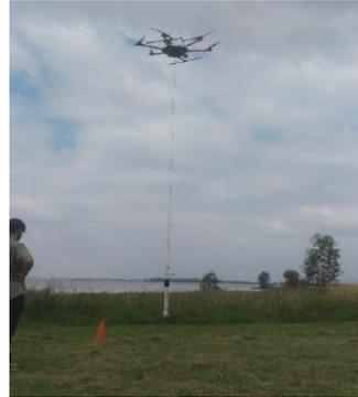
**Figure 44:** LS Multicopter Matrice 600 Pro Drone fully winch/jig loaded on take-off and water sampling operations.
