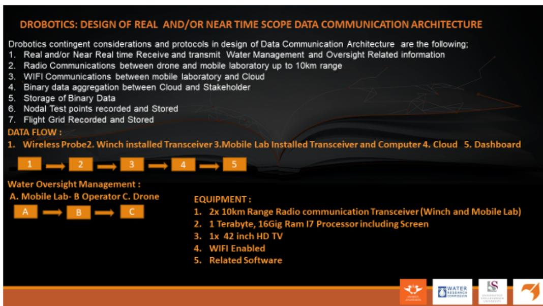
**Figure 59: Drobotics communication protocols and architecture.**
