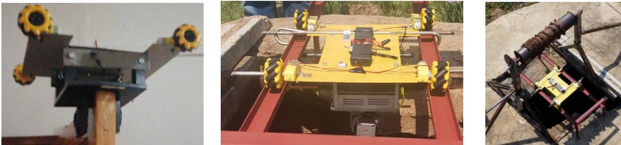
**Figure 66:** A) Printed winch housing attached to alternate platform (left). B) Winch system attached to modular rail cart platform (middle). C) Modular rail cart platform for static water sources and infrastructure.
