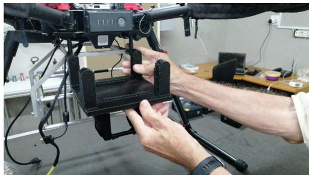
**Figure 48:** Winch 3D Printed Housing
