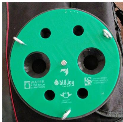
**Figure 56:** Prototype of multiprobe-holding jig.
