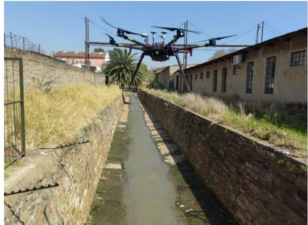
**Figure 43:** A) Matrice 600 Pro Drone; B) 5 kg weighted hover test using RTK at 5 m .
