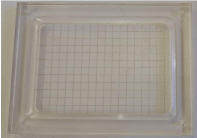
**Figure 3.5 De Grisse Counting dish used to count sporocarps.**
