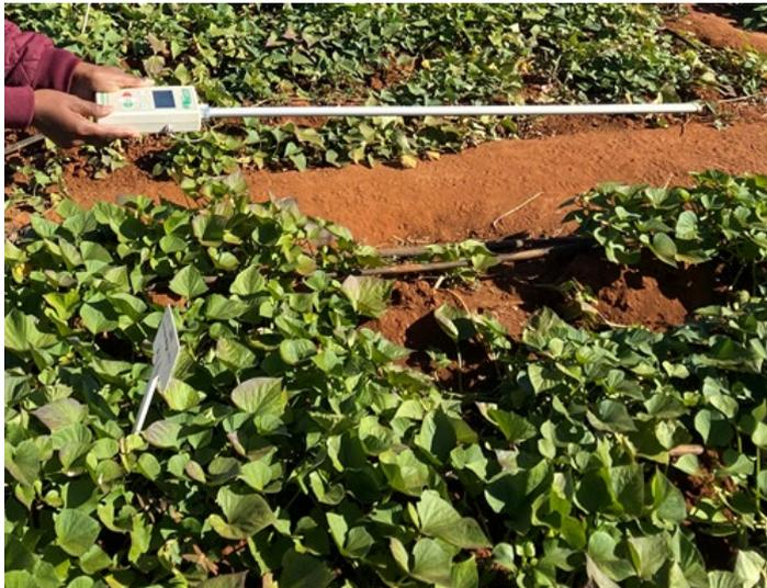
**Figure 4.6 Ceptometer used to take reading above plants.**
