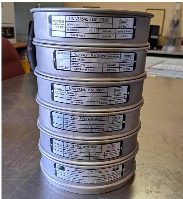
**Figure 3.4** Test sieves of different sizes were used for wet sieving of AMF.
