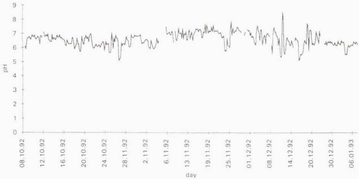
Figure 24: The pH of neutralised water during Phase 2.
