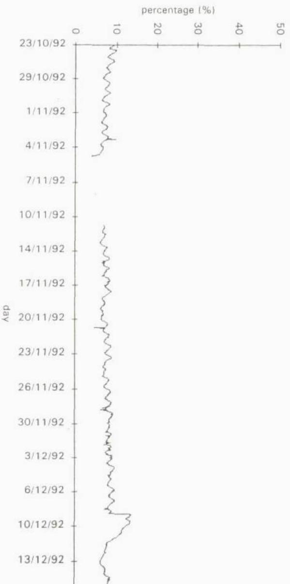
Figure 34: LPR data of Rand Water Board water (Phase 2).
