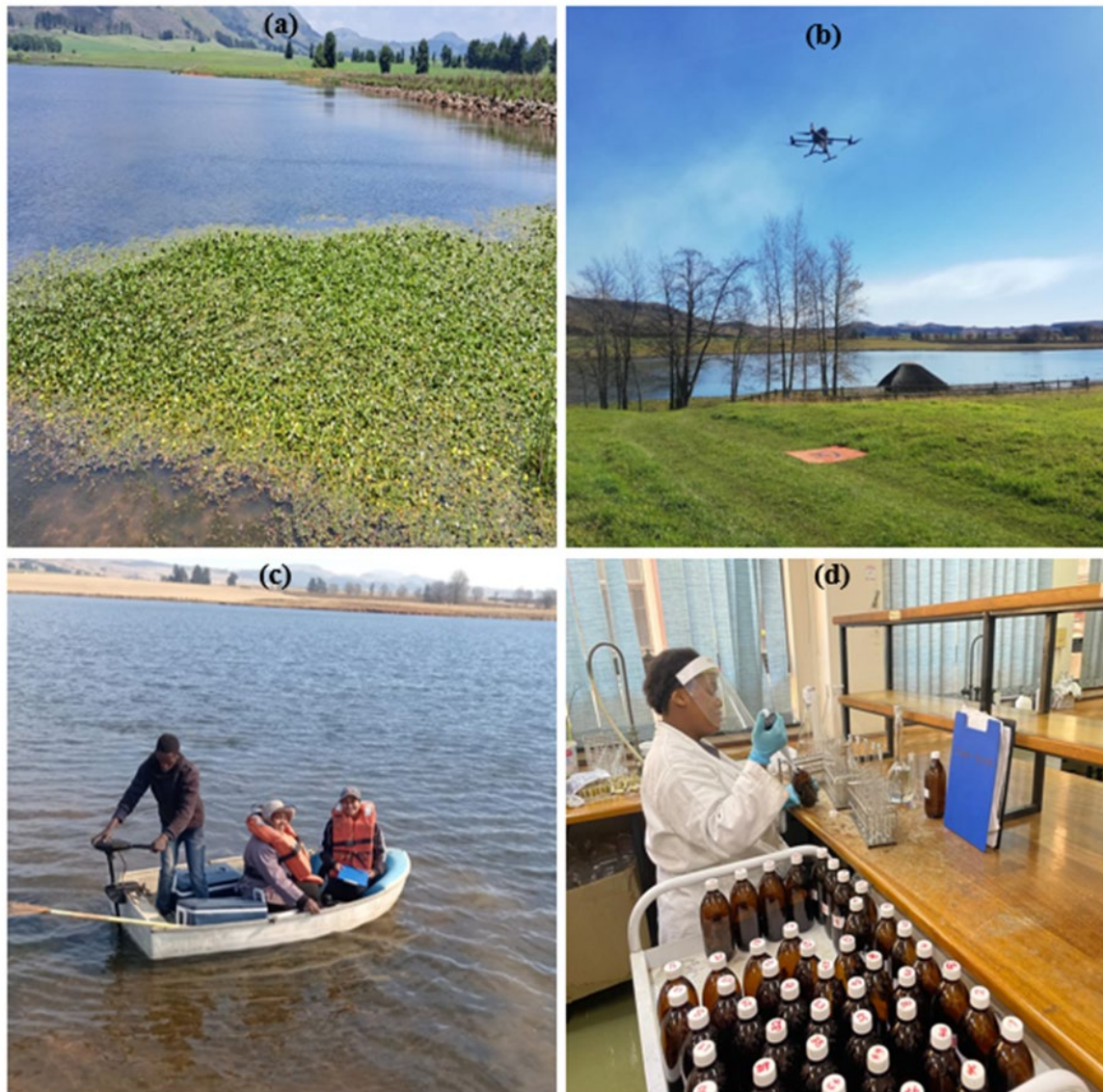
Figure 4-3 (a) Field observation of the dam showing water hyacinth presence, (b) UAV deployed for high-resolution multispectral imaging over the dam, (c) Field team navigating to sampling points within the dam by boat, (d) Laboratory analysis of water samples collected from the field
