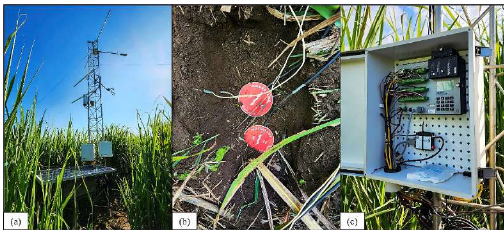
Figure 5.1 (a) EC system, (b) installation of the soil HFPs, and (c) CR3000 datalogger
