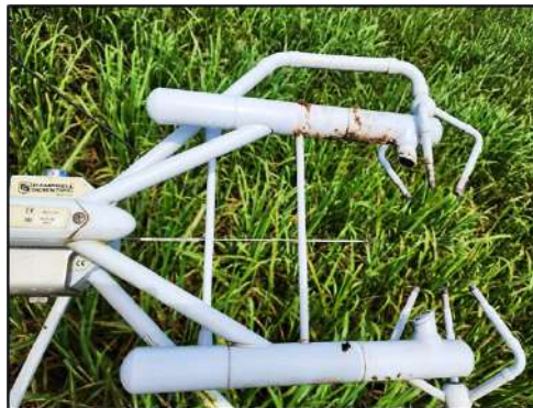
Figure D2 Soil accumulation on the co-located 3-D sonic anemometer and CO 2 /H 2 O Open-Path Gas Analyser, attributed to avian interference, resulting in data loss from January 23, 2024, to February 2, 2024
