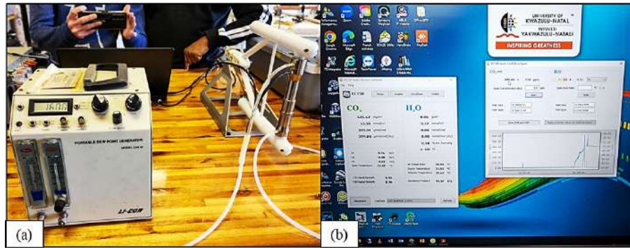
Figure D1 Calibration setup for the CO 2 /H 2 O Open-Path Gas Analyzer (EC150) using (a) the LI-610 Dew Point Generator and (b) the LI-670 Flow Control Unit, with data acquisition and analysis conducted via the EC100 Series Monitor Software
