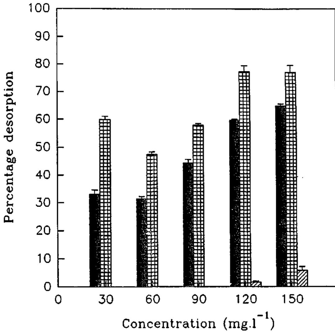
Fig. 5.9. Percentage desorption of Cr<sup>3+</sup> from sludge 2 by acetic acid (■), hydrochloric acid (▣) and deionised water (▨).
