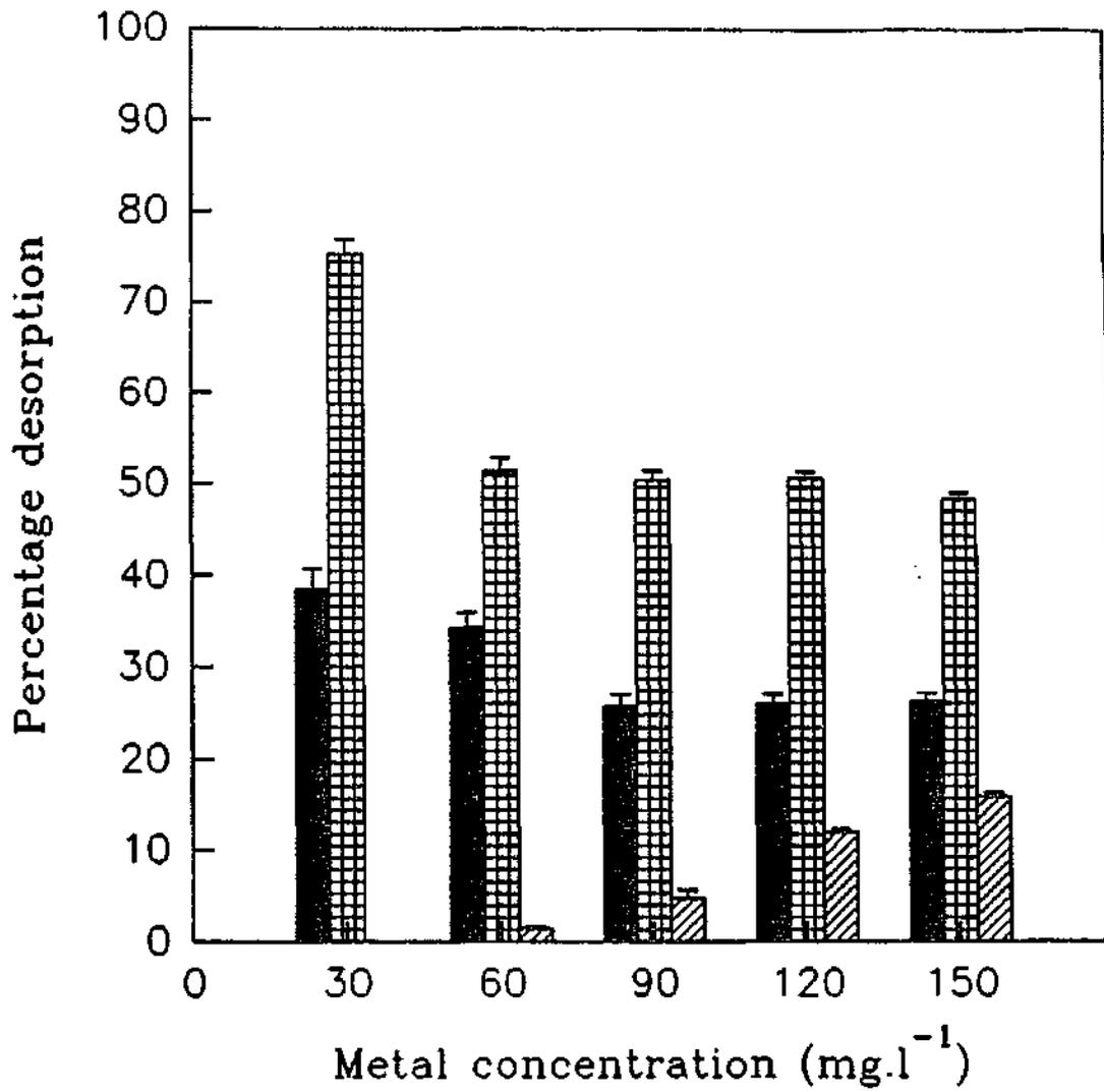
Fig. 5.22. Percentage desorption of Cr<sup>6+</sup> from sludge 3 by acetic acid (■), hydrochloric acid (▣) and deionised water (▨).
