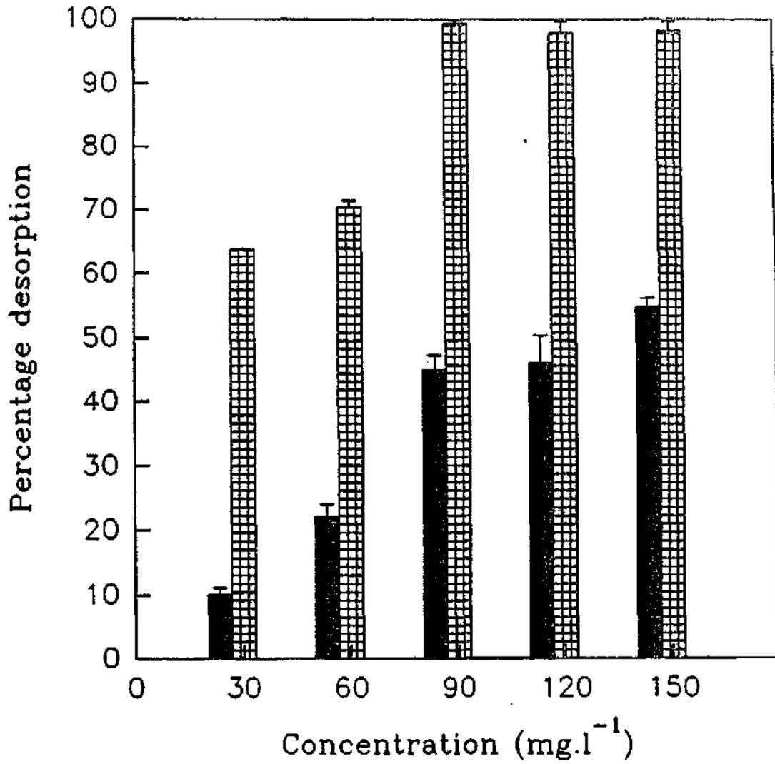
Fig. 5.10. Percentage desorption of Cr<sup>3+</sup> from sludge 3 by acetic acid (■), hydrochloric acid (▣) and deionised water (▨).
