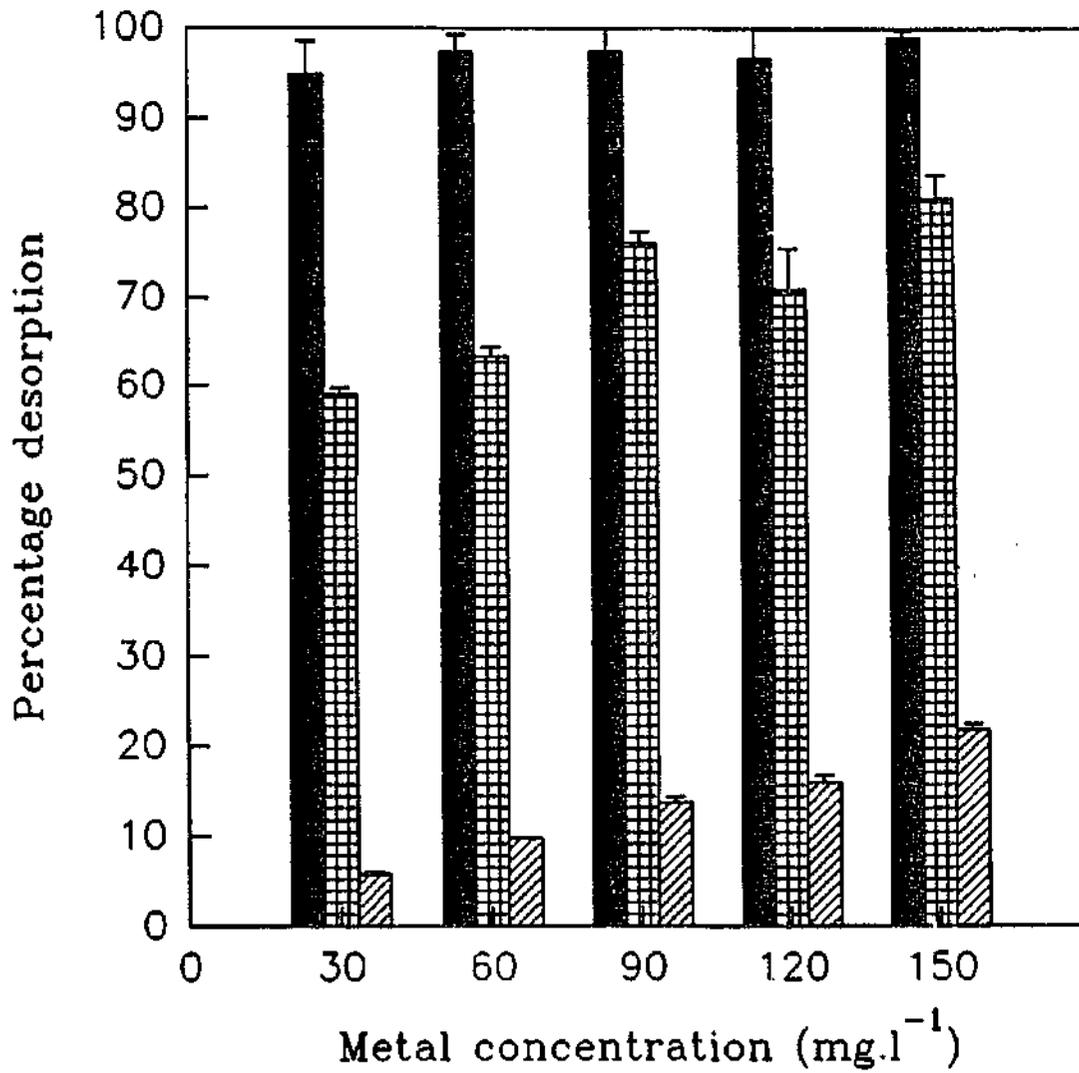
Fig. 5.15. Percentage desorption of Ni from sludge 4 by acetic acid (■), hydrochloric acid (▣) and deionised water (▨).
