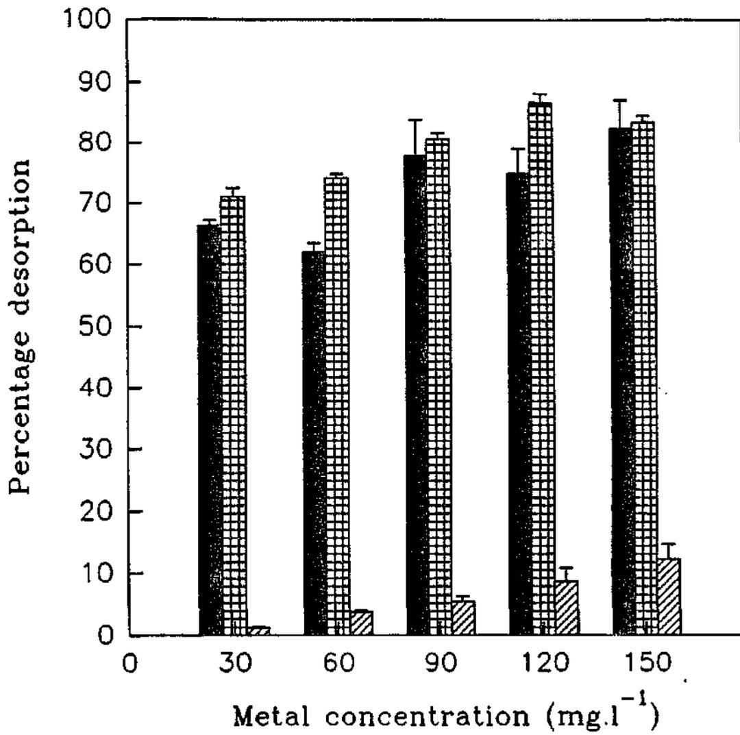
Fig. 5.3. Percentage desorption of Zn from sludge 4 by acetic acid (■), hydrochloric acid (▣) and deionised water (▨).
