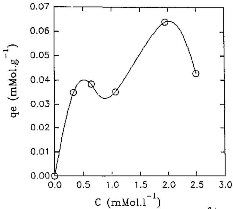
Fig. 4. 117. Adsorption isotherm for Cr<sup>6+</sup> uptake from solution by sludge 8.
