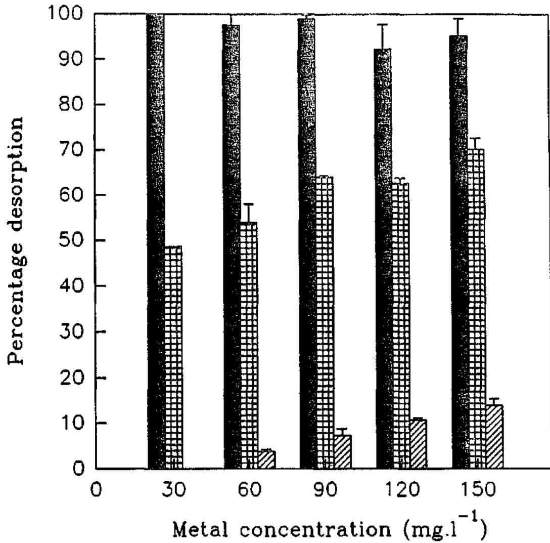
Fig. 5.14. Percentage desorption of Ni from sludge 3 by acetic acid (■), hydrochloric acid (▣) and deionised water (▨).
