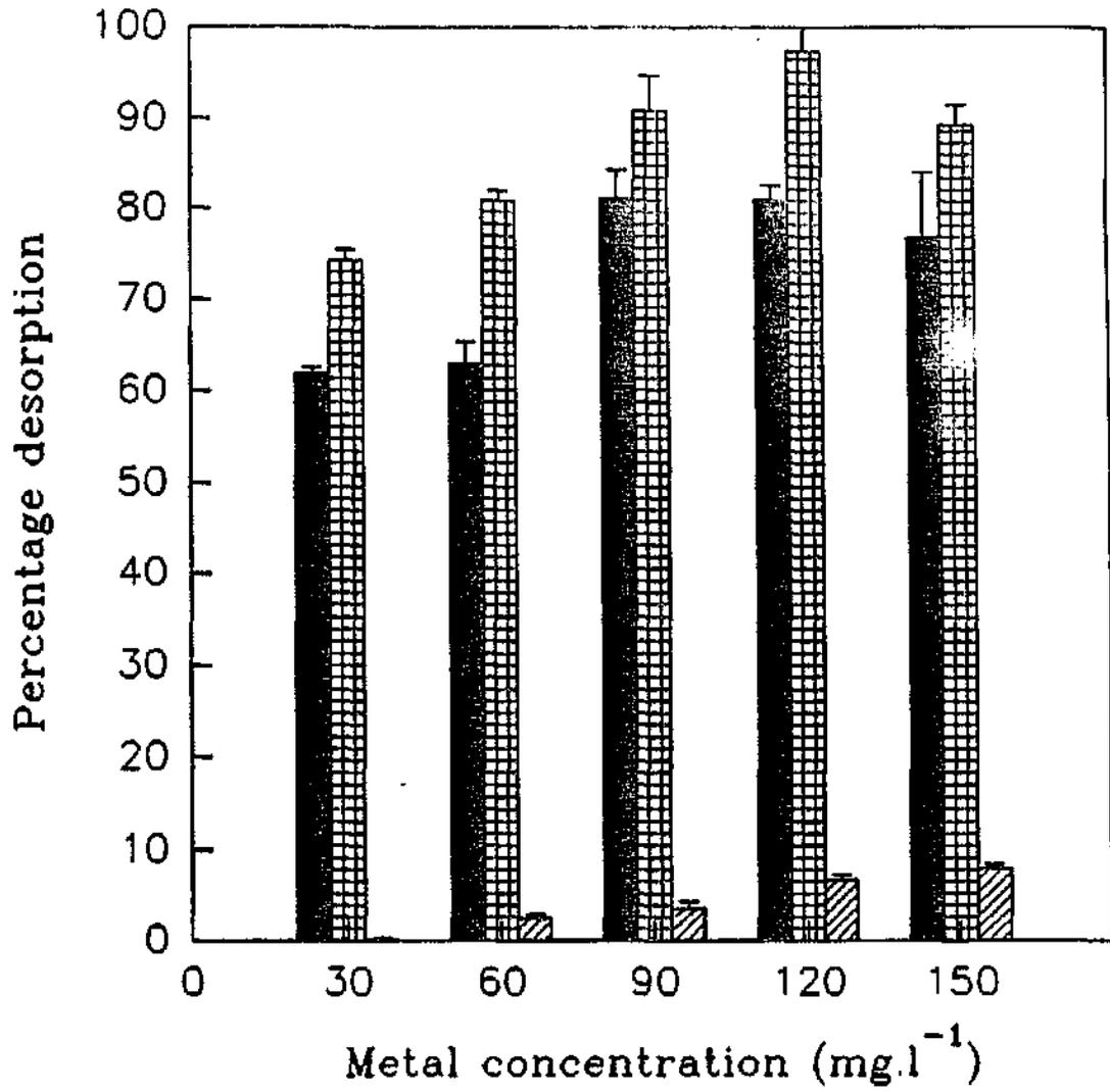
Fig. 5.4. Percentage desorption of Zn from sludge 9 by acetic acid (■), hydrochloric acid (▣) and deionised water (▨).
