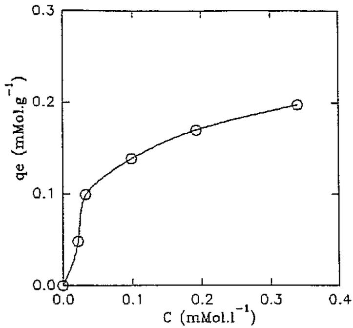
Fig. 4. 29. Adsorption isotherm for Cd uptake from solution by sludge 4.
