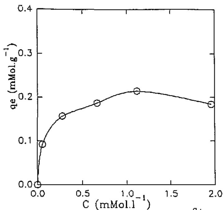
Fig. 4. 89. Adsorption isotherm for Cr<sup>3+</sup> uptake from solution by sludge 4.
