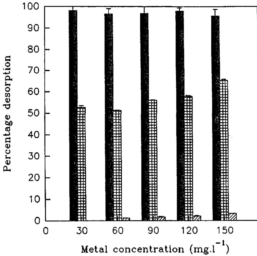
Fig. 5.17. Percentage desorption of Cu from sludge 2 by acetic acid (■), hydrochloric acid (▣) and deionised water (▨).
