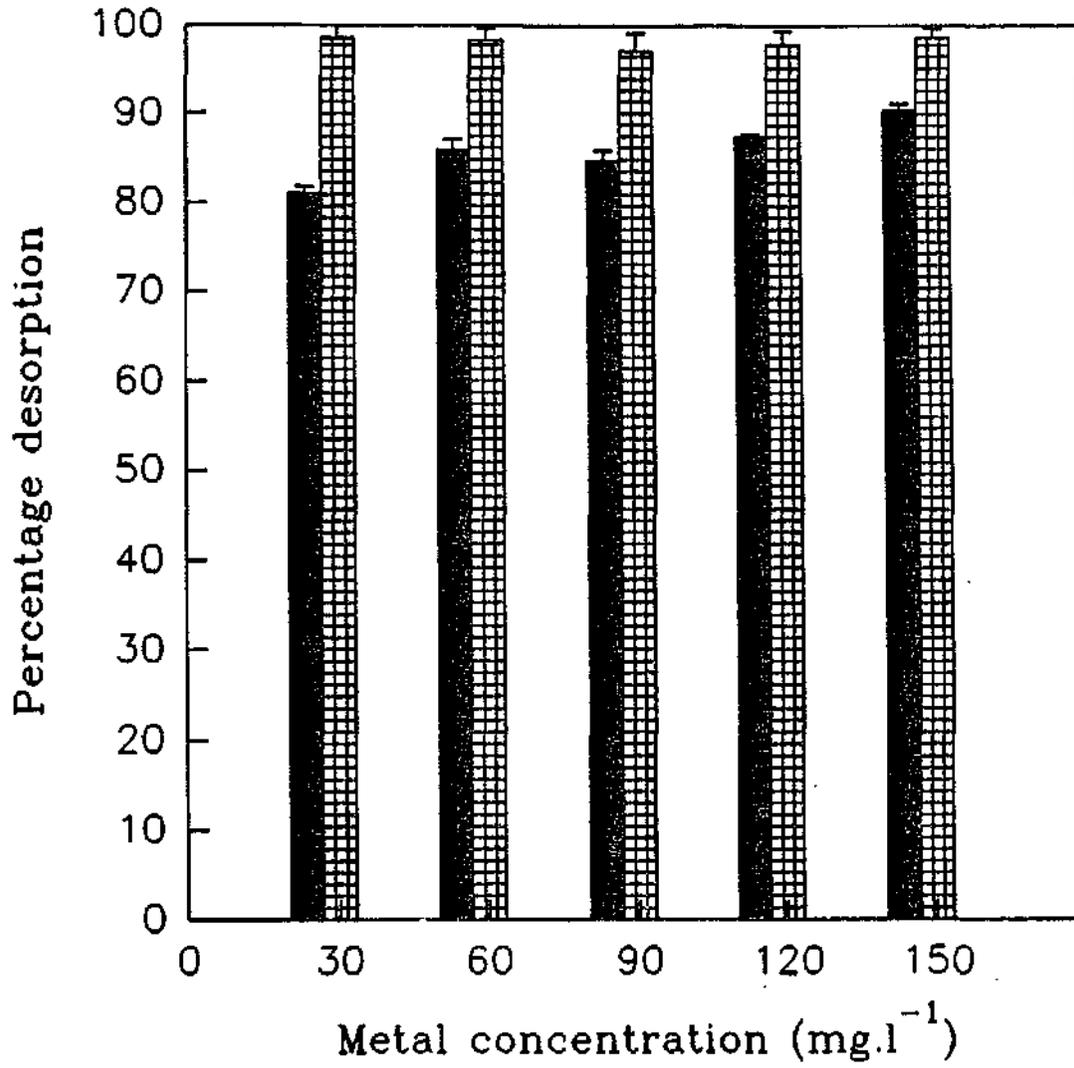
Fig. 5.5. Percentage desorption of Cd from sludge 2 by acetic acid (■), hydrochloric acid (▣) and deionised water (▨).
