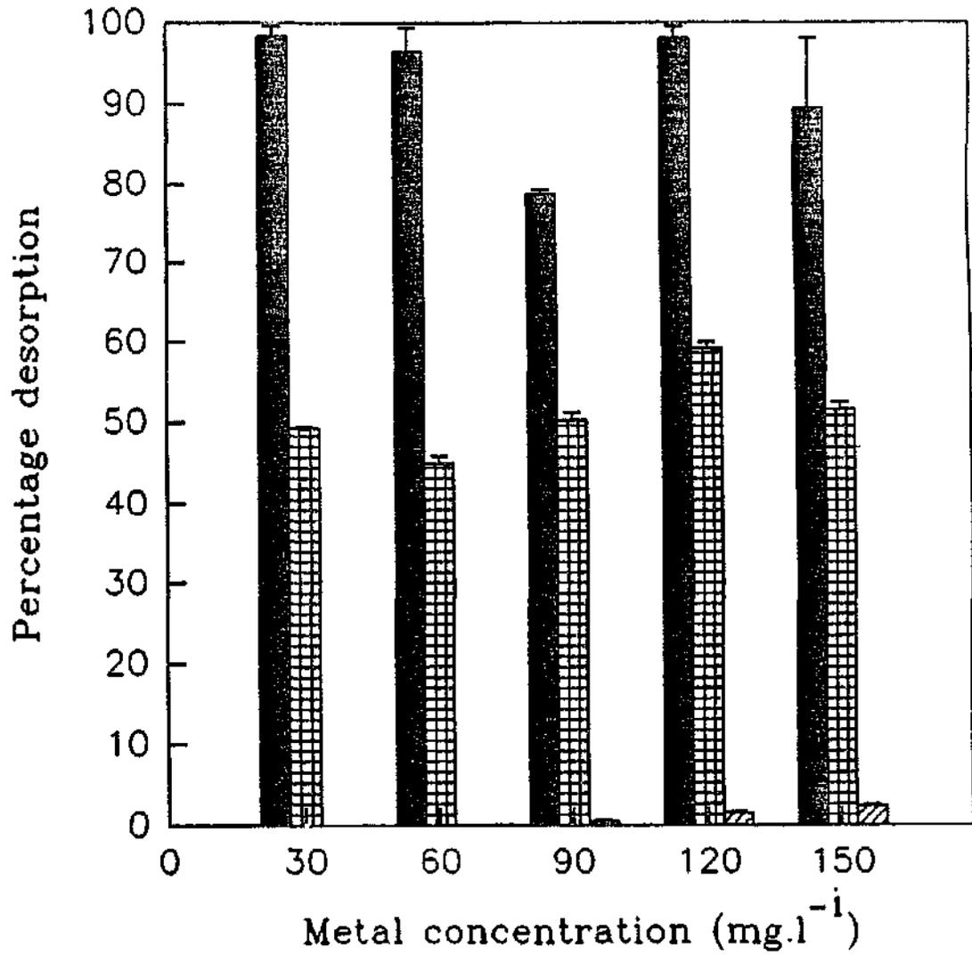
Fig. 5.18. Percentage desorption of Cu from sludge 3 by acetic acid (■), hydrochloric acid (▣) and deionised water (▨).
