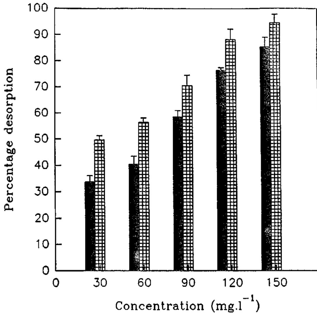
Fig. 5.12. Percentage desorption of Cr<sup>3+</sup> from sludge 9 by acetic acid (■), hydrochloric acid (▣) and deionised water (▨).
