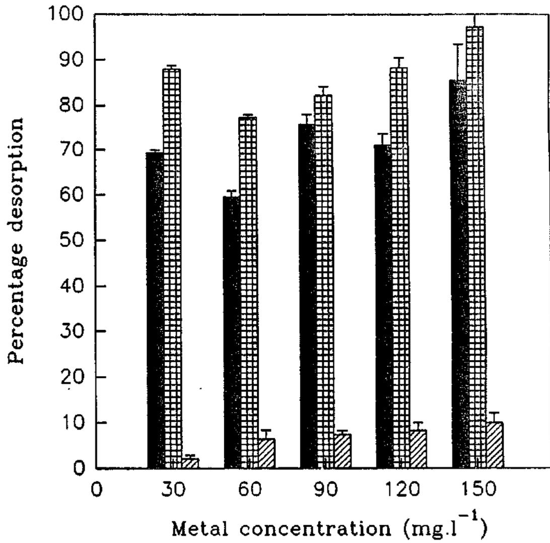
Fig. 5.2. Percentage desorption of Zn from sludge 3 by acetic acid (■), hydrochloric acid (▣) and deionised water (▨).
