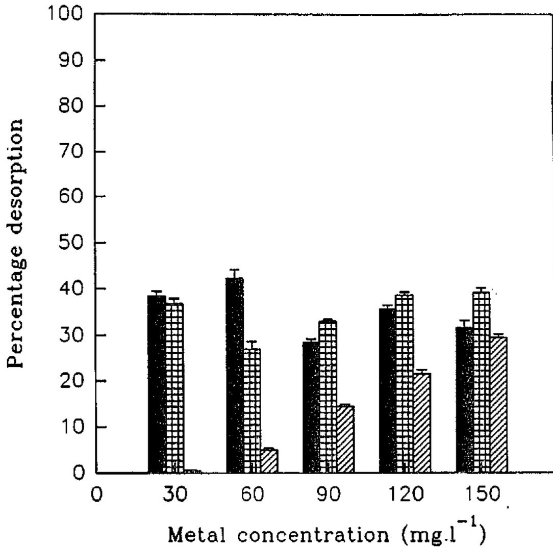
Fig. 5.23. Percentage desorption of Cr<sup>6+</sup> from sludge 4 by acetic acid (■), hydrochloric acid (▣) and deionised water (▨).
