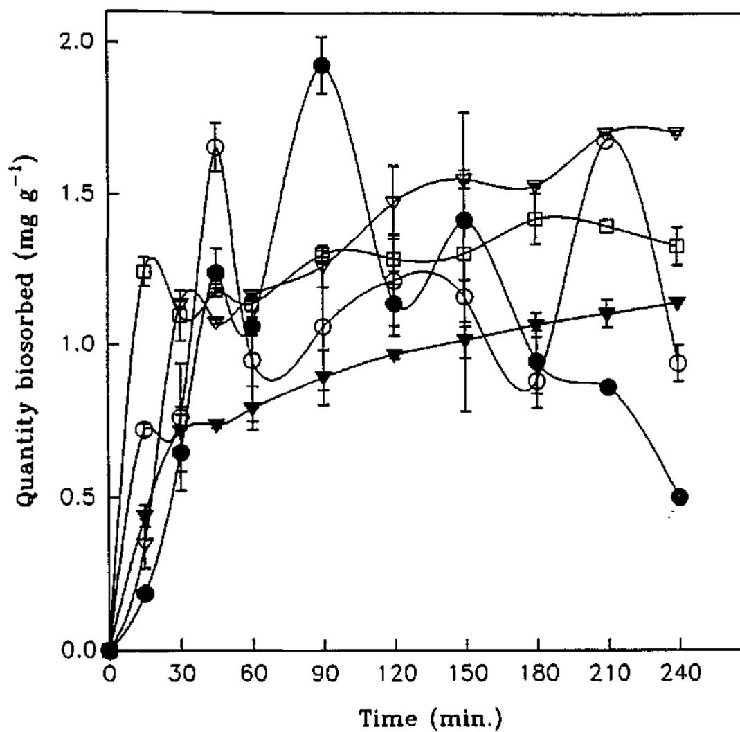
Fig. 7.1. Quantity of Zn biosorbed from synthetic effluent by sludges at concentrations of 5 000 (○), 10 000 (●), 15 000 (▽), 20 000 (▼) and 25 000 (□) mg l<sup>-1</sup>.
