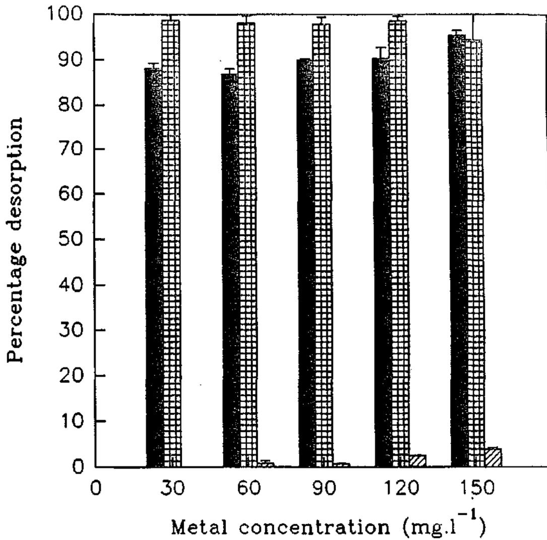
Fig. 5.8. Percentage desorption of Cd from sludge 9 by acetic acid (■), hydrochloric acid (▣) and deionised water (▨).
