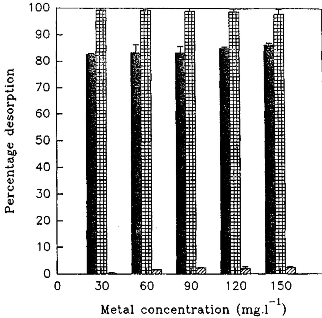
Fig. 5.6. Percentage desorption of Cd from sludge 3 by acetic acid (■), hydrochloric acid (▣) and deionised water (▨).
