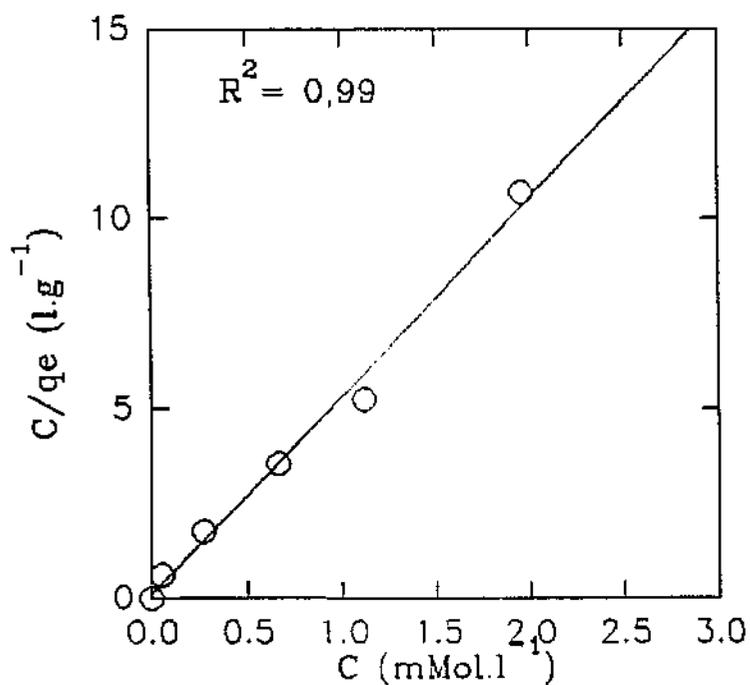
Fig. 4. 90. Reciprocal isotherm for Cr<sup>3+</sup> uptake from solution by sludge 4.
