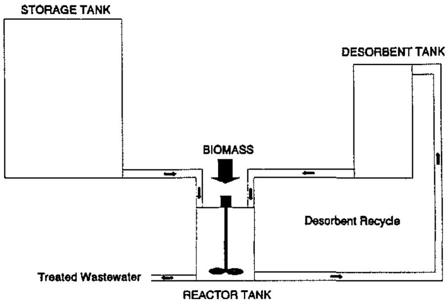
Fig. 9.1 Schematic representation of biological treatment process for the removal of metal ions from industrial wastewaters
