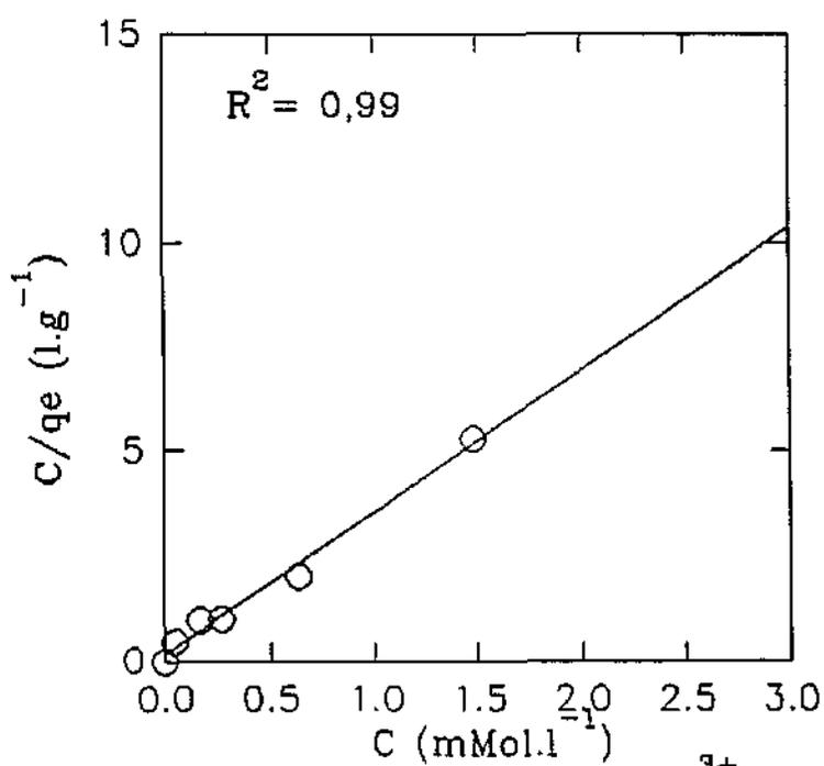
Fig. 4. 88. Reciprocal isotherm for  $\text{Cr}^{3+}$  uptake from solution by sludge 3.
