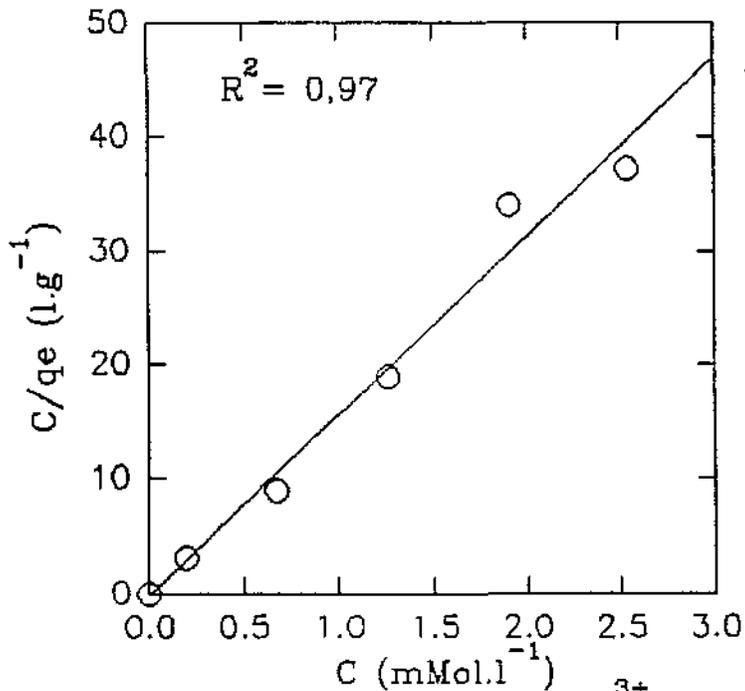
Fig. 4. 96. Reciprocal isotherm for  $\text{Cr}^{3+}$  uptake from solution by sludge 7.
