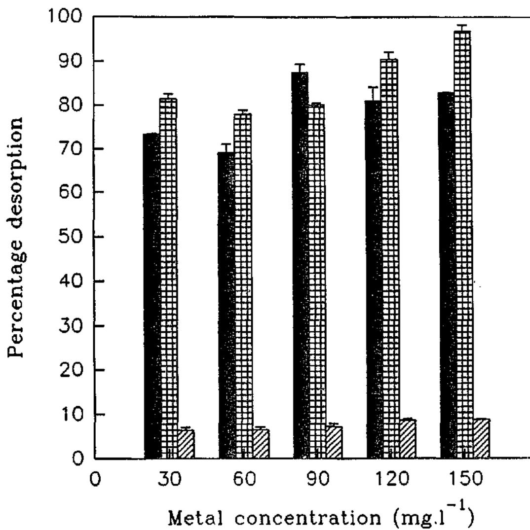
Fig. 5.1. Percentage desorption of Zn from sludge 2 by acetic acid (■), hydrochloric acid (▣) and deionised water (▨).
