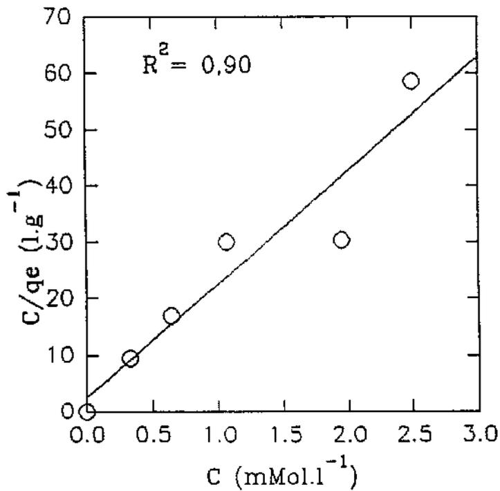
Fig. 4. 118. Reciprocal isotherm for Cr<sup>6+</sup> uptake from solution by sludge 8.
