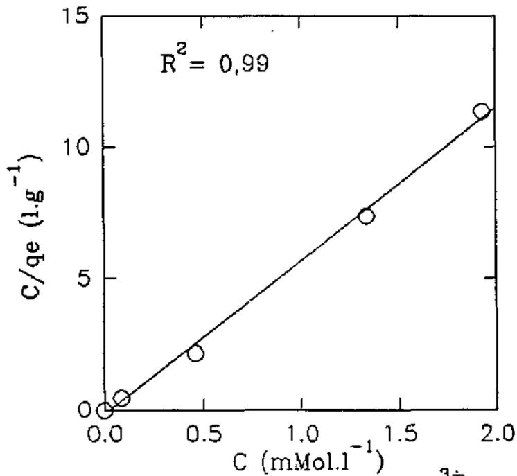
Fig. 4. 92. Reciprocal isotherm for Cr<sup>3+</sup> uptake from solution by sludge 5.
