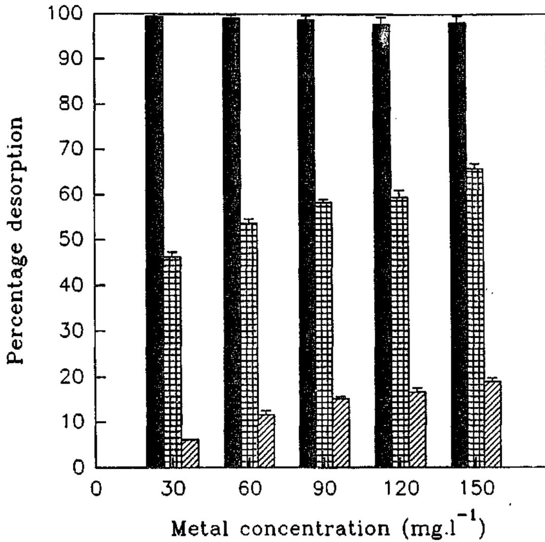
Fig. 5.13. Percentage desorption of Ni from sludge 2 by acetic acid (■), hydrochloric acid (▣) and deionised water (▨).
