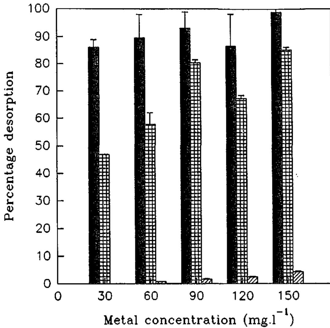
Fig. 5.19. Percentage desorption of Cu from sludge 4 by acetic acid (■), hydrochloric acid (▣) and deionised water (▨).
