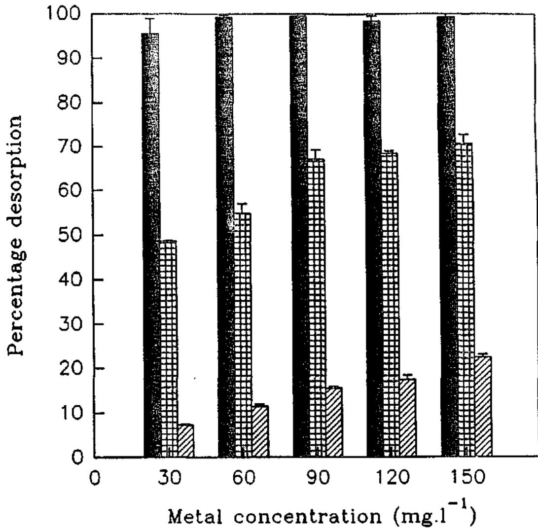
Fig. 5.16. Percentage desorption of Ni from sludge 9 by acetic acid (■), hydrochloric acid (▣) and deionised water (▨).
