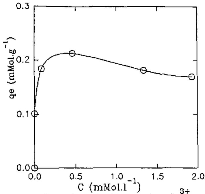
Fig. 4. 91. Adsorption isotherm for Cr<sup>3+</sup> uptake from solution by sludge 5.
