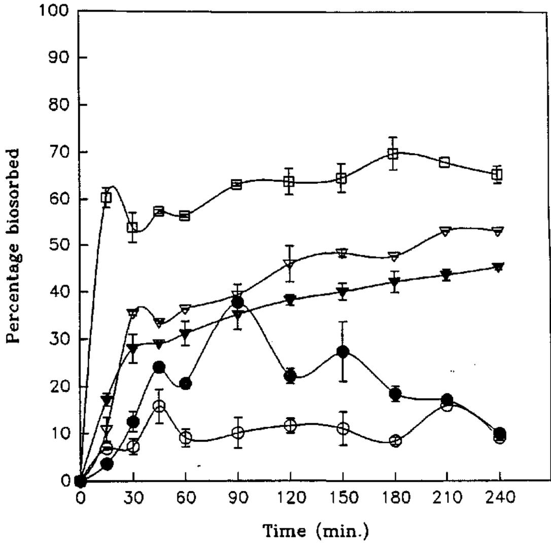
Fig. 7.2. Percentage Zn biosorbed from synthetic effluent by sludges at concentrations of 5 000 (○), 10 000 (●), 15 000 (▽), 20 000 (▼) and 25 000 (□) mg  $l^{-1}$ .
