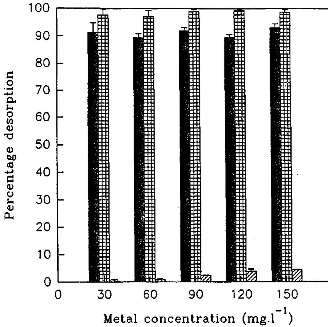
Fig. 5.7. Percentage desorption of Cd from sludge 4 by acetic acid (■), hydrochloric acid (▣) and deionised water (▨).
