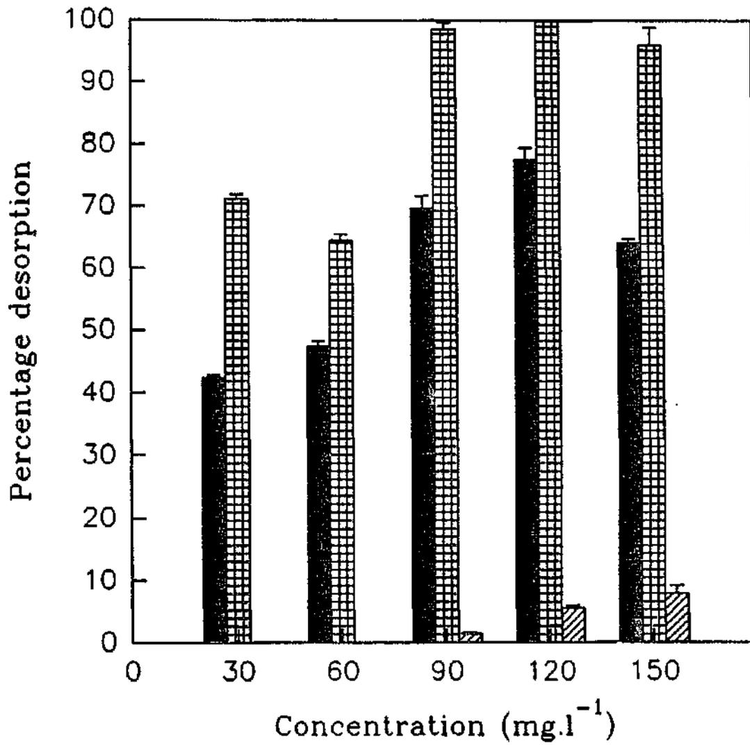
Fig. 5.11. Percentage desorption of Cr<sup>3+</sup> from sludge 4 by acetic acid (■), hydrochloric acid (▣) and deionised water (▨).
