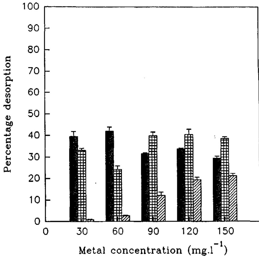
Fig. 5.24. Percentage desorption of Cr<sup>4+</sup> from sludge 9 by acetic acid (■), hydrochloric acid (▣) and deionised water (▨).
