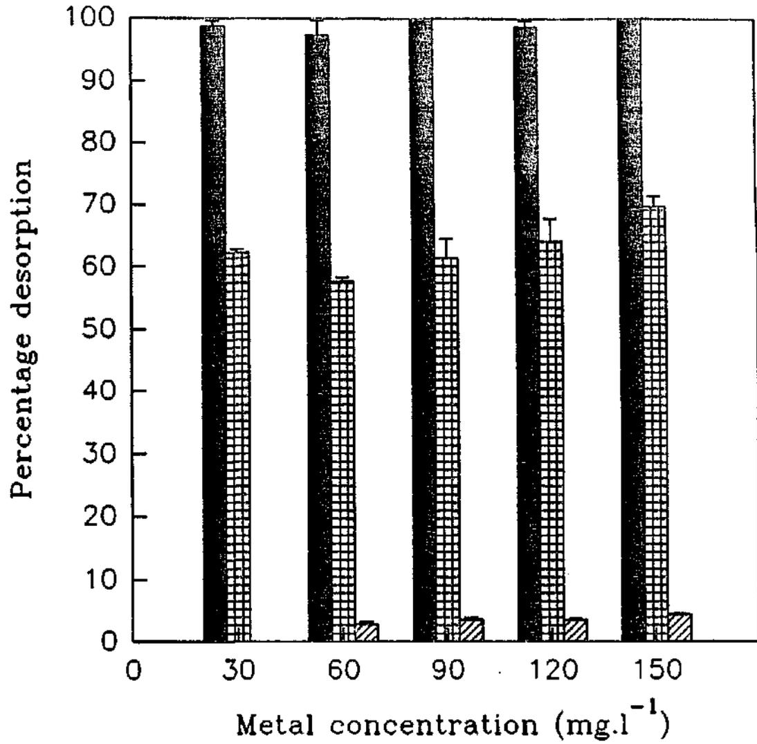
Fig. 5.20. Percentage desorption of Cu from sludge 9 by acetic acid (■), hydrochloric acid (▣) and deionised water (▨).
