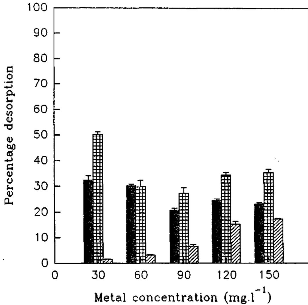
Fig. 5.21. Percentage desorption of Cr<sup>6+</sup> from sludge 2 by acetic acid (■), hydrochloric acid (▣) and deionised water (▨).
