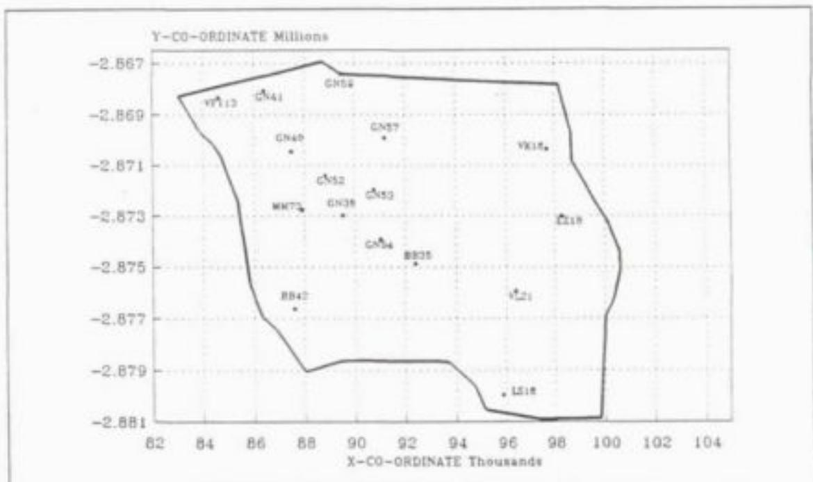
Figure 7 Grootfontein Compartment Observation Borehole Positions
