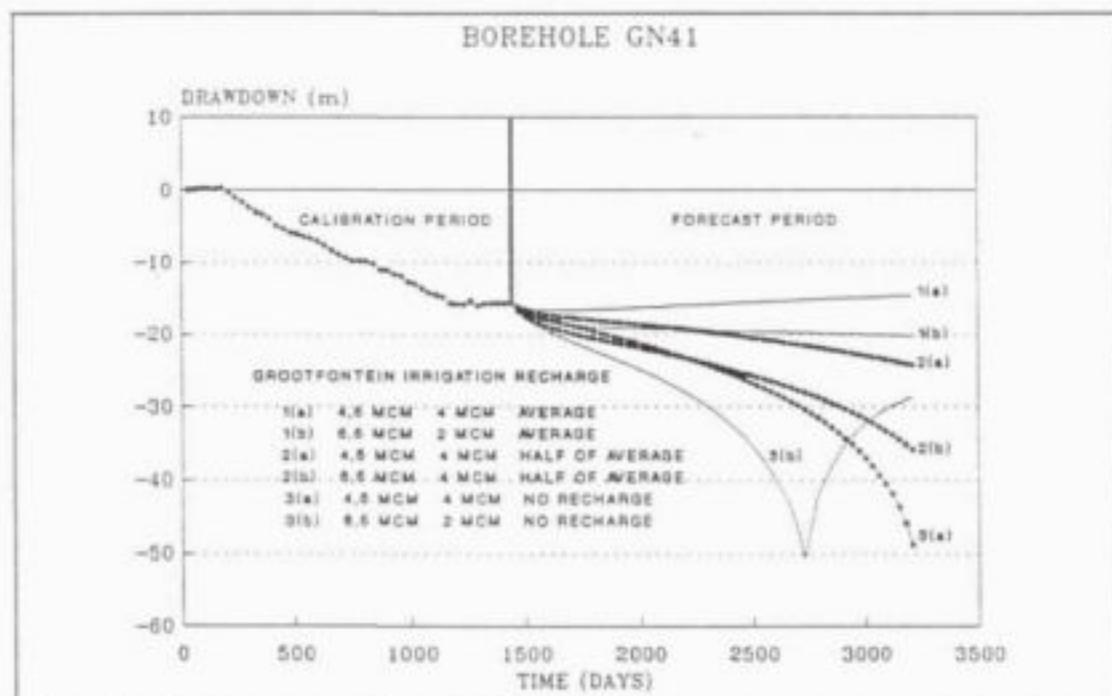
Figure 26 Forecast water level - GN41
