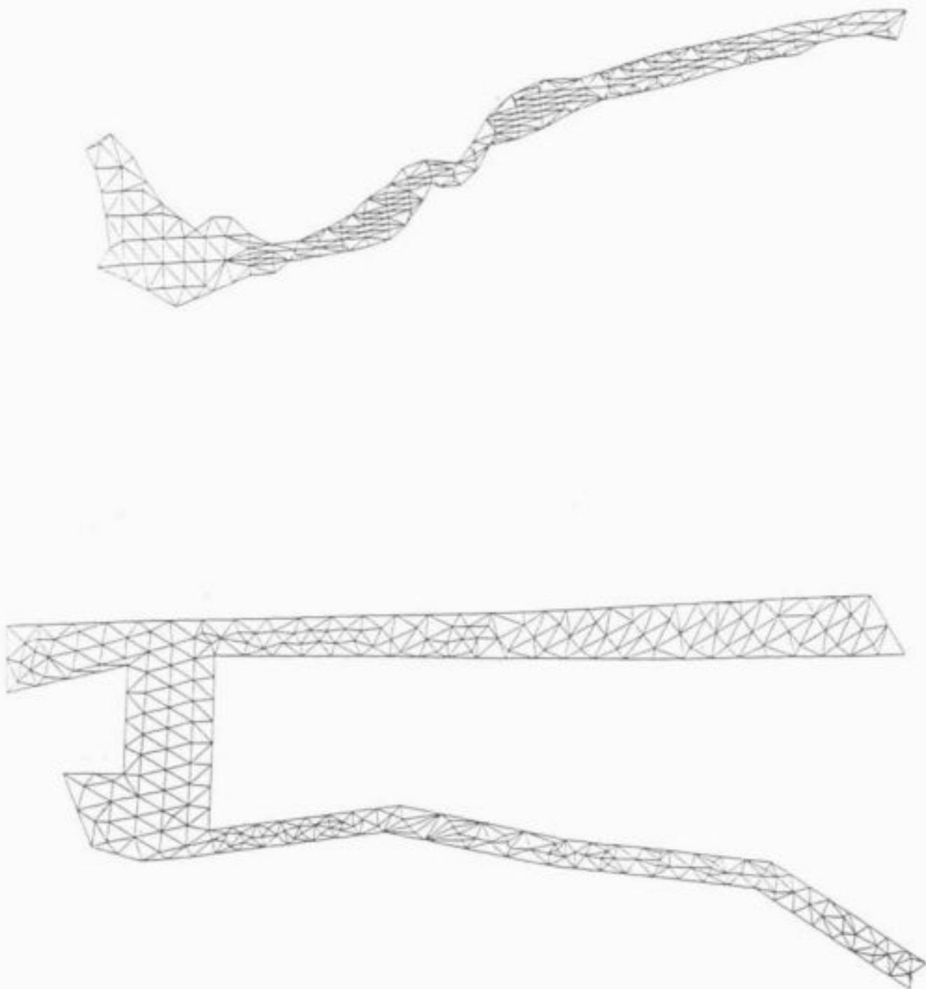
Fig. 1.4. Finite element meshes of the Greefswald- and Otjiwarongo Marble aquifer generated with the program AQUA-NET.
