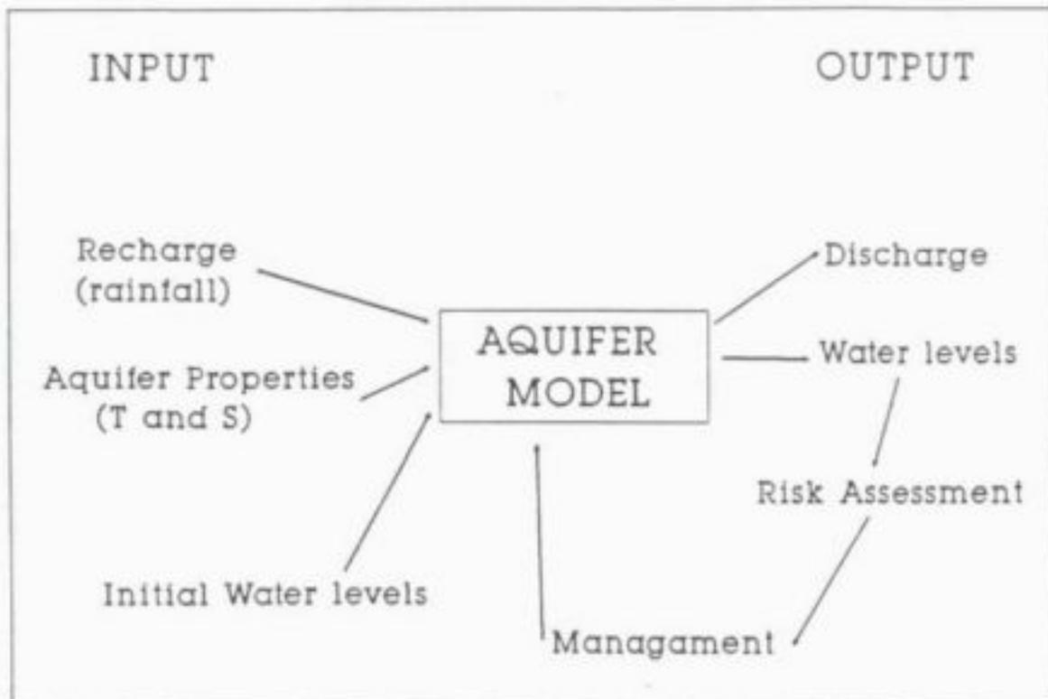
Figure 1: Schematic representation of the different components of an aquifer risk assessment model
