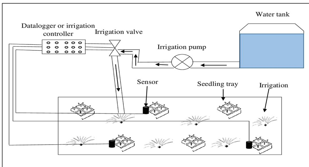
**Figure 2.** An automated irrigation system capable of measuring the water content of the substrate in the small-volume nursery containers, and controlling the opening and closing of irrigation valves according to lower and upper set points
