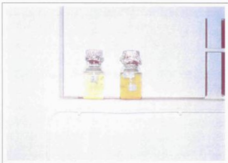
Colour removal by the Dynamic Filter on 18/11/96-r - filtrate, raw water
