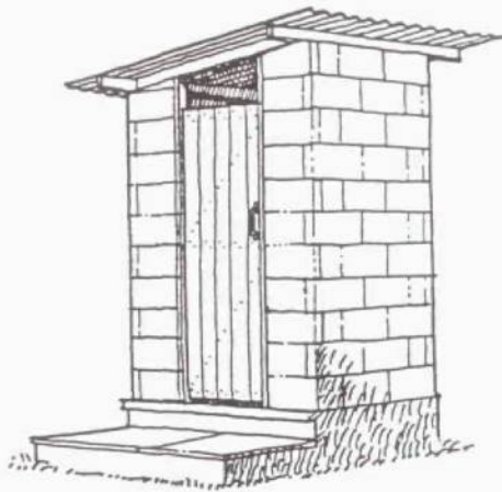
A shelter of concrete blocks with roof of corrugated-iron sheets
