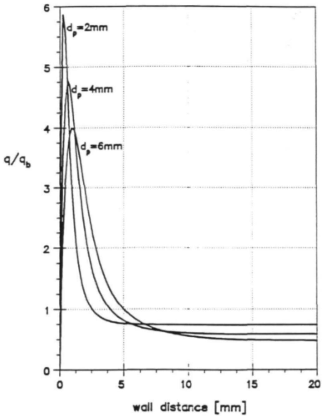
Figure 8: Flow profiles for granular medium between parallel plates.
