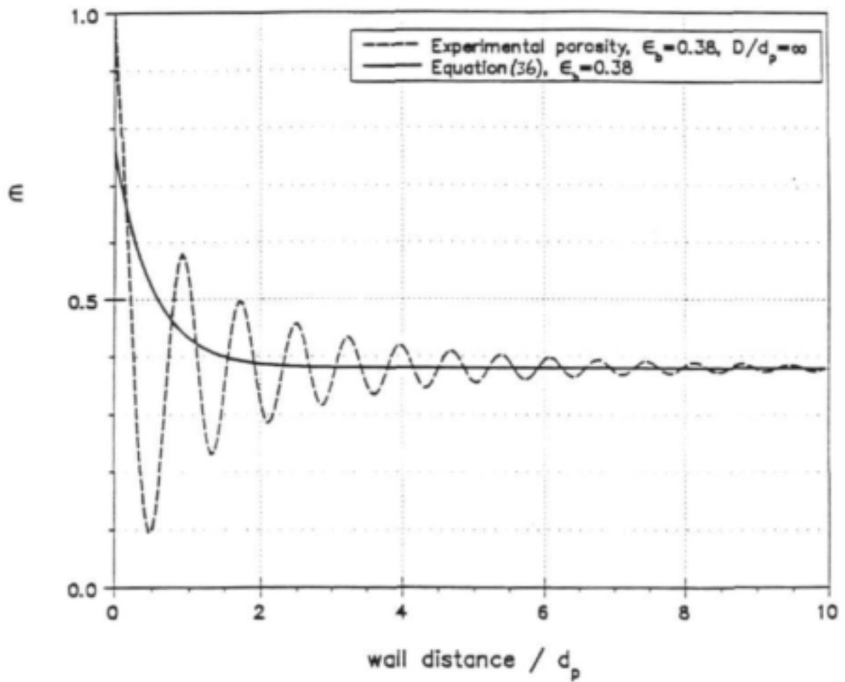
Figure 4: Porosity distribution near external wall.
