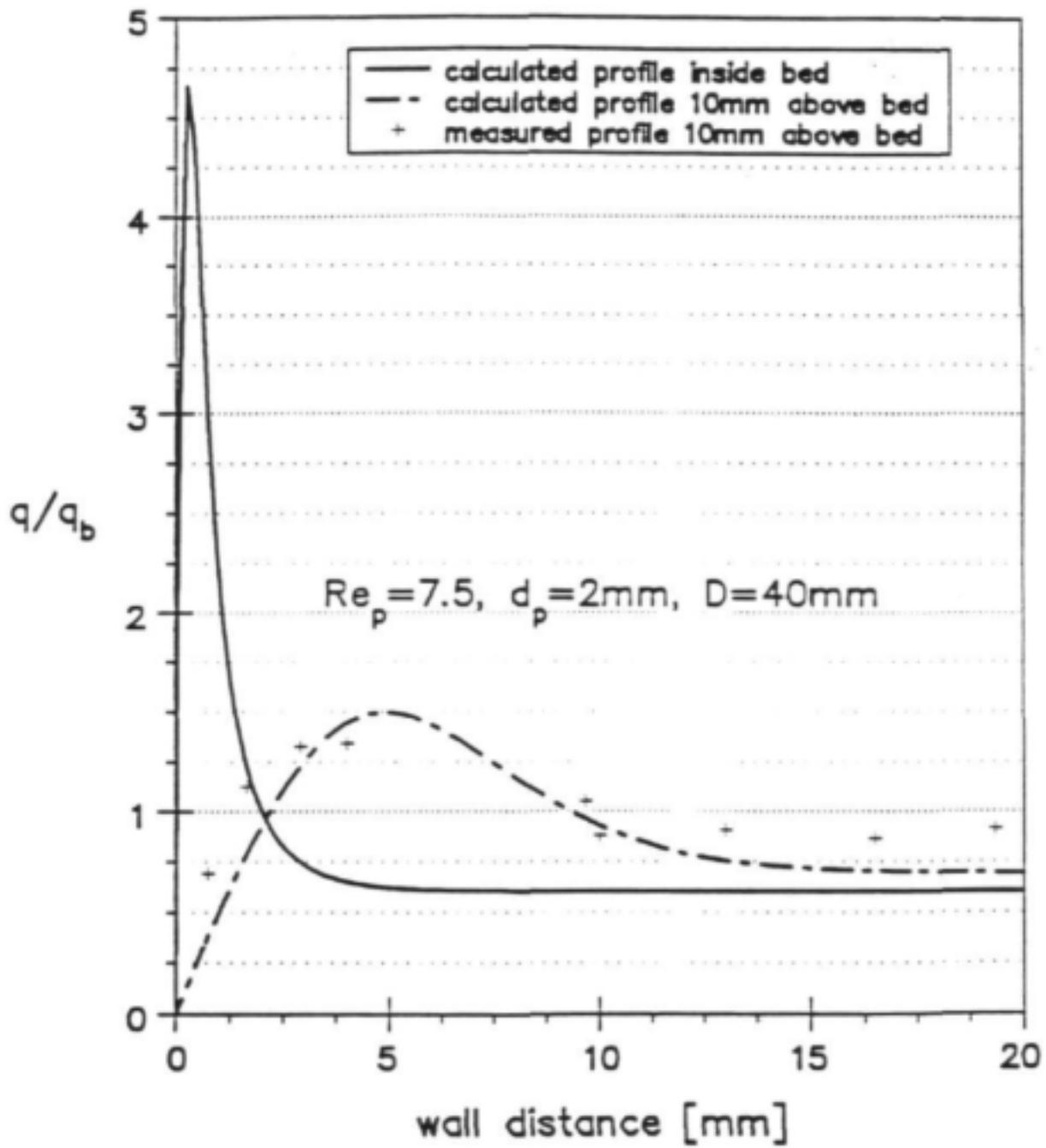
Figure 10: Flow profile inside and 10mm above a tubular packed bed.
