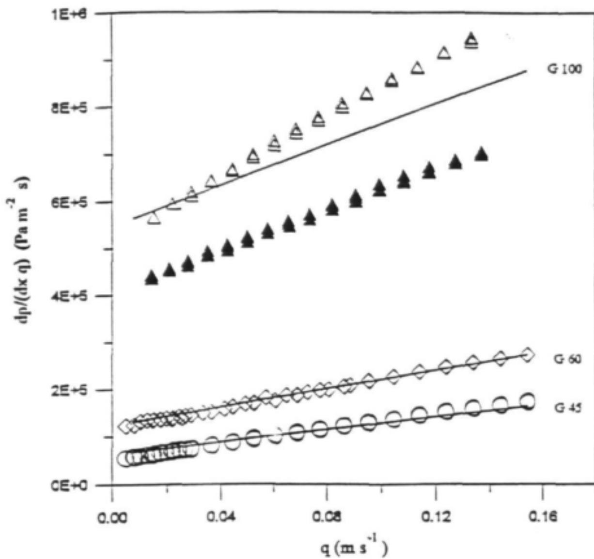
Figure 1: Comparison of results for isotropic foams with the grades (G pores per inch) indicated.
