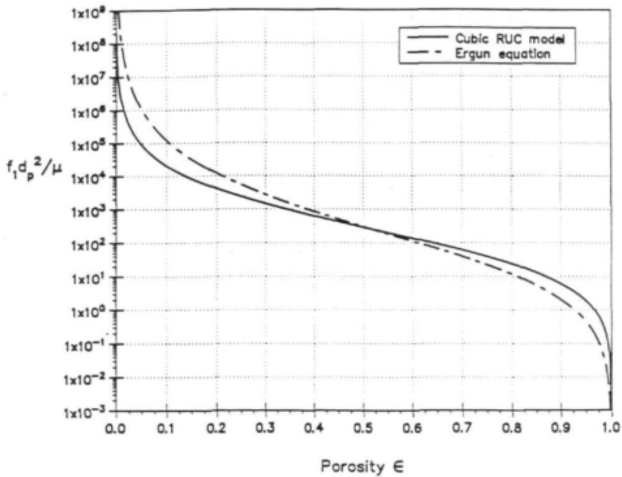
Figure 6: Viscous drag in granular medium.
