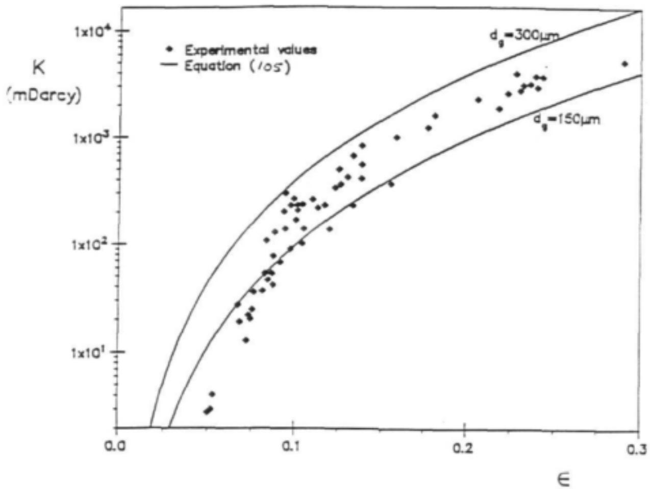
Figure 13: Experimental results for Fontainebleau sandstone.
