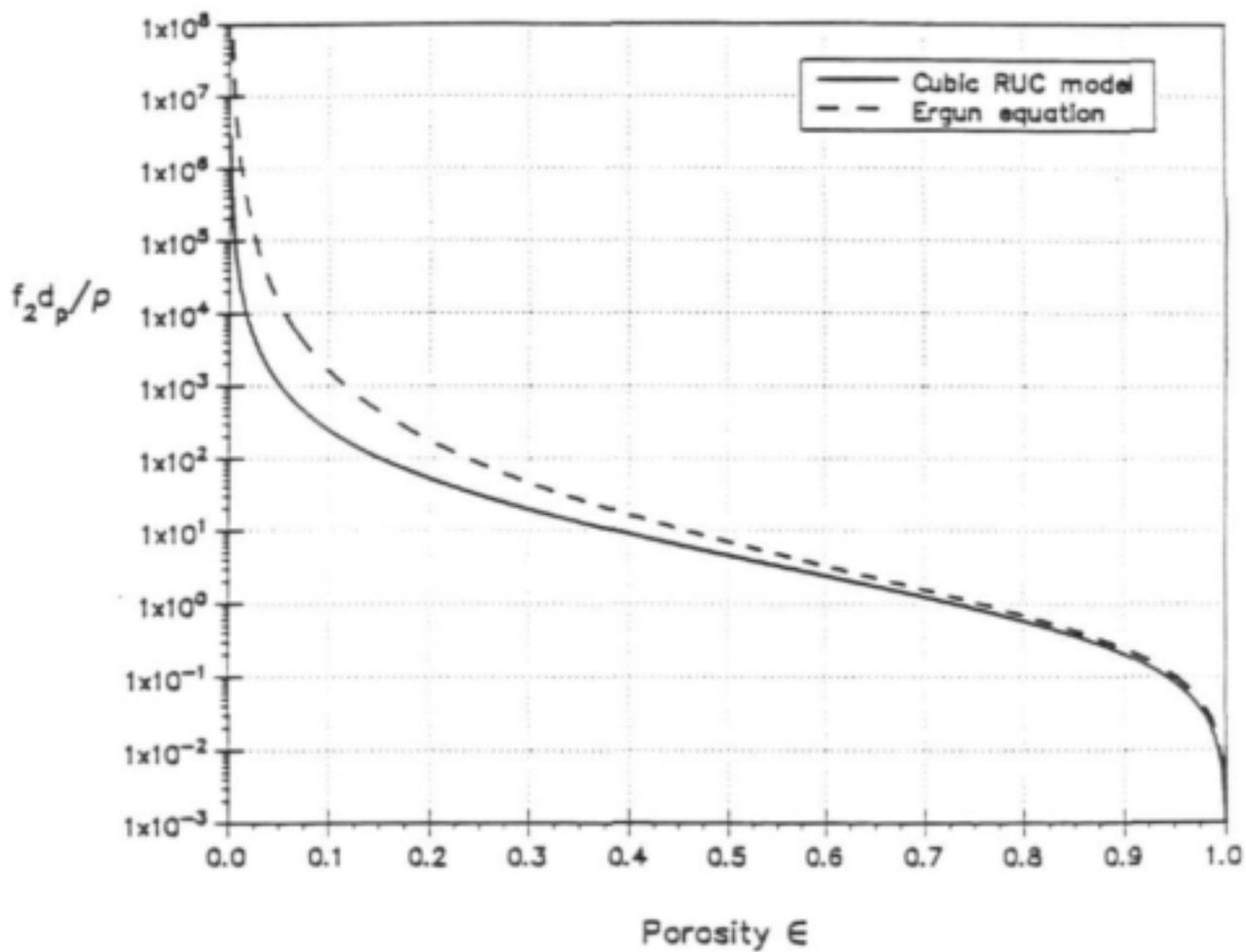
Figure 7: Form drag in granular medium.
