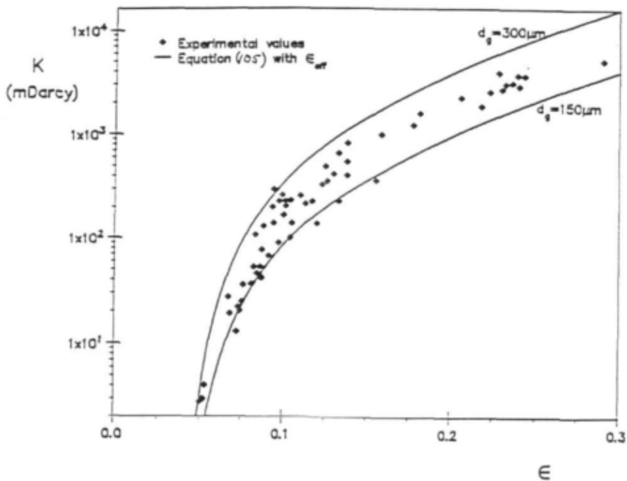
Figure 15: Final results for Fontainebleau sandstone.
