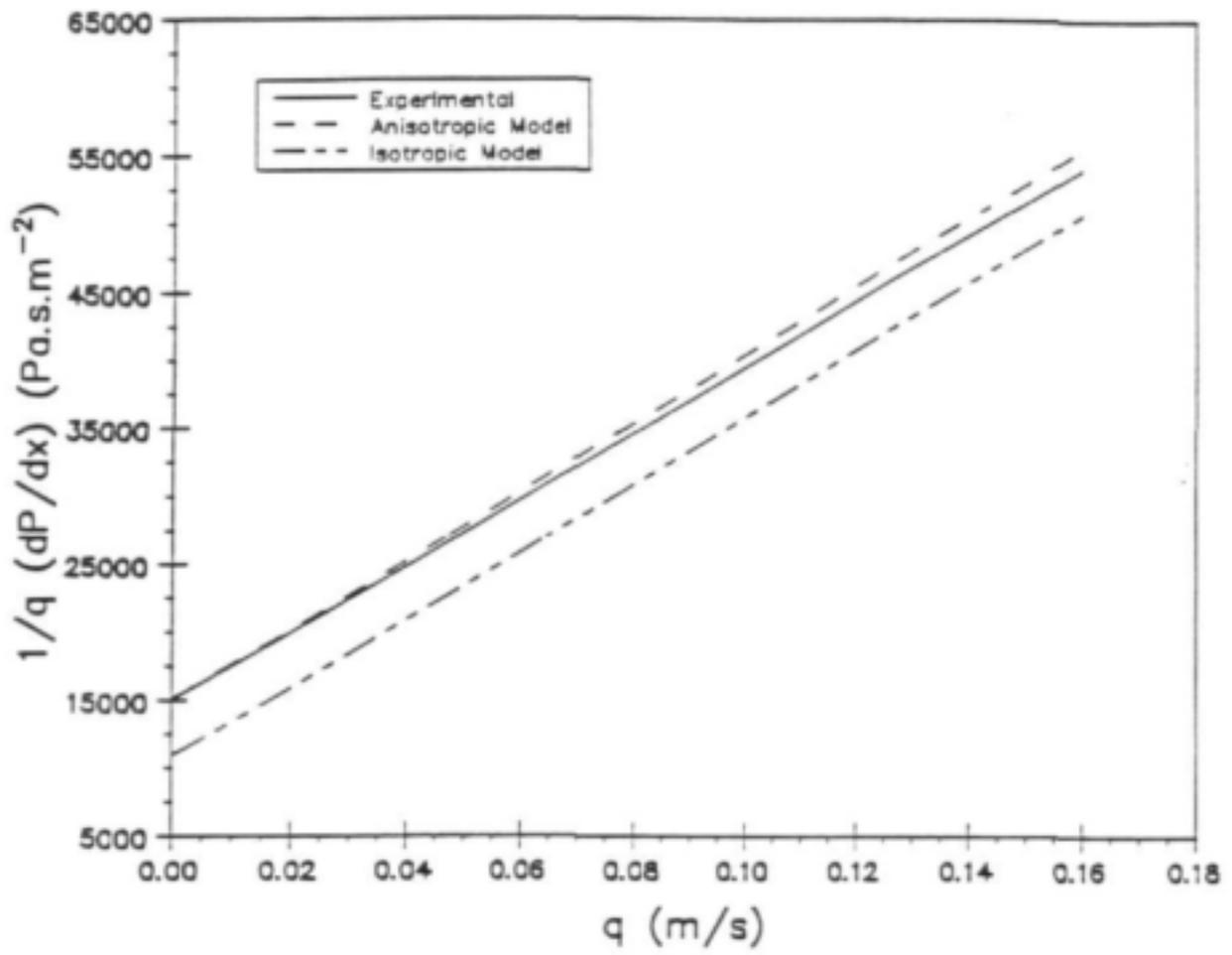
Figure 3: Comparative results for anisotropic foamlike material.
