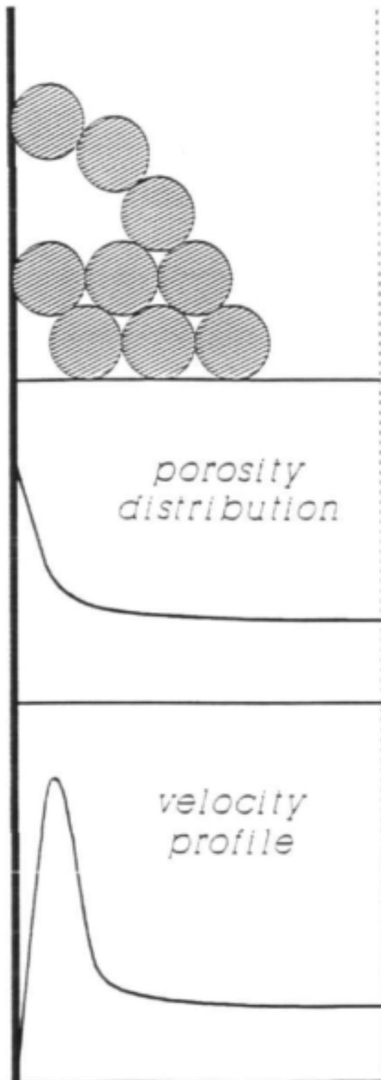
Figure 5: Effects induced by external wall for granular media.
