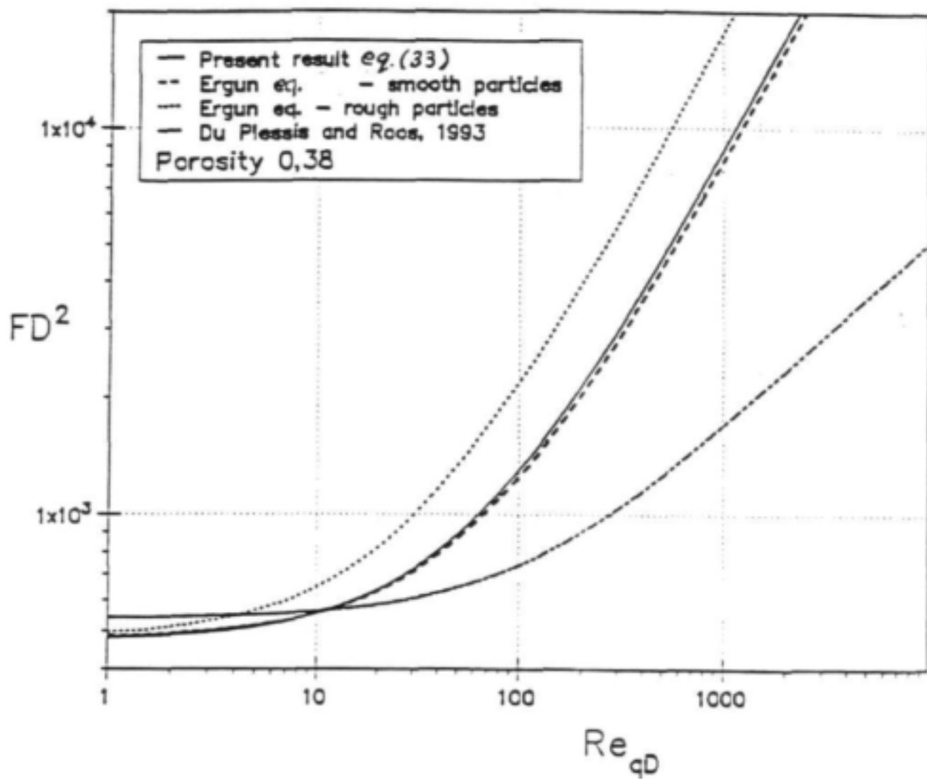
Figure 2: Comparison of results against Ergun equation for granular media.
