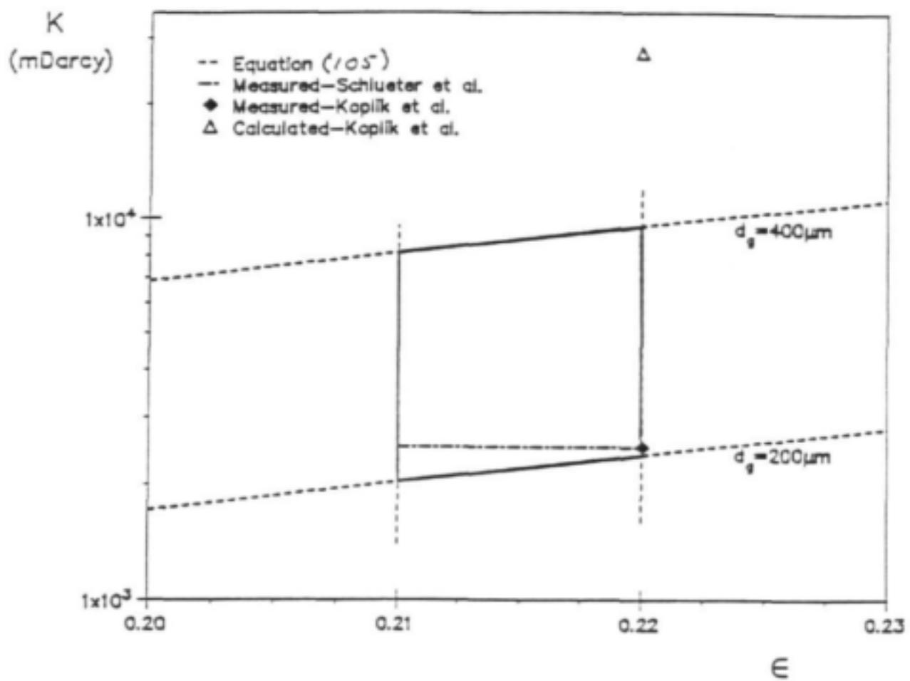
Figure 11: Results for Massillon sandstone.
