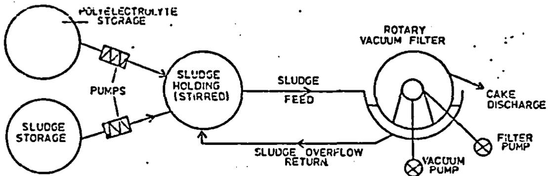
Figure 2.3 Rotary drum vacuum filter test equipment
