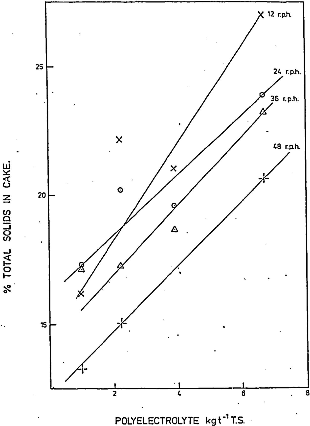
DEWATERING OF UNTREATED SLUDGE BY VACUUM FILTRATION.
