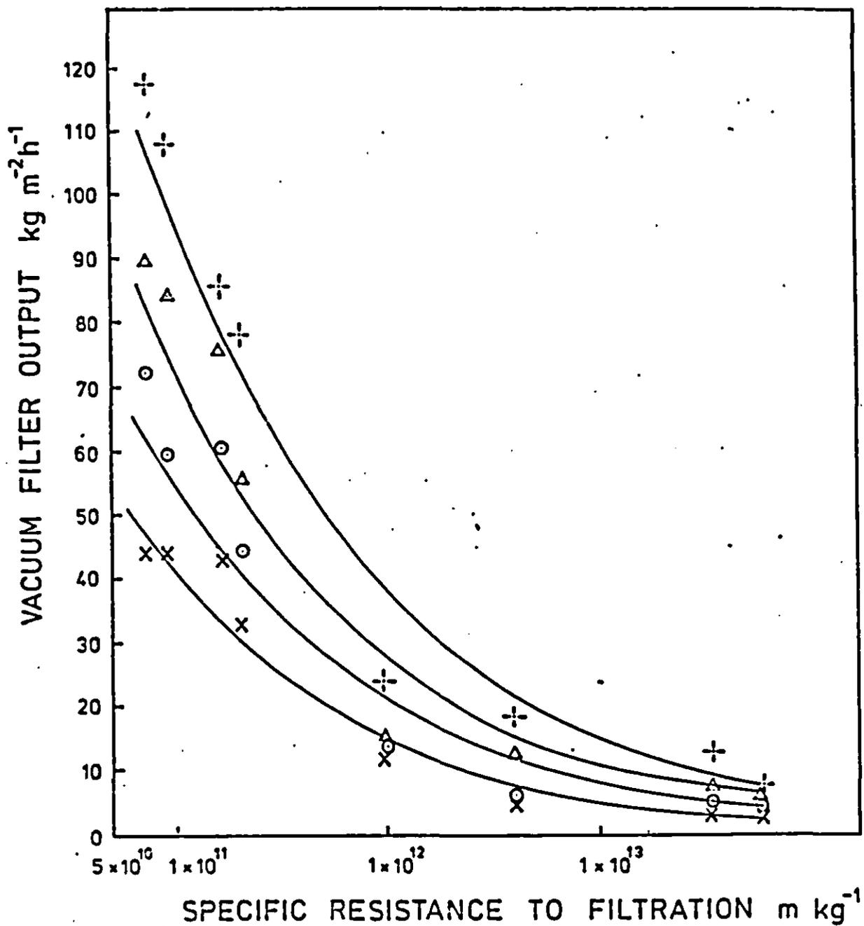
DEWATERING OF HEAT TREATED SLUDGE BY VACUUM FILTRATION.
