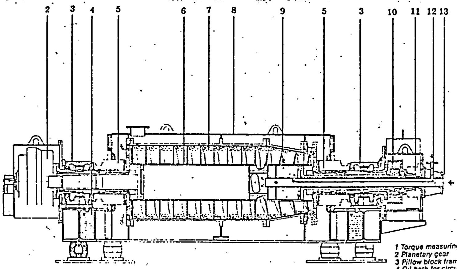
Figure 5.2: Countercurrent flow centrifuge.
