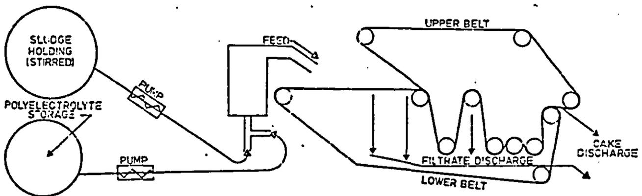
Figure 3.2 Filter belt press test equipment
