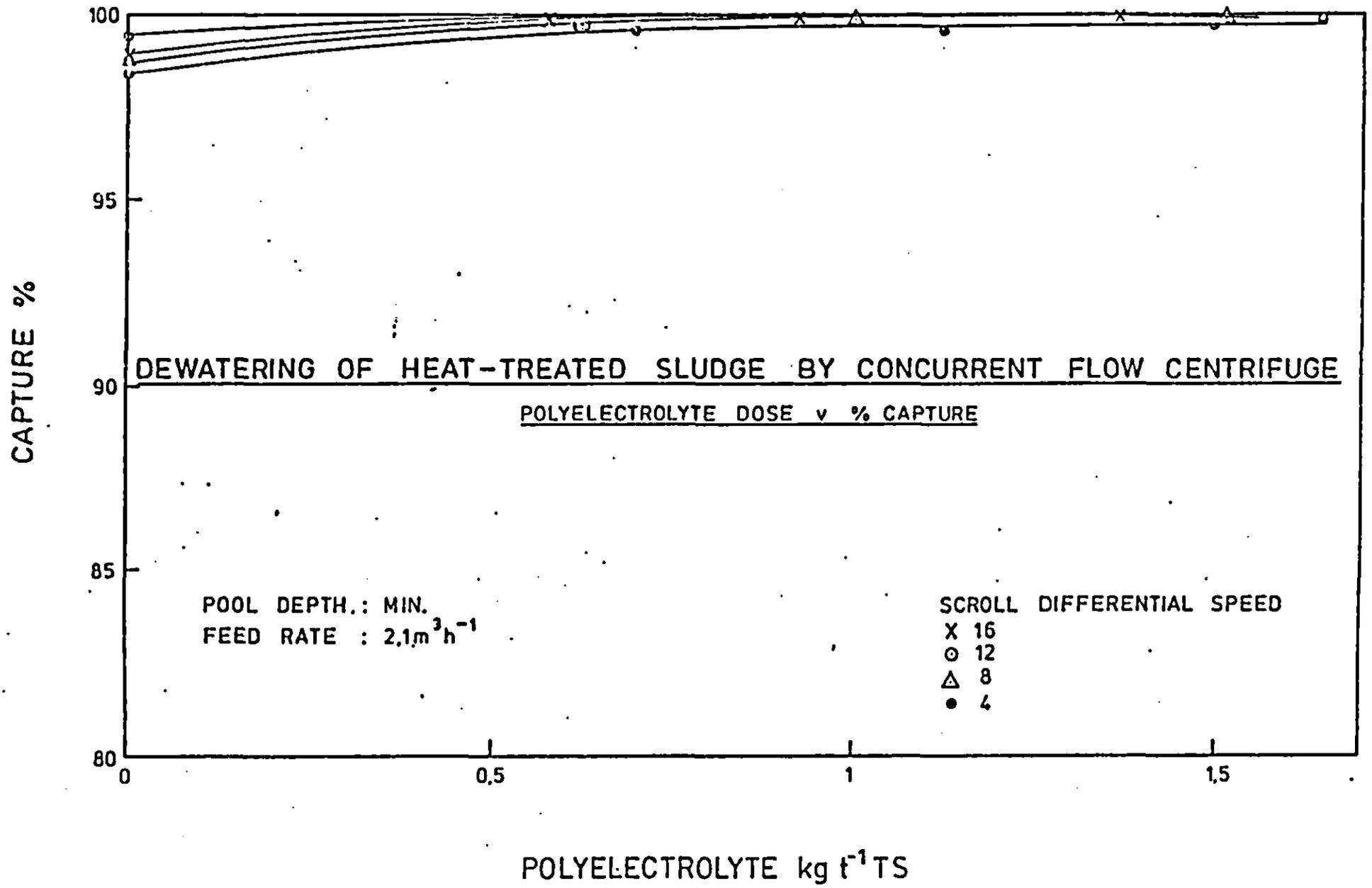
DEWATERING HEAT TREATED SLUDGE BY CONCURRENT FLOW CENTRIFUGE :
