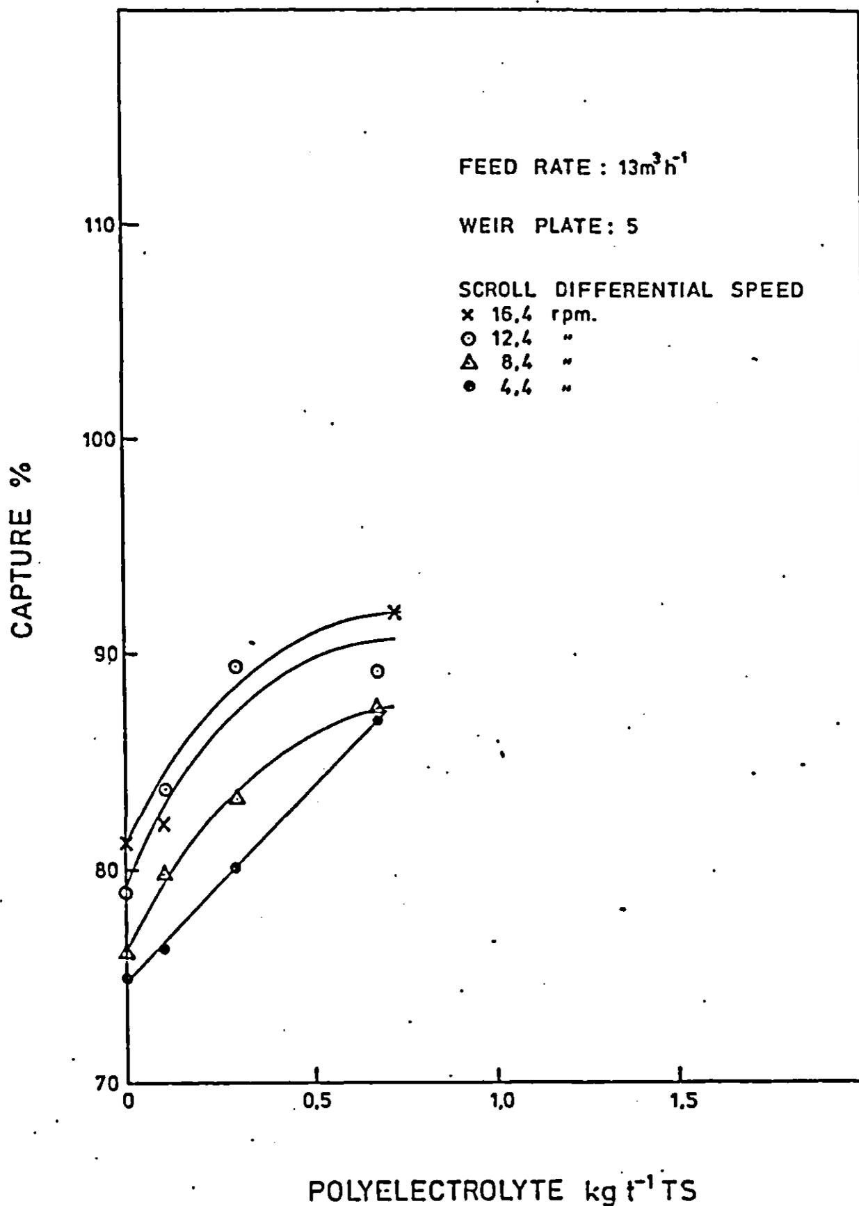
DEWATERING OF HEAT-TREATED SLUDGE:
