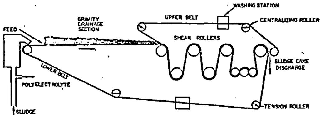
Figure 3.1 Configuration of a typical filter belt press
