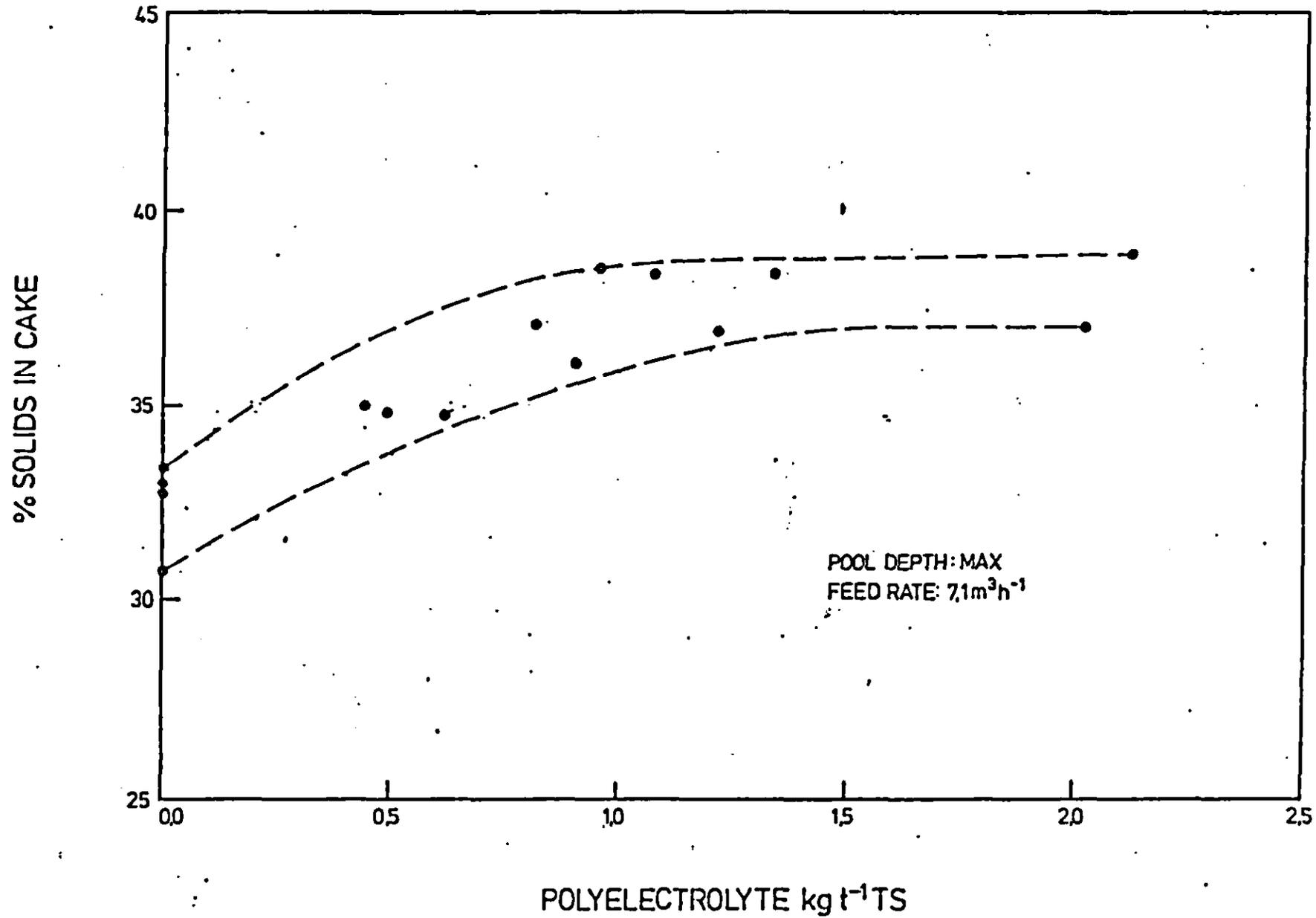
DEWATERING HEAT-TREATED SLUDGE BY CONCURRENT FLOW CENTRIFUGE.
