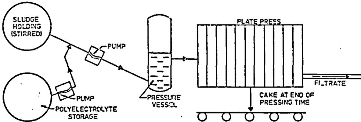
Figure 4.3 Filter plate press test equipment
