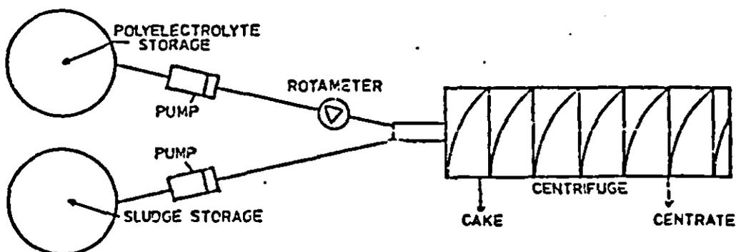
Figure 5.3 Centrifuge test equipment
