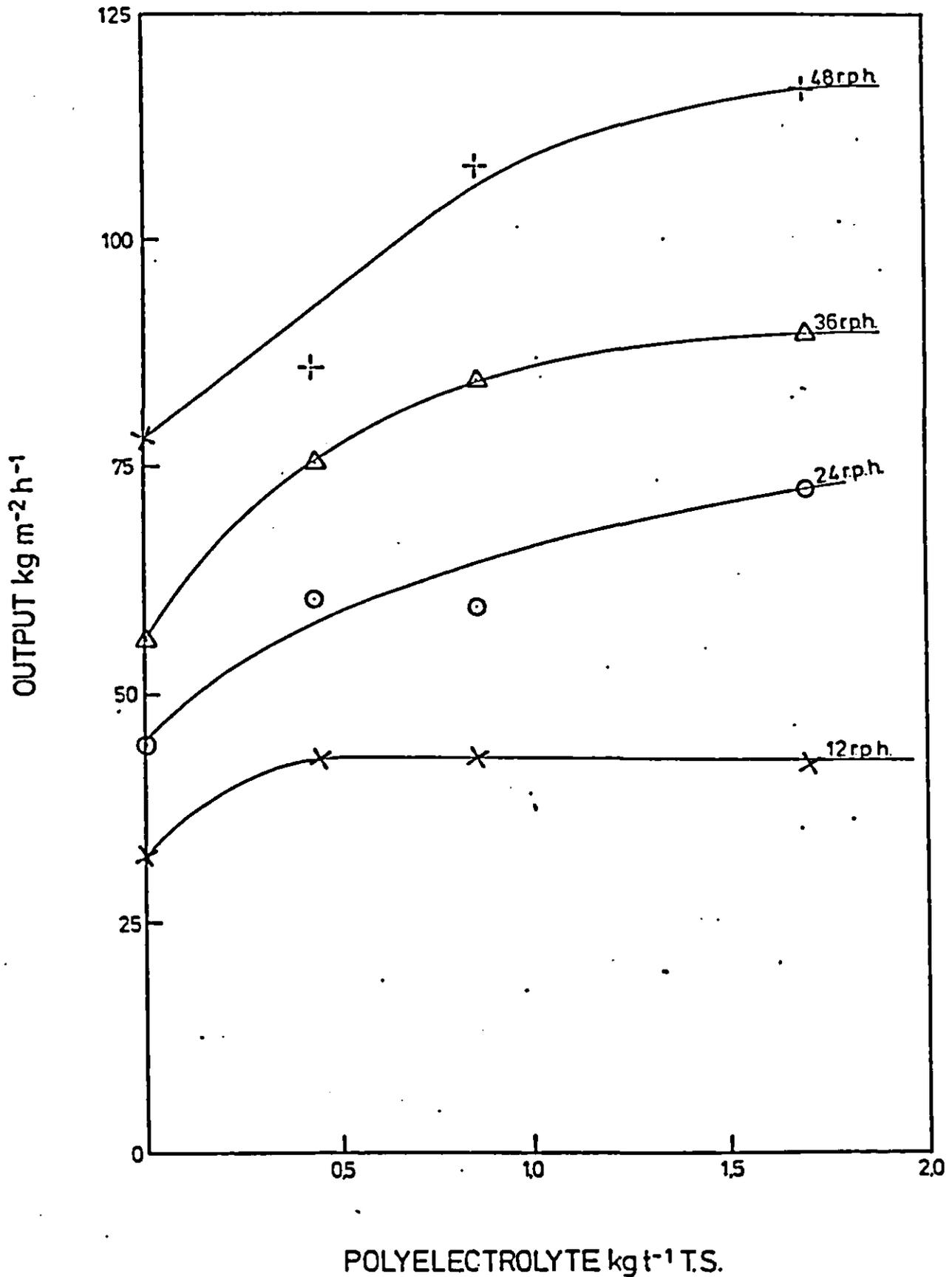
DEWATERING OF HEAT-TREATED SLUDGE BY VACUUM FILTRATION.
