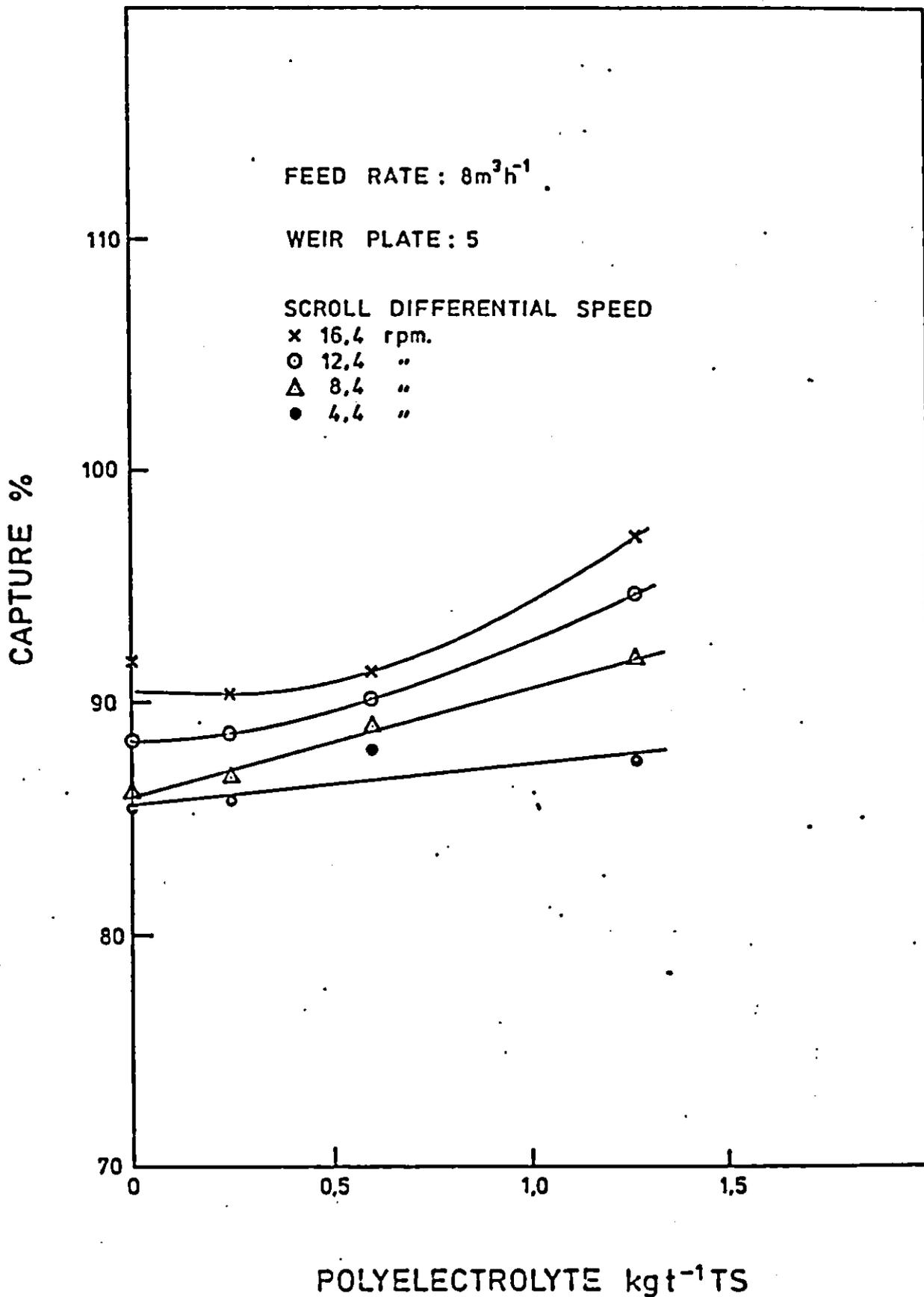
DEWATERING OF HEAT TREATED SLUDGE -
