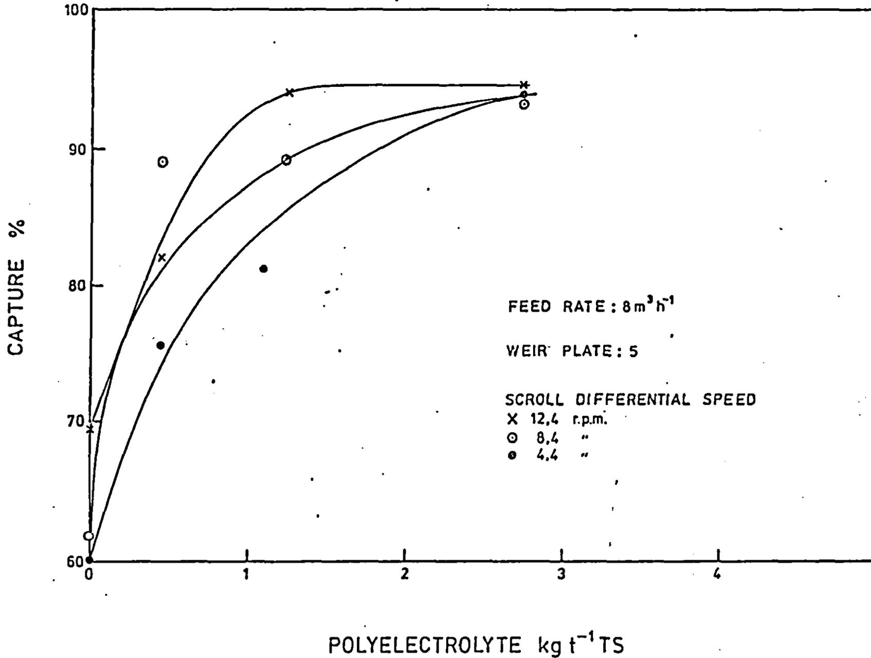
DEWATERING OF UNTREATED SLUDGE-COUNTERCURRENT CENTRIFUGE
