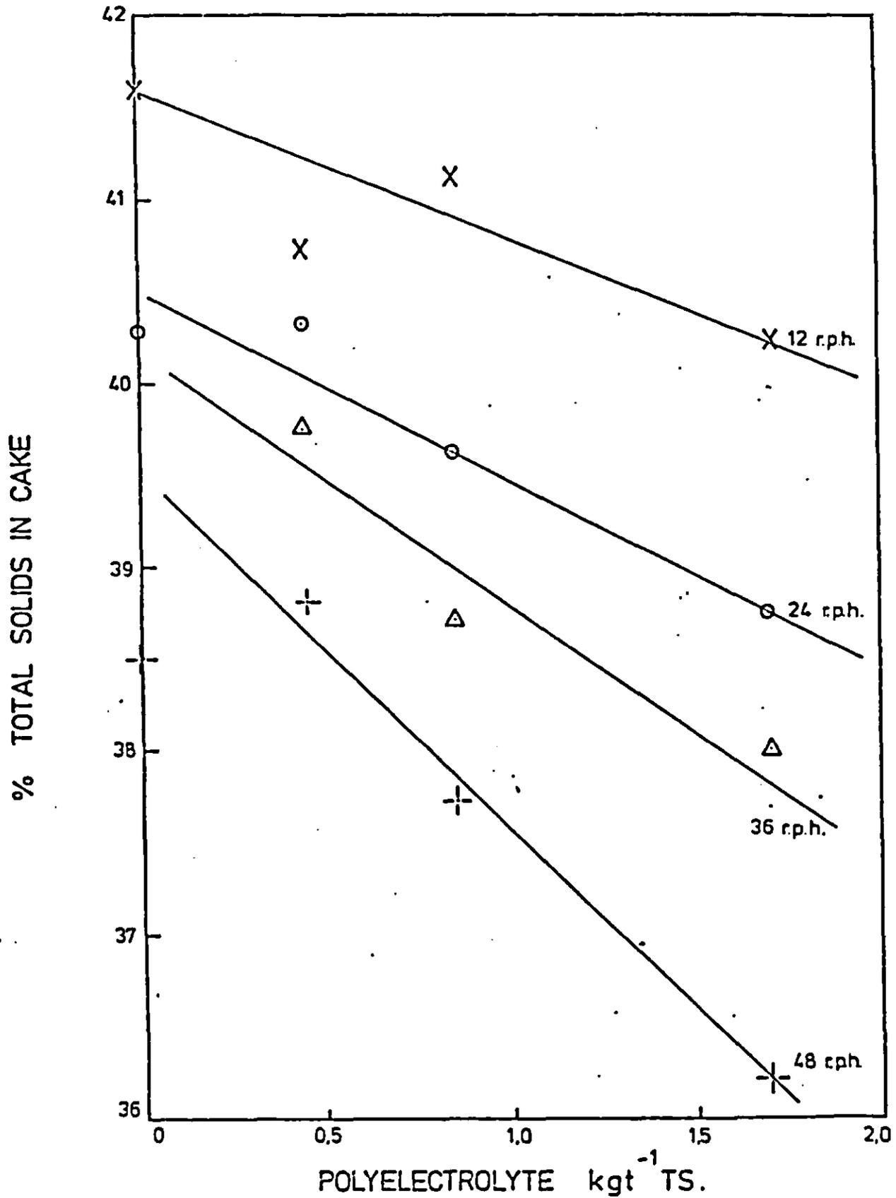
DEWATERING OF UNTREATED SLUDGE BY VACUUM FILTRATIONPOLYELECTROLYTE DOSAGE v VACUUM FILTER OUTPUT  $\text{kg m}^{-2}\text{h}^{-1}$
