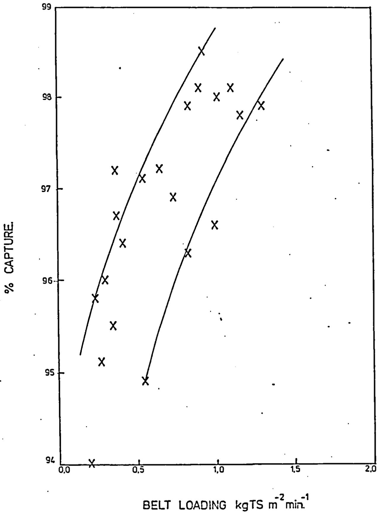
DEWATERING OF HEAT TREATED SLUDGE BY FILTER BELT PRESS
