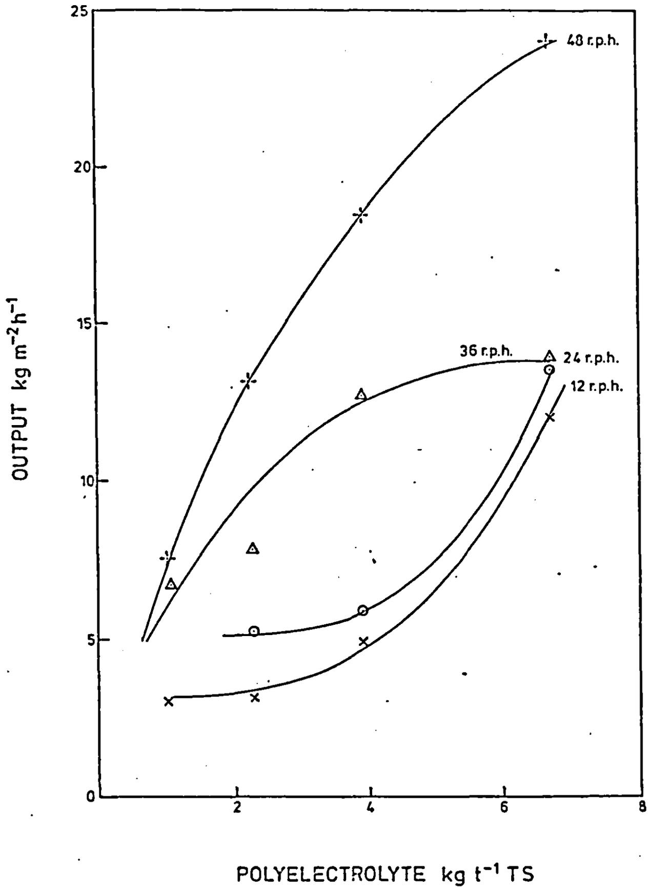
DEWATERING OF UNTREATED SLUDGE BY VACUUM FILTRATION.
