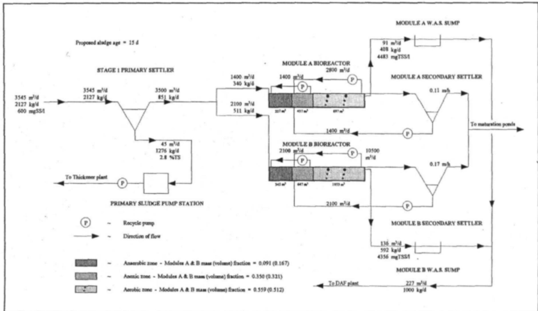
Fig 2.3: Layout of modified Mitchells Plain pilot plants as modified UCT systems.
