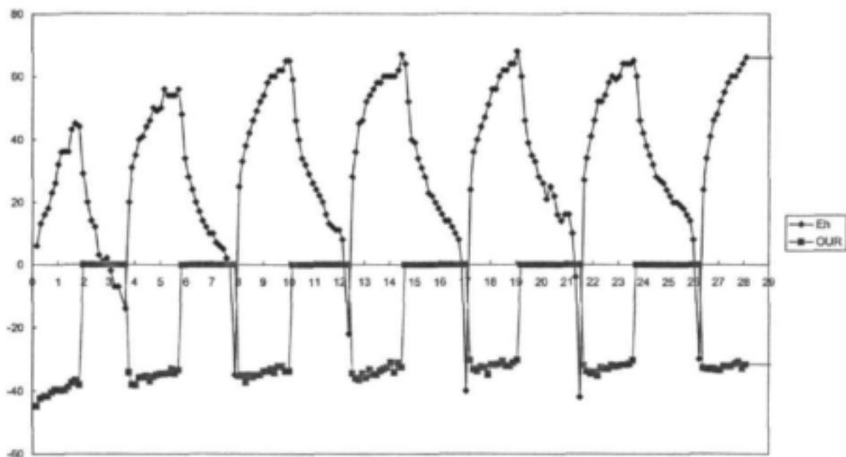
Fig 3.3: An example of daily measured redox potential and OUR (mgO/l/h) values collected by the Redox/DO controller system.
