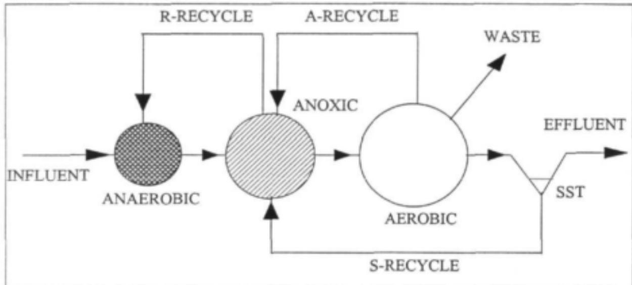
Fig 2.18 : Schematic layout of the laboratory-scale UCT system.
