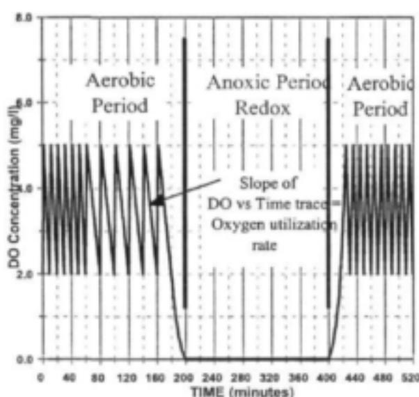
Fig 3.2: Operation of the Redox/DO controller on the ES.
