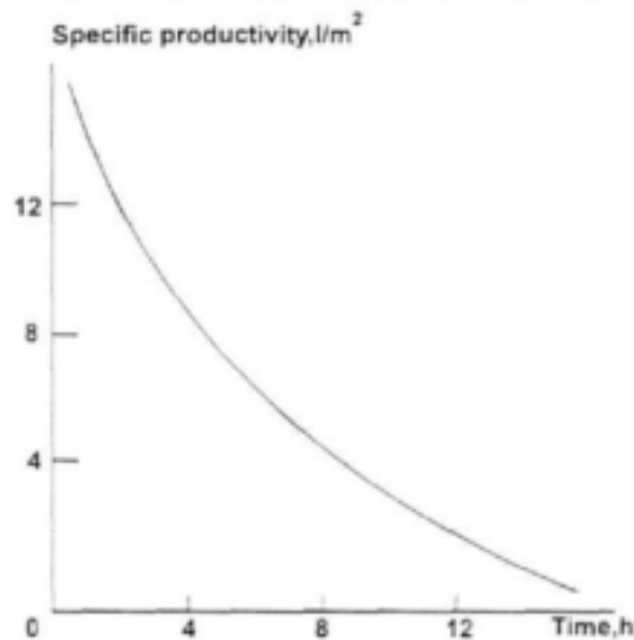
Figure 3.7: Specific productivity of cellulose acetate membranes versus operation time, during the treatment of mining effluents without any pre-treatment.
