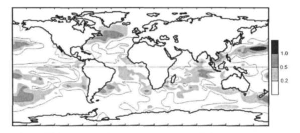
FIGURE 5.5(b) CGCM forecast Sea Surface Temperature (SST) anomalies for December 2001 measured in °C. The forecast simulation has been initialised from the beginning of August 2001. The dotted line represent the zero isotherm and the shaded areas has temperatures of 0.2 degrees and higher.
