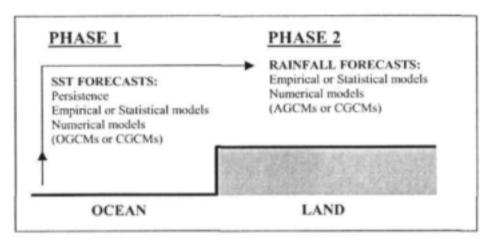
FIGURE 1.1: A typical example of the various models (or methods) used during the two phases of a two-tiered forecasting procedure. As a result of the response of the atmosphere to ocean forcing, Sea Surface Temperature (SST) forecasts are normally used to estimate future rainfall projections over land (or ocean).
