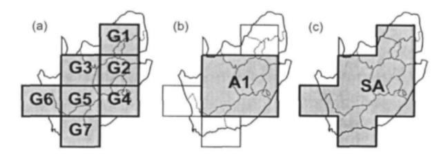
FIGURE 3.1 Spatial regions used in the forecast analyses namely (a) seven separate model grid boxes (G1 to G7), (b) a composite of four model grid boxes to form a central continental region (A1) and (c) a composite of seven model grid boxes to form one region (SA) that covers most parts of South Africa.
