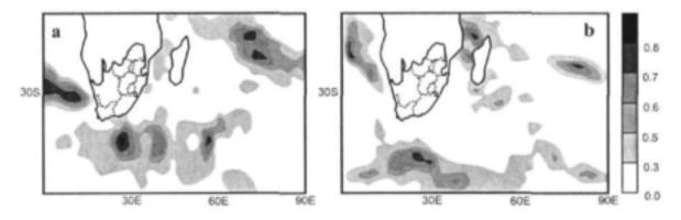
FIGURE 5.4 Regional spatial anomaly correlations between CGCM forecast SSTs with a time lag of 6 months and observations. The correlations have been calculated from 13 hindcast simulations (1987 to 1999 = 13 years) where the model was initiated at the beginning of (a) July to forecast for January and (b) January to forecast for July. The 95% and 99% significance levels are 0.54 and 0.69 respectively.
