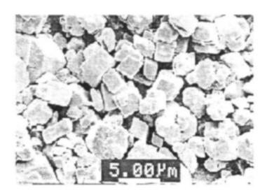
Fig. 5-8. Representative SEM images: the membrane surfaces after 30 min of operation with 2 g/l CaCO<sub>3</sub> in dead-end experiments.
