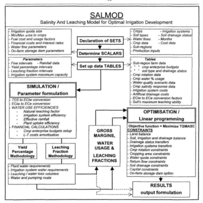
Figure 4.1 A schematic representation of SALMOD
