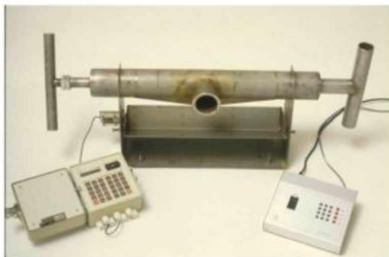
Figure 3.4 A tipping bucket flow gauge with logging equipment built locally to monitor tile drain flow (De Clercq 1992)
