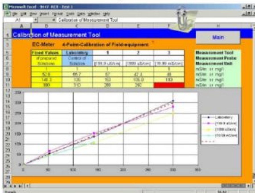
Figure 6 Input screen 'Calibration' of software TRACER
