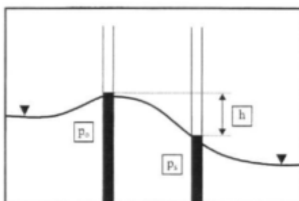
Figure 3.18: The same flow set-up as shown in figure 3.17, pressure and pressure differences in terms of manometer levels and manometer level differences
