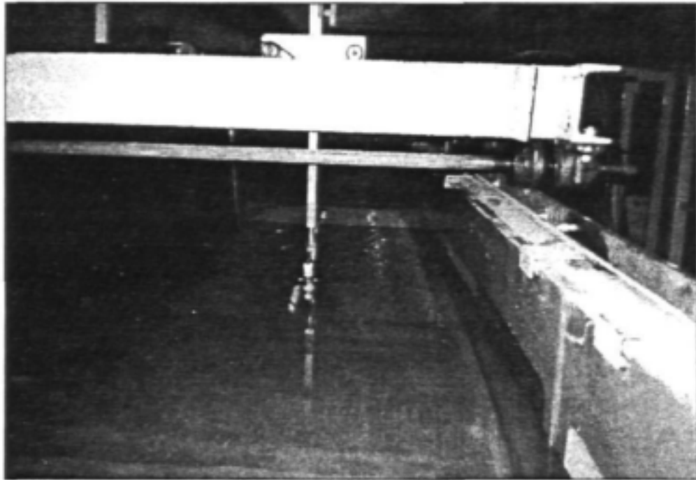
Fig 5.10: Velocity readings with the Doppler meter in approach channel of the flume in combination with Crump weirs. The Probe is directly above position 6 on this photograph.
