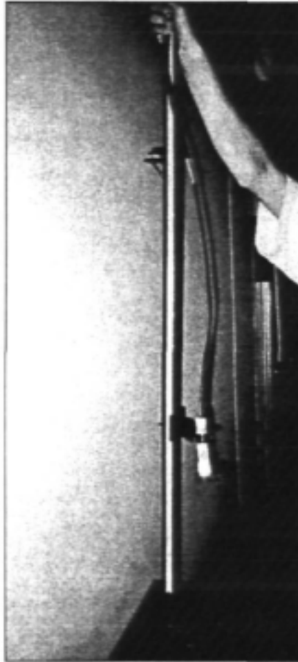
Fig 5.9: Staff with probe fixed to it. The probe shown here is nearly parallel to the canal bed.
