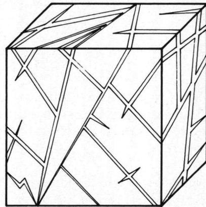
C. Joints in hard rock e.g. granite, quartzite
