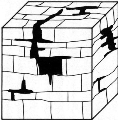
B. Caverns and solution-enlarged openings in limestone and dolomite
