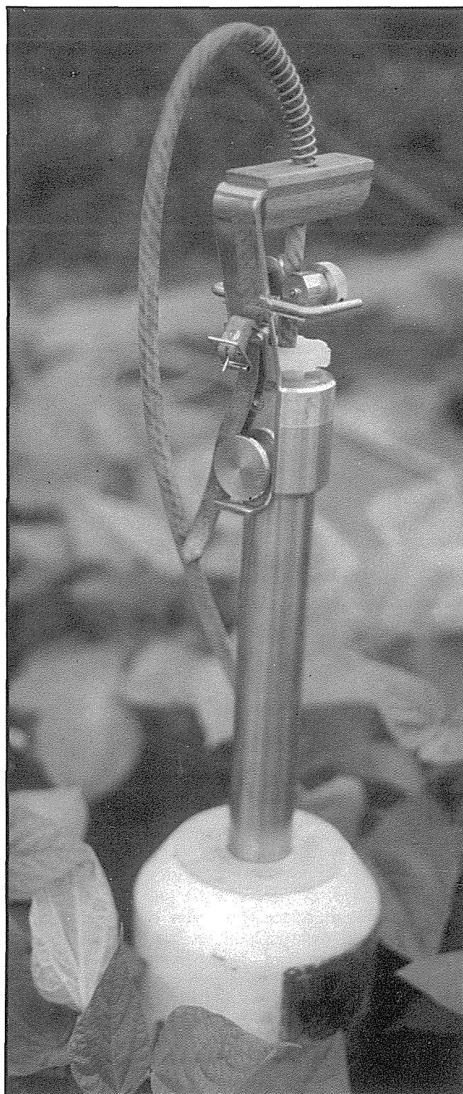
The probe of a neutron moisture meter with which soil moisture can be determined. This apparatus is used in determining the plant moisture stresses on the growth and production of certain agronomic crops.
