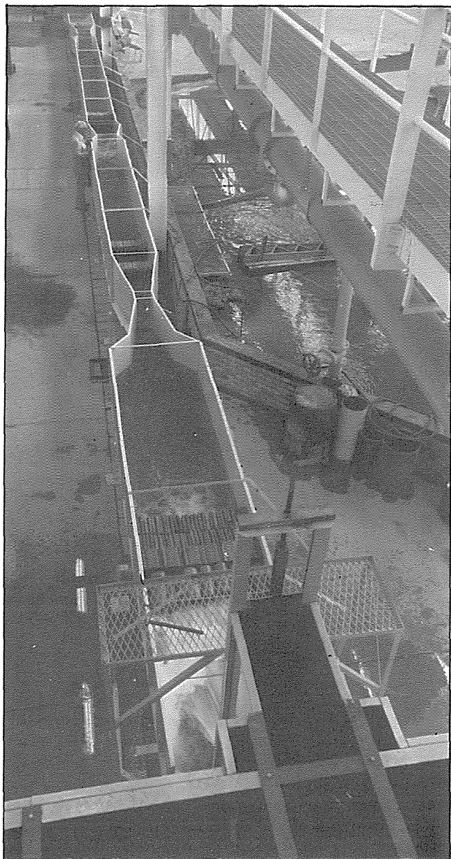
(Left) A variety of flumes in an open conduit at the Hydraulics Laboratory of the Department of Civil Engineering of the University of Stellenbosch. This equipment forms part of a project on the irrigation of steep lands.
