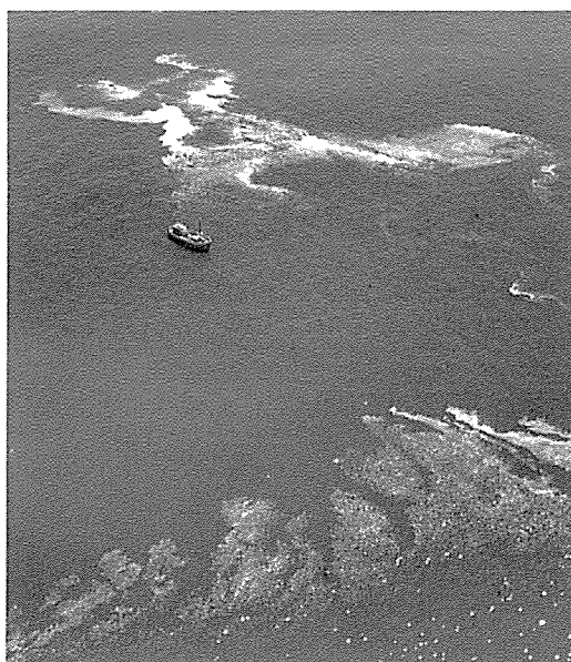
An aerial photograph of the survey vessel sampling the rhodamine coloured surfaced effluent plume from the Camps Bay sea outfall sewer (Photograph courtesy of C Best of EMA / CSIR).
