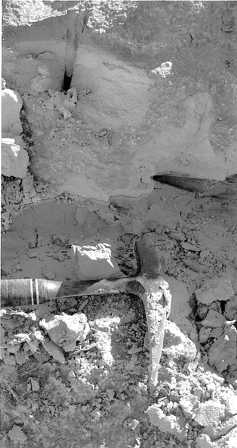
Evidence of pyrite oxidation in a shrinkage crack on a gold mine tailings impoundment.
