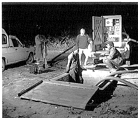
Determining the minimum night flow.
