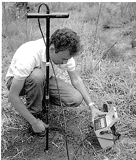
Measurement of soil salinity using the four-electrode electrical conductivity technique.
