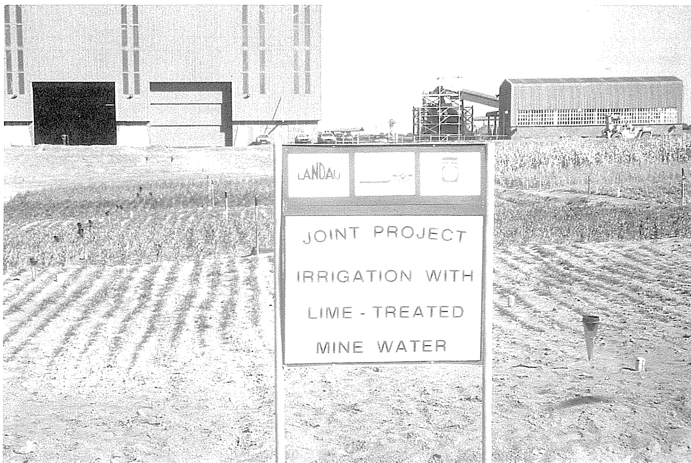
Evaluating the irrigability of various agricultural crops with neutralised acid mine water.
