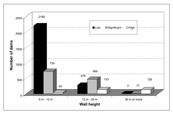
Figure 1 Classification of existing dams according to size class and hazard potential rating (31st March 2006)
