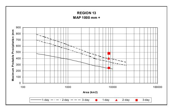
Figure 2 HRU PMP envelope curves for Region 13 (1000 mm+) with 1-day, 2-day and 3-day duration rainfall for the September 1987 storm
