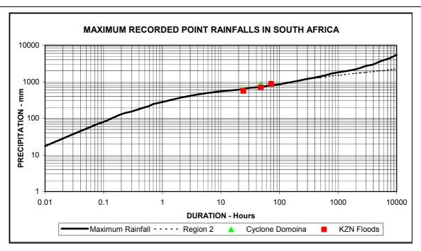
Figure 3 Maximum point rainfalls for Cyclone Domoina and KwaZulu-Natal Floods plotted against small-area storm curves for Region 2 and the Maximum Point Rainfall envelope curve
