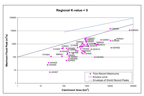
Figure 6 Maximum observed flood peaks for K-value 5
