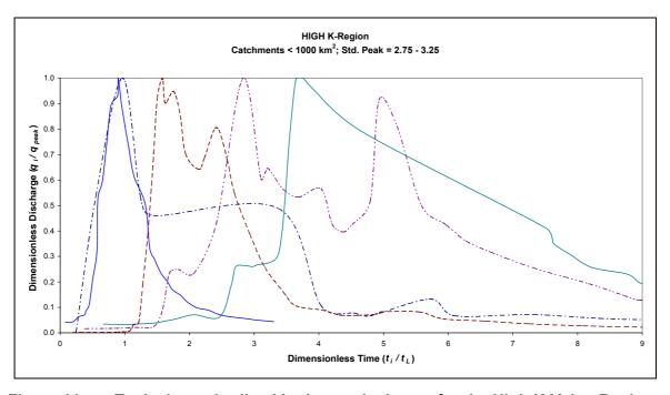
Figure 11 Typical standardised hydrograph shapes for the High K-Value Regions
