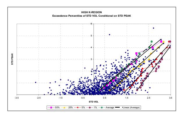
Figure 10 Relationship between standardised flood volumes and flood peaks for the high K-Value Regions
