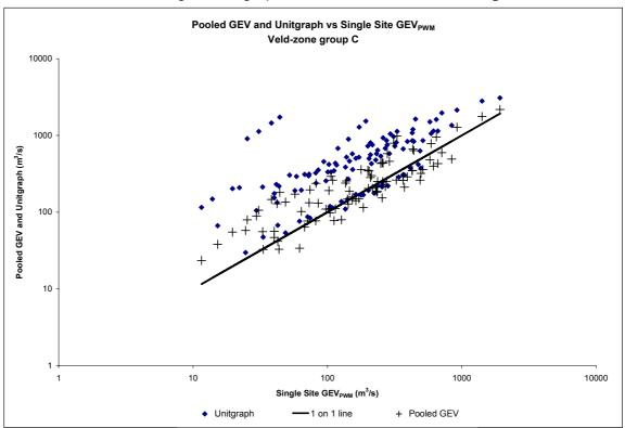
Figure 12 Comparison of design flood estimates using single site and pooled data for Veld-Zone Group C against unitgraph-based estimates
