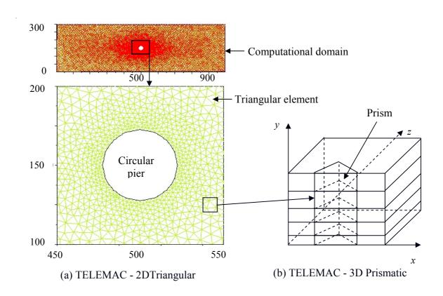
Figure 4-11: TELEMAC Two-dimensional (2D) and three-dimensional (3D) mesh
