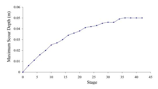
Figure 4-7: Variation of maximum scour depth with stage (FLUENT)
