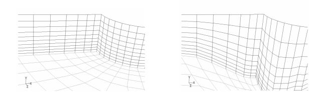
Figure 4-5: Illustration of mesh adaptation (FLUENT)
