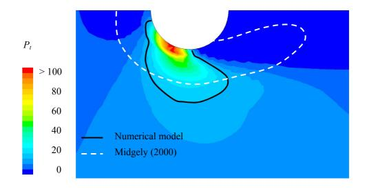
Figure 4-3: Plan view of the contours of applied unit stream power indicating the region affected by local scouring at a circular pier (FLUENT)
