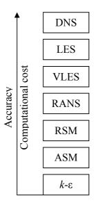
Figure 4-1: Relationship between computational cost and accuracy of turbulence models
