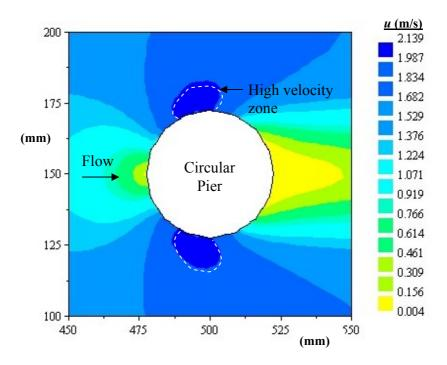
Figure 4-12: Scalar x-velocity contours around circular pier (TELEMAC-2D)
