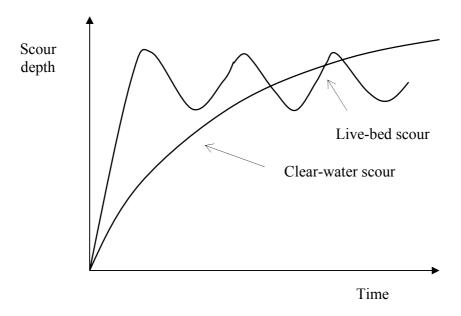
Figure 2-1: Scour depth as a function of time (After Armitage and McGahey, 2003)
