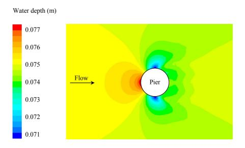
Figure 4-2: Plan view of the variation of the free surface around a circular pier (FLUENT)
