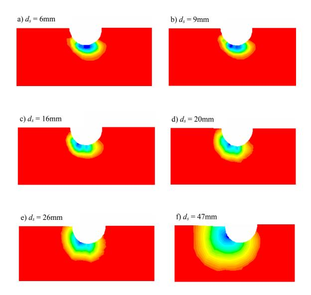
Figure 4-6: Stages in scour hole development (FLUENT)
