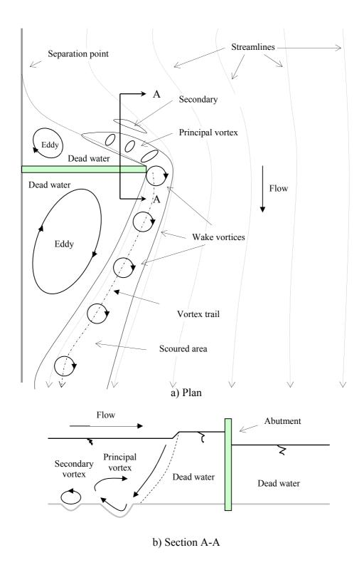
Figure 2-3: Flow patterns around an abutment (After Breusers & Raudkivi, 1991; Hoffmans & Verheij, 1997; Raudkivi 1998)
