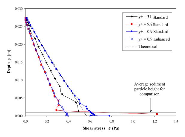
Figure 4-4: Distribution of shear stress with depth for different wall models
