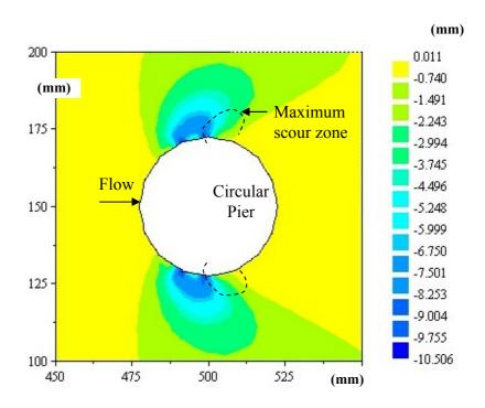
Figure 4-13: Scoured bottom topography around circular pier (TELEMAC-2D)
