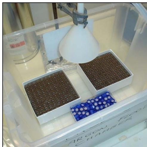
Picture 11. Samples being flooded with argon.
