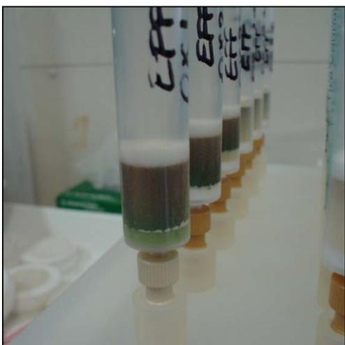
Picture 9. SPE cartridges after sample extraction.
