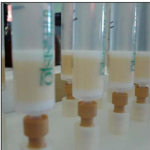
Picture 8. Pre-conditioned Waters Oasis HLB cartridges.
