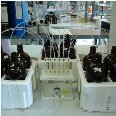
Picture 7. Samples are passed by vacuum through solid-phase extraction cartridges.
