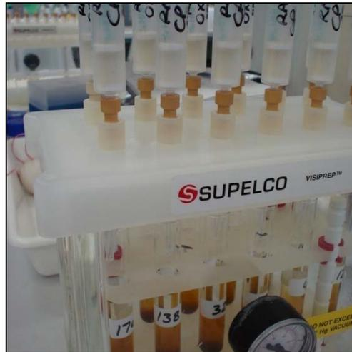
Picture 10. Eluted SPE cartridges. Note extracted sample in tube underneath.
